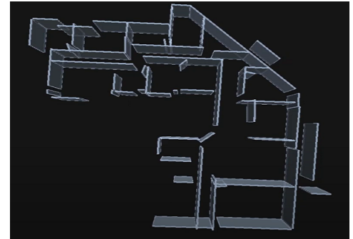
Figure 2: Automatic wall extraction in "EdgeWise". The set of detected walls is incomplete and contains wrong cuboids. Besides, the accuracy of wall dimensions is not perfect and a human needs to adjust wall length manually.
