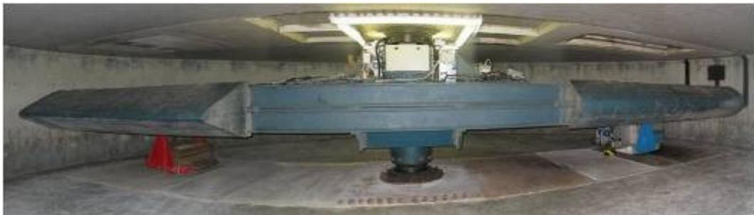
**Figure 4.2** Turner beam centrifuge, where all tests were conducted. Photograph from SERIES (2011)
