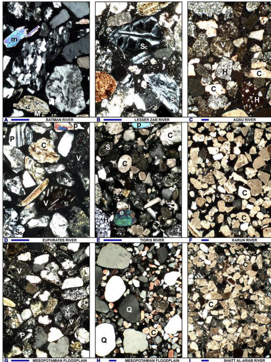
Figure 2.15: Petrography of Various Areas of Iraq “A) Metamorphiclastic detritus from the Bitlis massif (M = metamorphic lithic; m = mica). B) Cellular serpentinite (Sc) and foliated serpentinite/schist (Ss) grains from ophiolites of the Zagros suture. C) Volcanic (V) chert (H) and carbonate (C) grains recycled entirely from Neogene molasse units of the foothills. Trunk-river systems: D) Euphrates sand rich in volcanic detritus including plagioclase (P) and clinopyroxene (p). (E) Tigris sand rich in sedimentary detritus (S = shale lithic; e = epidote). F) Carbonaticlastic Karun sand. Foreland-basin fill: G) Mesopotamian sediments derived from Euphrates and Tigris Rivers in subequal proportions. H) Rounded quartz grains (Q) recycled from Arabian sources mixed with finer-grained quartz-poor orogenic detritus in the Karbala area (calcareous grains stained with alizarine red). I) Carbonaticlastic Shatt al-Arab sand supplied entirely by the Karun River because Euphrates and Tigris bedload is trapped in Iraqi marshlands before reaching the Gulf. All photos with crossed polars; all blue bars for scale are 250 \mu\text{m} ” (Garzanti et al 2016: Fig. 3).
