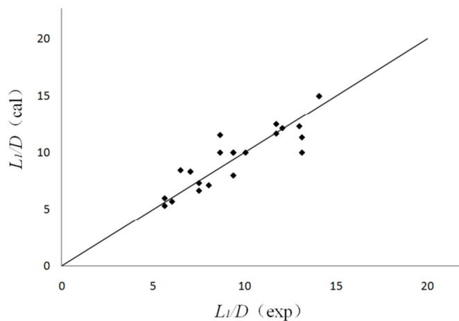
Fig.9 Comparison of the experimental and calculated  $L_1 / D$  for discharges of less than bankfull discharge
