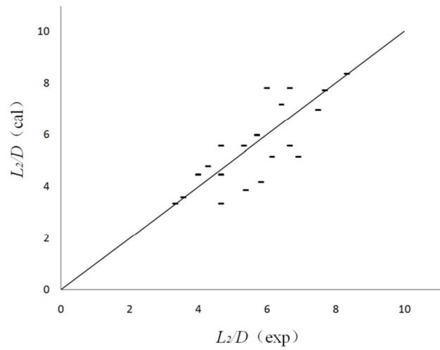
Fig.10 Comparison of the experimental and calculated  $L_2 / D$  for discharges of less than bankfull discharge
