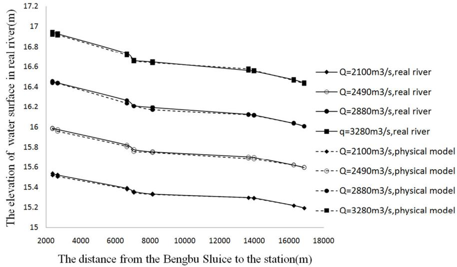
Fig.2. Comparison of the water surface elevation between the real river and the physical model
