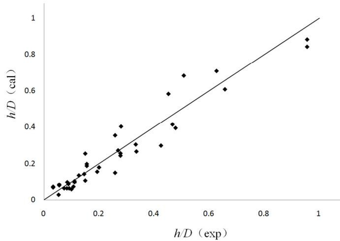
Fig.8 Comparison of the experimental and calculated increased depth for discharges that exceed bankfull discharge
