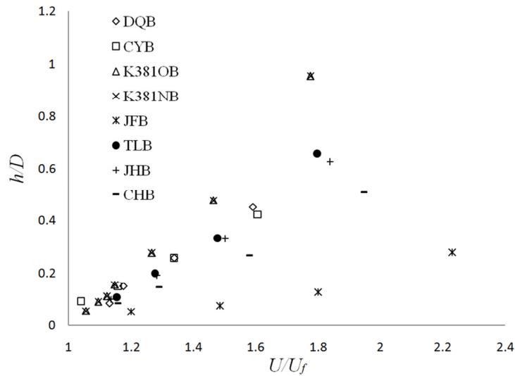
Fig.7. Increased depth for discharges that exceed bankfull discharge
