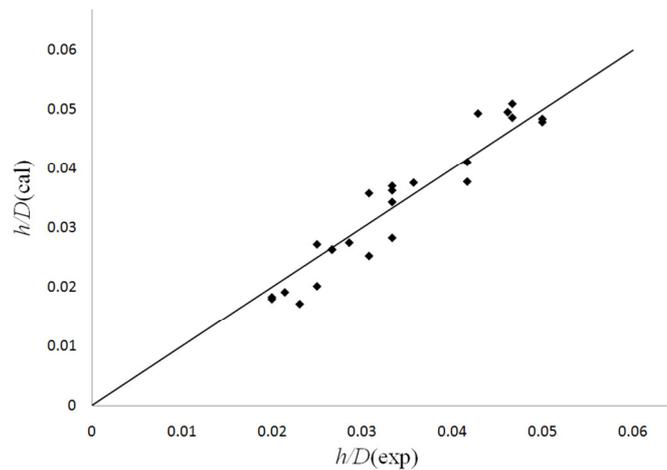
Fig.6 Comparison of the experimental and calculated increased depth for discharges of less than bankfull discharge
