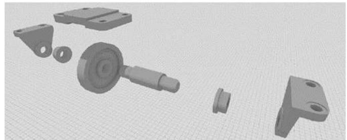
**Fig. 8: The exploded view of a caster wheel.**
