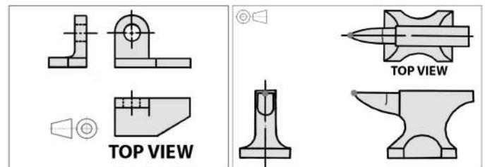
**Fig. 5: First angle projection of a bracket (left) third angle projection of an anvil (right)**
