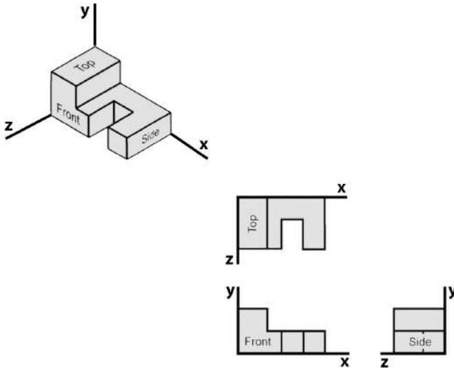
**Fig. 1: Three-dimensional object represented in a single view drawing (top left) and multi-view drawing (bottom right).**
