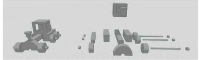
**Fig. 7: An example of a toy truck in the assembled view (left) and in the exploded view (right).**
