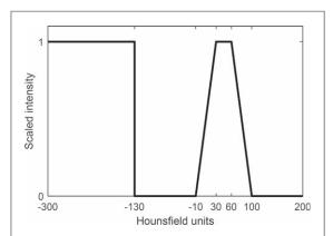
Figure 2. Rescaling from Hounsfield Units (HU) to scaled intensity. Pixels less than  $-130\,$  HU are identified as rectal gas and are rescaled to an intensity value of 1 to be included as rectal content. Pixels between  $-10\,$  HU and  $100\,$  HU are in the 'critical range' identified as rectal contents, and are rescaled to intensity values between 0 and 1.
