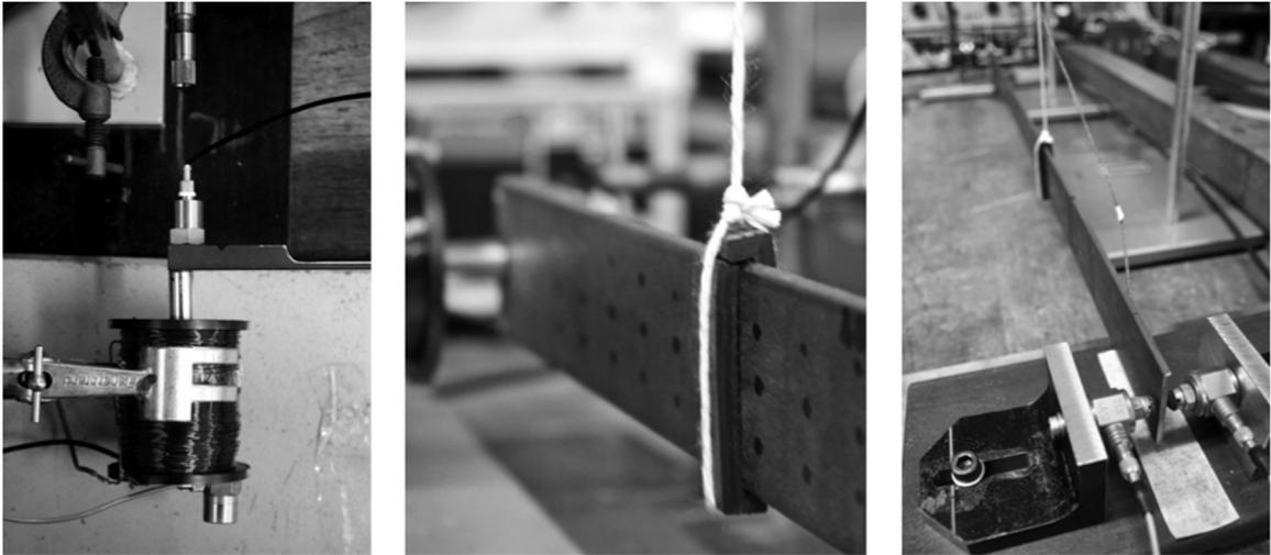
**Fig. 3.** Photographs of the experimental ‘free-free’ beam with a locally nonlinear end-stop: (left) magnet and coil providing the input force with no contact between the coil and magnet; (middle) isolated suspension to reduce boundary condition nonlinearity; and (right) end-stop nonlinearity.
