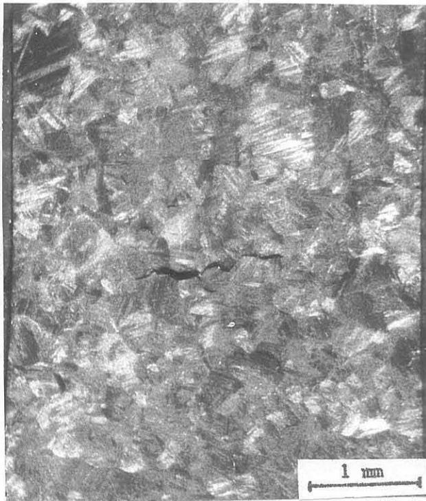
Figure 97. Cavitation in  $\frac{1}{2}\text{Cr}$   $\frac{1}{2}\text{Mo}$   $\frac{1}{4}\text{V}$  H.P. Steel having a prior austenite grain size of approximately  $170\ \mu\text{m}$  and deformed at  $500^\circ\text{C}$ .
