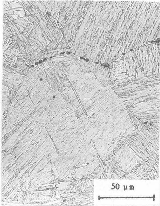
Figure 54. Cavitation in specimen #3
