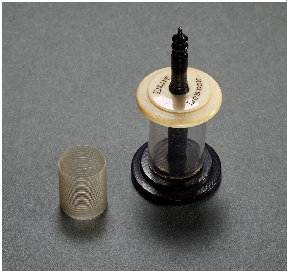
Figure 2(b). Glass balance-spring on ebony stand, dated: 1835-40, displayed but not used in a mechanism, British Museum No. 1958,1006.3009. The Trustees of the British Museum, (CC BY-NC-SA 4.0).
