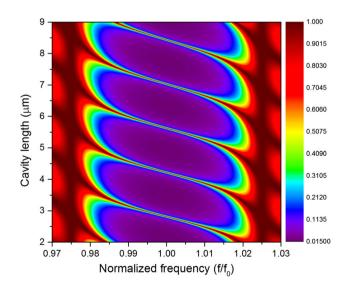
**Fig. 7** Contour plot of the transmission coefficient of a single cavity resonator for different cavity lengths and normalized drive frequencies ( $f_0 = 3$  GHz) with 50 ABR reflectors ( $L_{b1} = L_{b2} = \lambda/4$  at 3 GHz)
