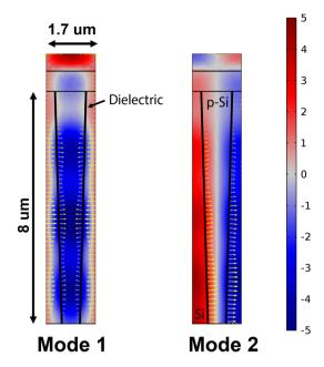
**Fig. 4** Simulated principal longitudinal mode shapes assuming a Floquet periodic ABR structure. The contour map represents the longitudinal strain distribution and the arrows represent the local material displacement
