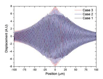
Fig. 10 Simulated vibratory mode shape for the single cavity a five cavity resonator with different perturbations
