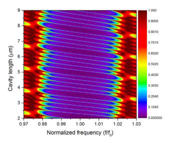
**Fig. 8** Contour plot of the transmission coefficient of a five coupled cavities resonator for different cavity lengths and normalized drive frequencies ( $f_0 = 3$  GHz) with 50 ABR reflectors ( $L_{b1} = L_{b2} = \lambda/4$  at 3 GHz), ABCG ( $N_2$ ) = ABGC( $N_1$ ) = 3 ( $L_{b1} = L_{b2} = \lambda/4$  at 3 GHz)
