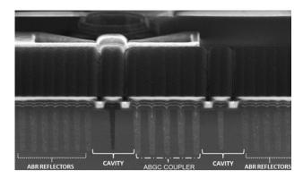
Fig. 6 SEM of a micro-fabricated mechanically coupled unreleased acoustic cavities resonator
