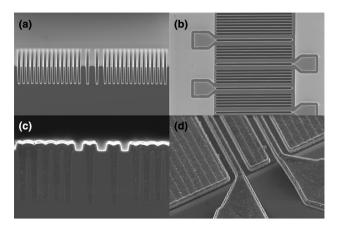
Fig. 13 SEM images of representative devices showing:  $\bf{a}$  etch of the deep trenches in the Si bulk,  $\bf{b}$  PSG deposition and drive-in for the low-resistivity channel,  $\bf{c}$  dielectric Si<sub>3</sub>N<sub>4</sub> deposition, poly-Si trench fill and d) field-oxide and metal deposition for the electrical routing
