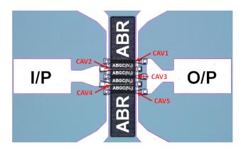
**Fig. 14** Optical micrograph of a five coupled cavities design in the  $\langle 110 \rangle$  direction, with the ABR, ABGC( $N_1$ ), ABGC( $N_2$ ) and CAV regions labeled
