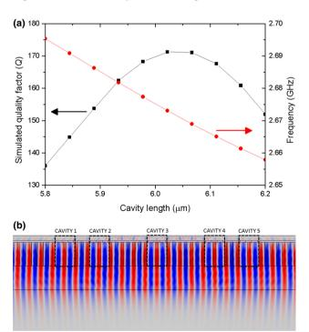
Fig. 12 a Simulated quality factor Q and resonant frequency, for different cavity lengths. b Simulated strain field for the largest Q case when  $L_{\rm cav}=6.02~\mu{\rm m}$  for a five coupled cavities resonator
