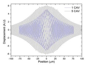
**Fig. 9** Simulated vibratory mode shape for the single cavity (1 CAV blue curve) and five cavity (5 CAV black curve) resonators (colour figure online)
