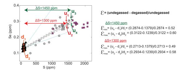
Figure A13: The upper and lower bounds of the 95% confidence interval on the regression of a given element against S were used to estimate an upper and lower bound on the emanation coefficient for each  $\Delta S$  value.
