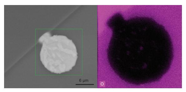
Figure A9: Map of O in a sulfide which does not show textural evidence for resorption. The sulfide is very O-poor (compare to Fig. A8, Fig. 6).
