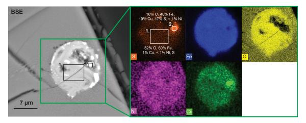
Figure A8: A broken down sulfide within degassed matrix glass. Area 1 is almost entirely composed of iron oxides, while area 2 is still relatively sulfur and copper-rich (although it also contains significant amounts of O, unlike pristine sulfides; see Fig. A9).
