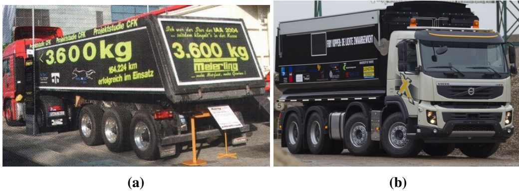
Fig. 1.7 (a) Carbon fibre monocoque tipper trailer developed by TTT Composite AG in collaboration with fellow German company Meierling [4]. (b) Thermoplastic based Fiby tipper developed by a collection of Dutch companies for ComposiTTTransport [10].
