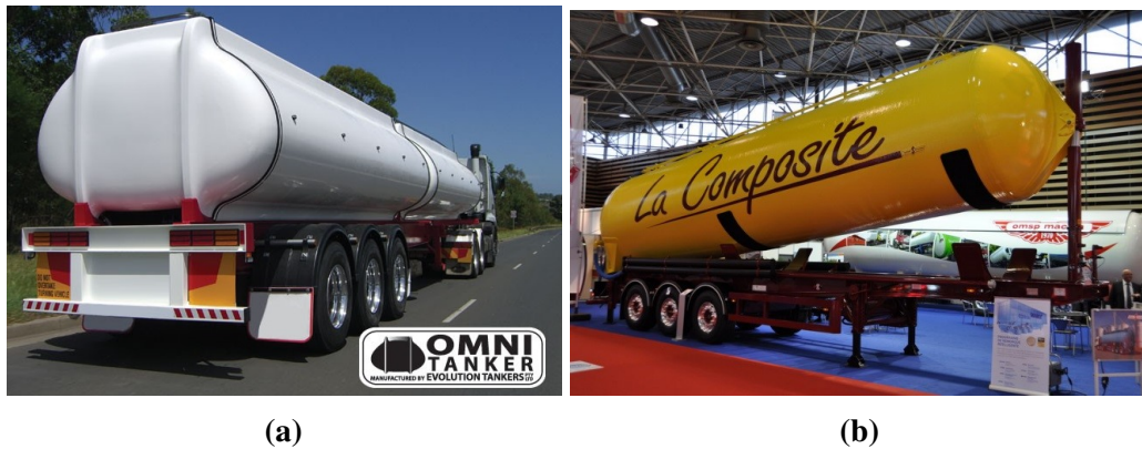
Fig. 1.6 (a) The carbon fibre based Omni Tanker developed by Australian company Evolution Tankers Pty Ltd. [8]. (b) Tippable composite cylindrical tanker made by French company Spitzer-Eurovac [9].
