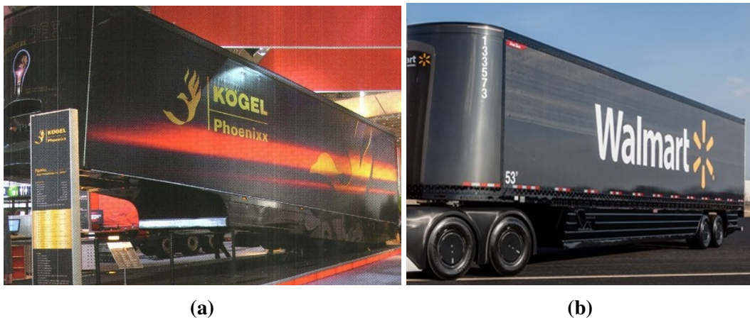
Fig. 1.4 (a) The 13.6 m carbon fibre based Phoenixx trailer developed by TTT Composite AG for German trailer manufacturer Kögel [4]. (b) The carbon fibre based Walmart concept trailer developed by American trailer manufacturer Great Dane Trailers project [5].
