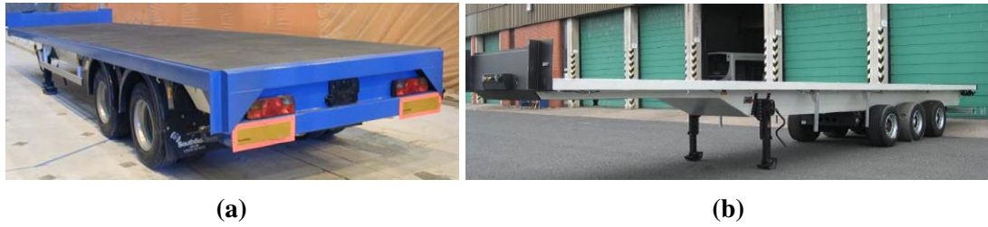
Fig. 1.3 (a) The 10 m ROADLITE trailer developed by Nottingham University and EPL composites [2]. (b) The 13.6 m CleanMould trailer developed by EPL composites and other collaborators continued on the work from the ROADLITE trailer project [3].
