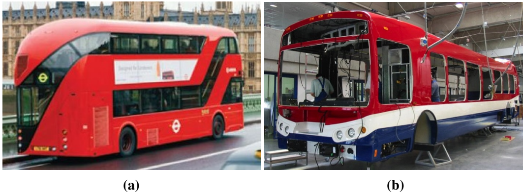
Fig. 1.11 (a) The new London Wrightbus incorporates a large structural GFRP section at the rear developed by Gurit [14]. (b) The CompoBus used in Los Angeles boasts a wholly composite design [15].
