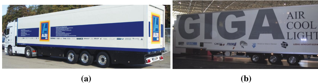
Fig. 1.5 (a) The 13.6m carbon fibre based refrigerated trailer developed by TTT Composite AG for German retailer Aldi [6]. (b) The 13.6m refrigerated GIGA trailer which uses a carbon fibre monocoque structure developed by Dutch company Talson Transport Engineering [7].
