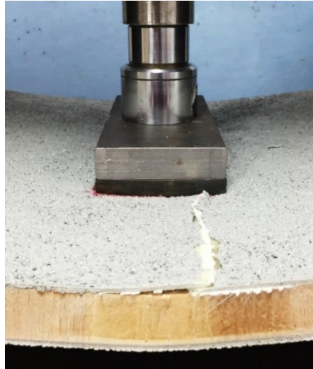
Fig. 4.19 Top face sheet failure observed during large panel testing of 30 mm thick woven GFRP-balsa (SB.150) single shot sandwich panel with non-slip coating. Failure propagates along one edge of the rubber pad that simulates a forklift wheel.
