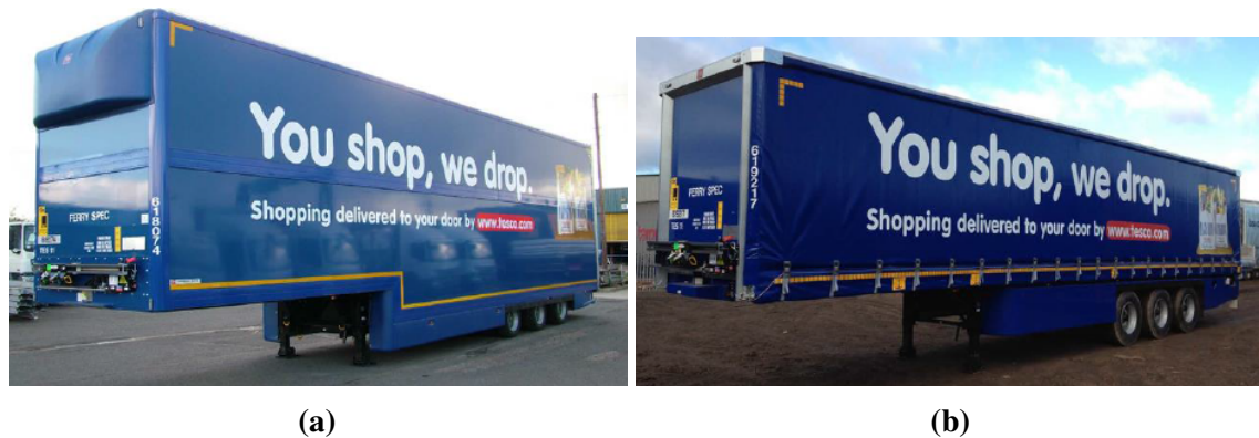
Fig. 2.3 (a) A three axle 13.6 m double-deck trailer with box side-walls. (b) A three axle 13.6 m single deck curtain side trailer.
