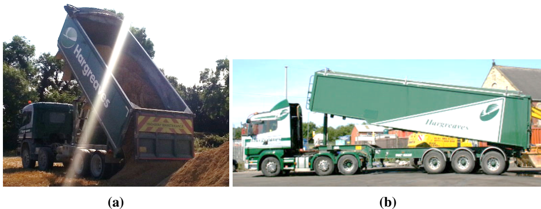
Fig. 2.7 (a) Rigid '8 wheeler tipper' used in bulk haulage. (b) Steel tipping bin articulated combination with a total of six axles used in bulk haulage.
