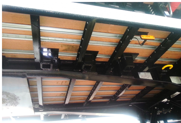
Fig. 2.13 Hardwood flooring laid over steel chassis beams (view from underside of a 13.6 m flat-bed trailer at the goose-neck).
