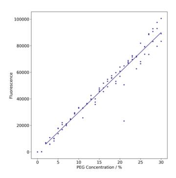
**Figure 2.** The robot pipetting is accurate despite the high viscosity of PEG-containing solutions. The automated PEG assay was carried out by titrating a PEG stock containing free AlexaFluor488 fluorophore. We validated the accuracy of the robot in transferring solutions by assessing the linear relationship between the AlexaFluor488 fluorescence (y-axis) and the expected PEG concentration (x-axis). The median error which represents the shift from the expected PEG concentration is about 0.8%.
