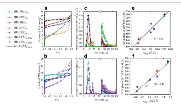
Fig. 4 N<sub>2</sub> isotherms (77 K) and pore size distributions for MIL-53(AI) materials with adjusted modulator stoichiometry/concentration (a and c) and varied reaction time (b and d); linear fits obtained by plotting (e) the BET surface areas (S<sub>BET</sub>) and (f) micro pore volume (V<sub>micro</sub>) of all 8 samples against their respective TGA plateau at 250 °C.
