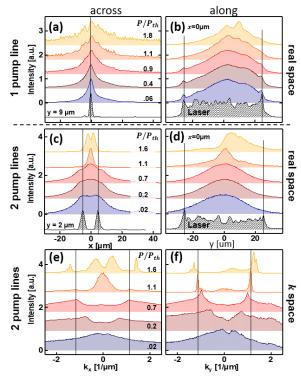
FIG. 2. (a-d) Real-space cuts of the polariton distributions (a) across and (b) along a single pump line, (c) across and (d) along two pump lines, for increasing pump powers. Grey lines show measured excitation profiles (speckle contributes noise). (e,f) Corresponding cuts along  $k_x$  and  $k_y$  for two pump lines.
