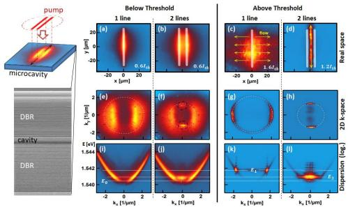
FIG. 1. (a-d) Real-space images of polariton emission when pumped with single or pairs of lines (as indicated in left schematic), both below and above the condensation threshold. (e-h) Corresponding momentum-space images of the entire polariton emission, white circles mark eventual condensation wavevector. (i-l) Cuts of the E(k) dispersion across the centre of the dashed circles marked in (e-h).
