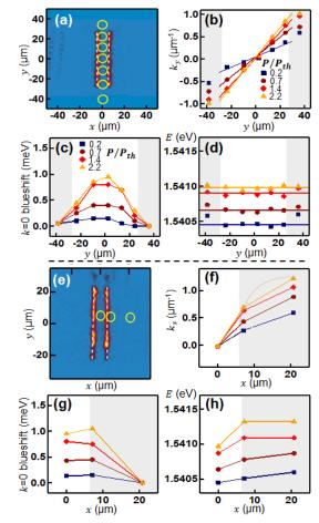
FIG. 3. Spatially- and energy-resolved polariton emission using two pump lines, scanned along (a-d) y- and (e-h) xdirections. (a,e) Images of pump laser, yellow circles mark pinhole positions. (b-d) Polariton momentum, local blueshift energy and absolute energy for positions in (a) along y, (f-h) equivalent along x. Regions outside the polariton waveguide are shaded grey.
