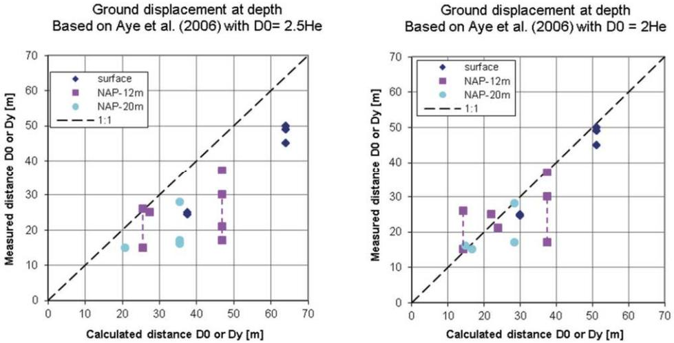
Figure 5.17 Comparison between measured and calculated influence distance a) for  $D_0=2.5H_e$  and b) for  $D_0=2H_e$
