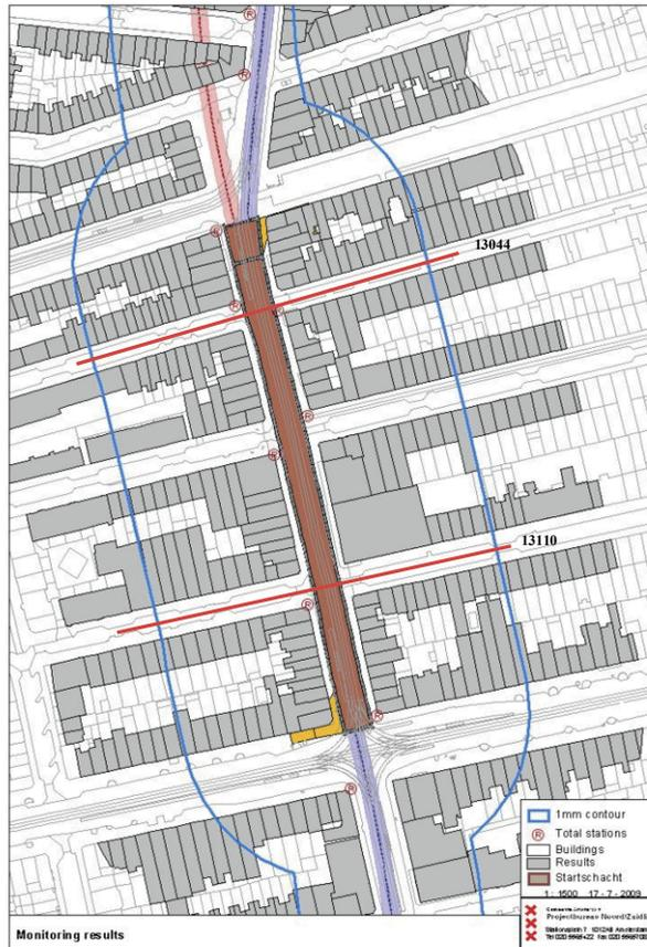
Figure 4.24 Locations of cross sections with subsurface monitoring
