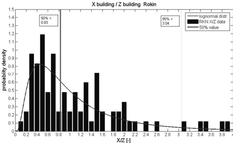
Figure 9.12 Histogram plots for probability of X/Z values for Rokin station with X/Zbuilding
