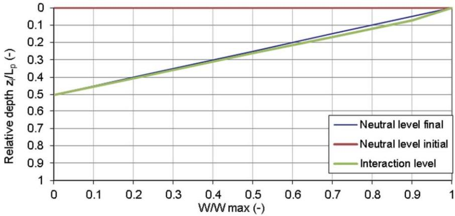
Figure 7.13 Changes of depth of neutral level with initial load increasing from  $W/W_{max}$  is 0 to 1 for  $\Delta S/D_z = 50$ .
