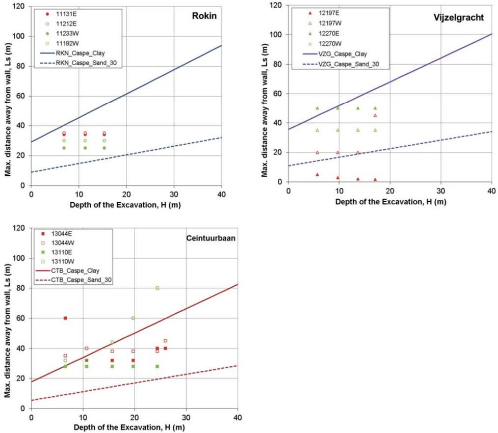
Figure 5.11 Maximum distance away from the wall to which the displacement is found compared to Caspe's prediction model for the excavation stages for each of the three stations
