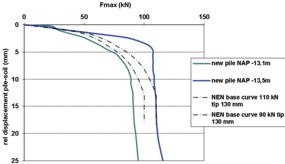
Figure 6.6 Base load displacement curve for new piles
