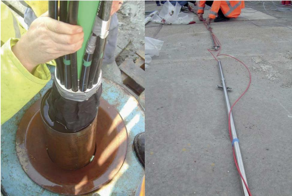
Figure 4.37 Combined inclino- and extensometer (a) and assembled inclinometer instrument (b)
