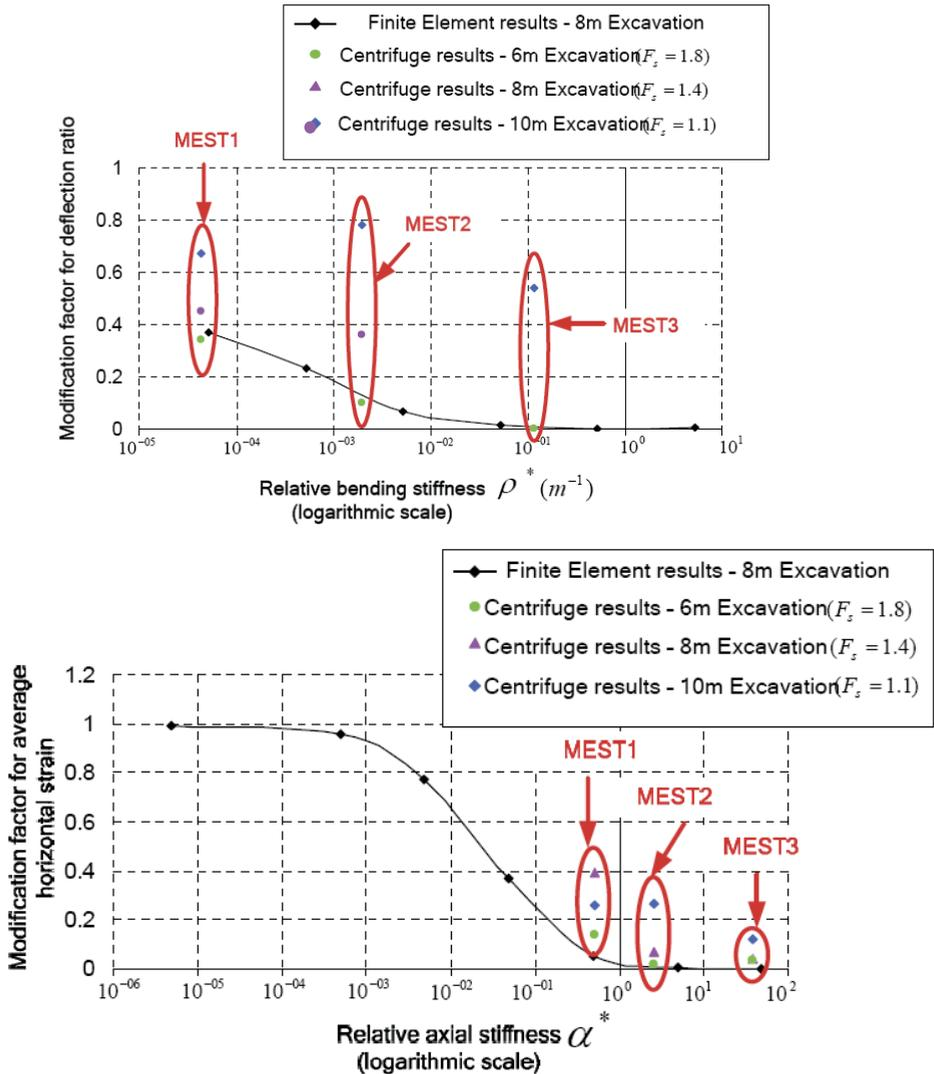
Figure 2.23 Modification factors for deflection ratio (top) and horizontal strain (bottom) from FEM and centrifuge tests (Elshafie, 2008)
