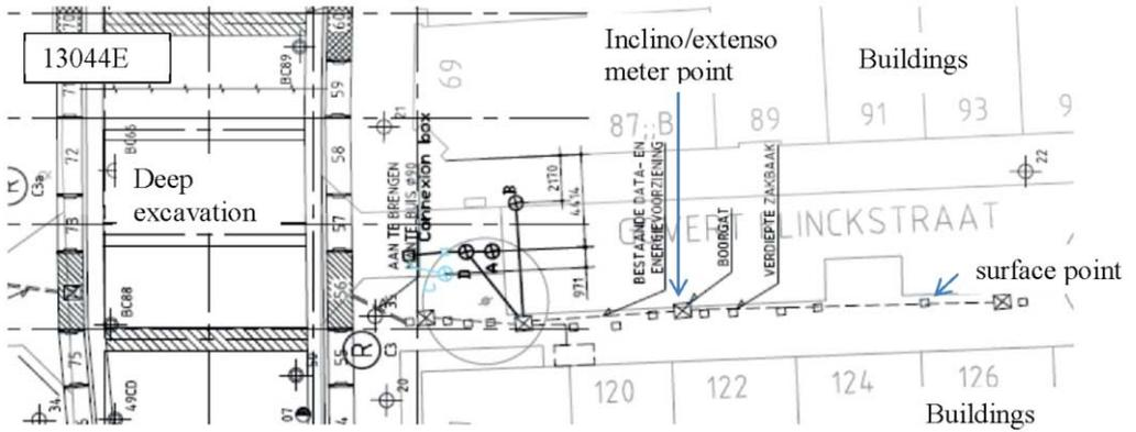
Figure 8.1 Top view of deep excavation and buildings in Govert Flinckstraat (Ceintuurbaan)
