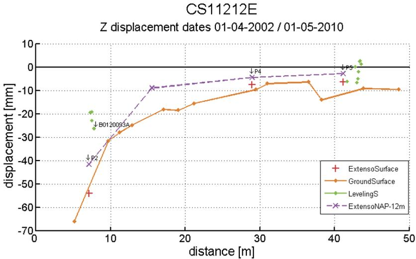
Figure 8.18 Ground and building displacements for Rokin 93 (Rokin) with distance from the deep excavation.
