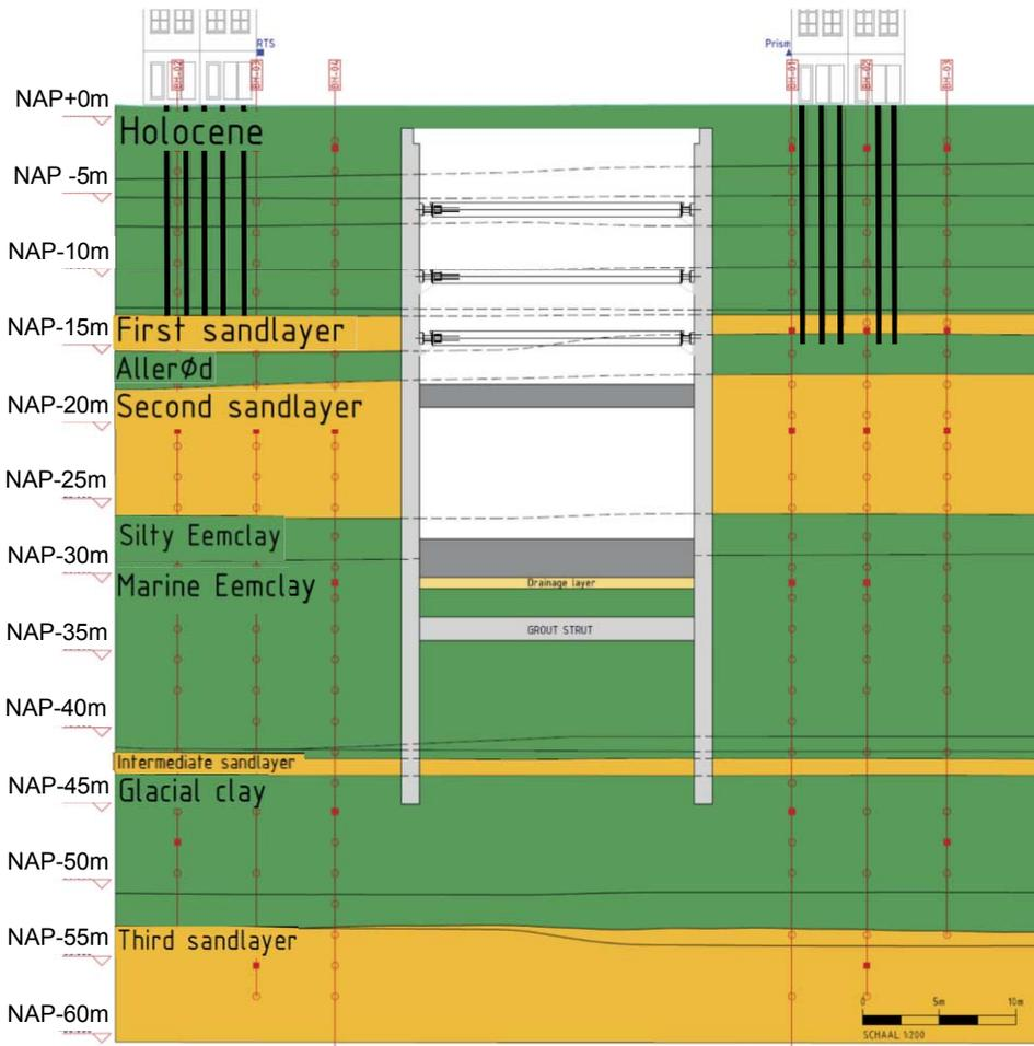
Figure 4.18 Cross section 12197
