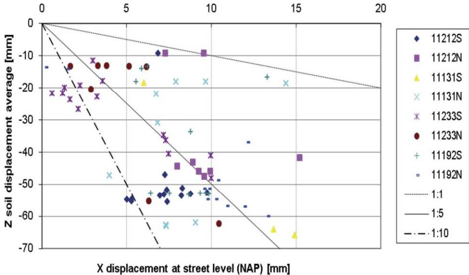
Figure 8.36 Displacements of the building in horizontal (X) direction and soil in vertical (Z) direction for Rokin station (2002-2010) with trend line (1:5), upper- and lower bound values.
