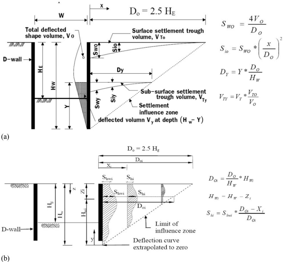
Figure 2.12 Subsurface soil displacements by Aye et al. (2006) with vertical ground displacements (a) and horizontal ground displacements (b)
