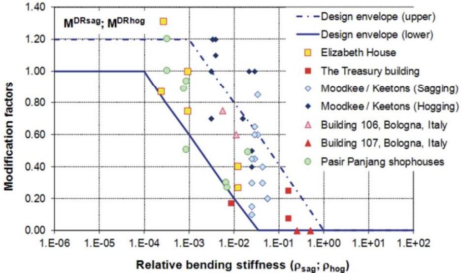
Figure 2.24 Field data of modification factor versus relative bending stiffness according to Goh (2010), Farrell (2010) and Mair (2011)
