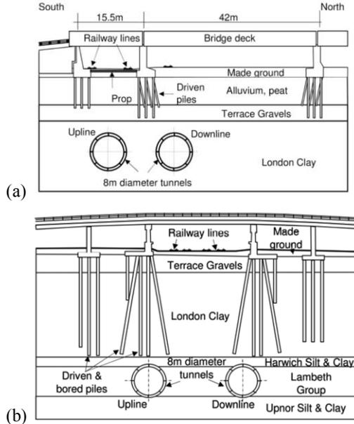
Figure 2.27 Renwick Road bridge (a) and Ripple Road Flyover (b)
