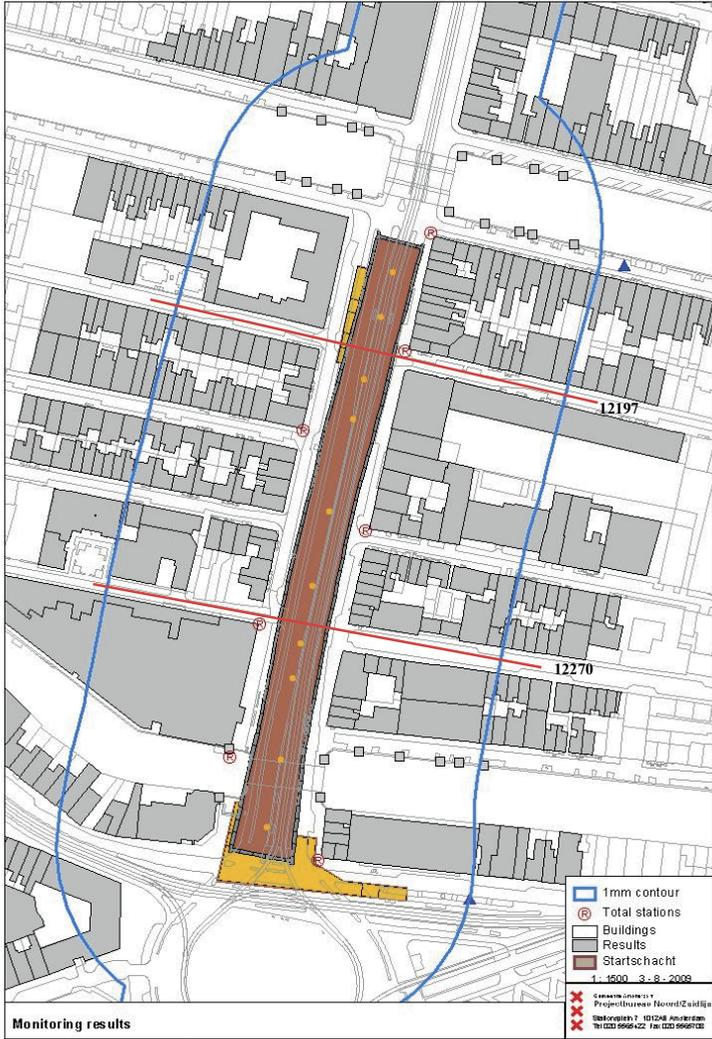
Figure 4.17 Locations of cross sections with subsurface monitoring
