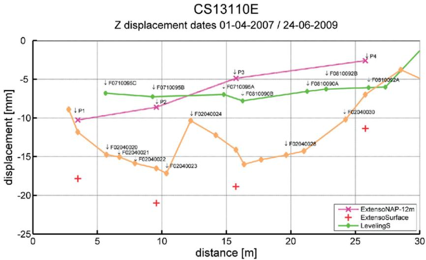
Figure 8.8 Ground and building displacements for Ferdinand Bolstraat 95 and 1e Jan van der Heijdenstraat 90-92 (Ceintuurbaan) during excavation 2007-2009 with distance from the deep excavation.
