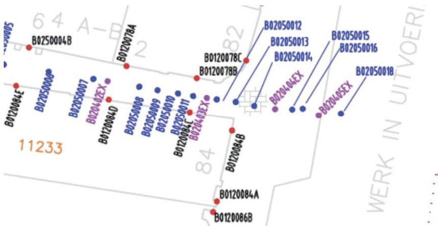
Figure 8.22 Top view of deep excavation (right) and monitoring points in cross section 11233W, Engle Kapelsteeg (Rokin)
