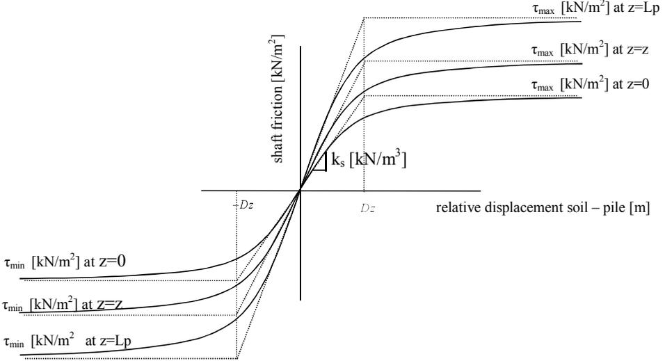
Figure 7.8 Shaft friction versus relative displacement between pile and soil, increasing with depth with constant  $Dz$
