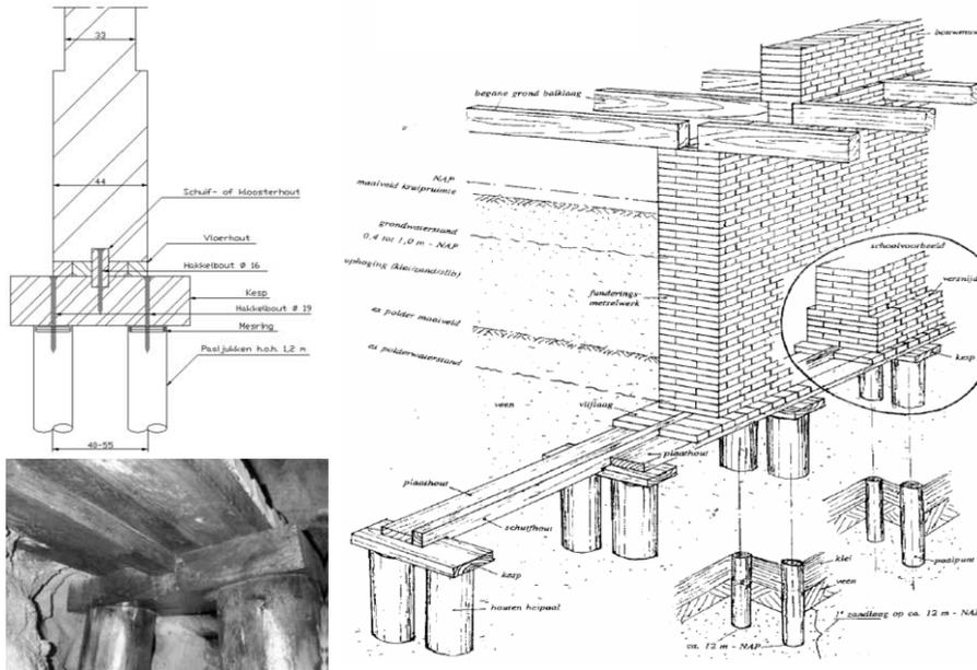
Figure 4.6 Typical Amsterdam pile system (Zantkuijl, 1993)
