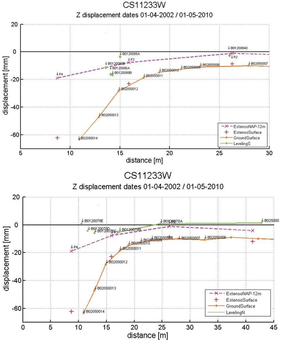
Figure 8.23 Ground and building displacements for Rokin 84-88 (top) and Rokin 82 (bottom) with distance from the deep excavation (Rokin).
