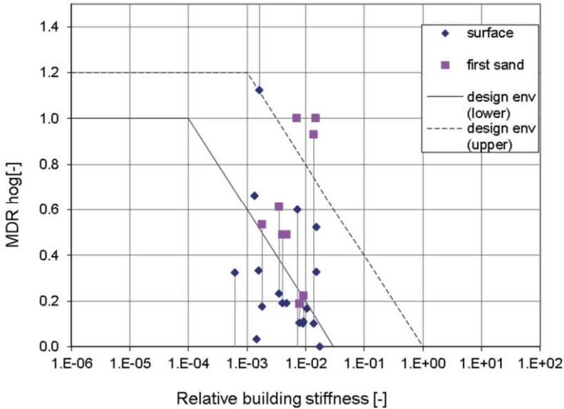
Figure 9.10 Modification factors from Amsterdam deep excavation for surface level and foundation level, compared with the design envelope presented by Mair (2011)
