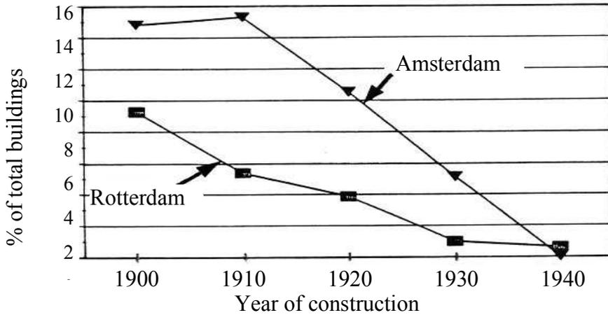
Figure 4.7 Percentage foundations with insufficient foundation quality (van Tol, 1994)
