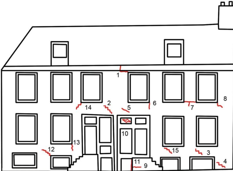
Figure 10.8 Cracks at the front façade (VZG 26 on the left side, VZG 24 on the right)
