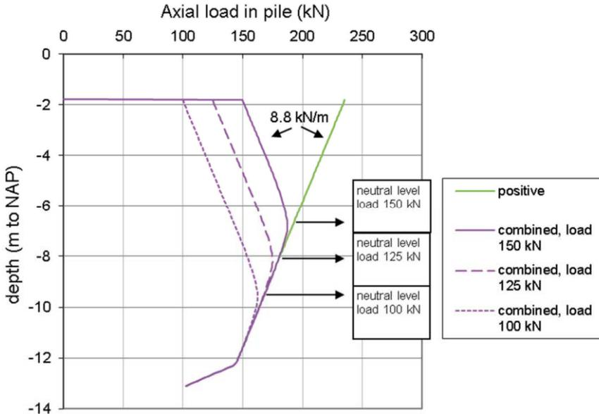
Figure 6.9 Neutral level for the new pile with pile tip at NAP -13.1 m for different pile loads with DPileGroup.
