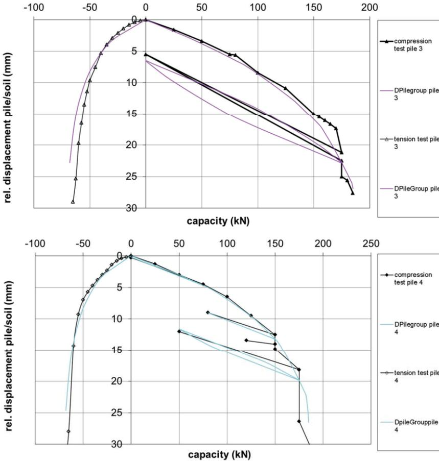
Figure 6.12 DPilegroup results based on average shaft friction and load- displacement values, compared to tests in compression and tension for old pile 3 (top) and pile 4 (below).
