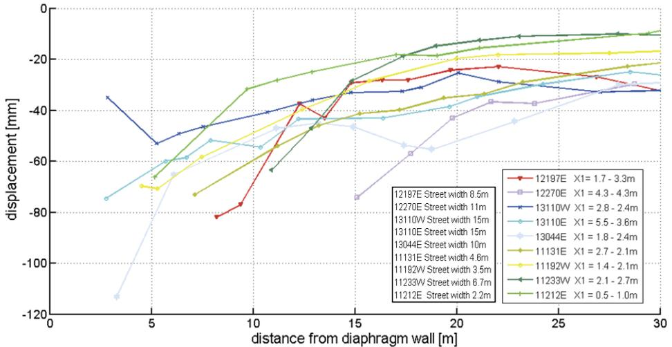
Figure 5.20 Measured surface displacements in periods 2001/2002 – 2009/2010 for three Amsterdam deep excavations with distance X1 to facades and street widths, excluding incident locations at Vijzelgracht.
