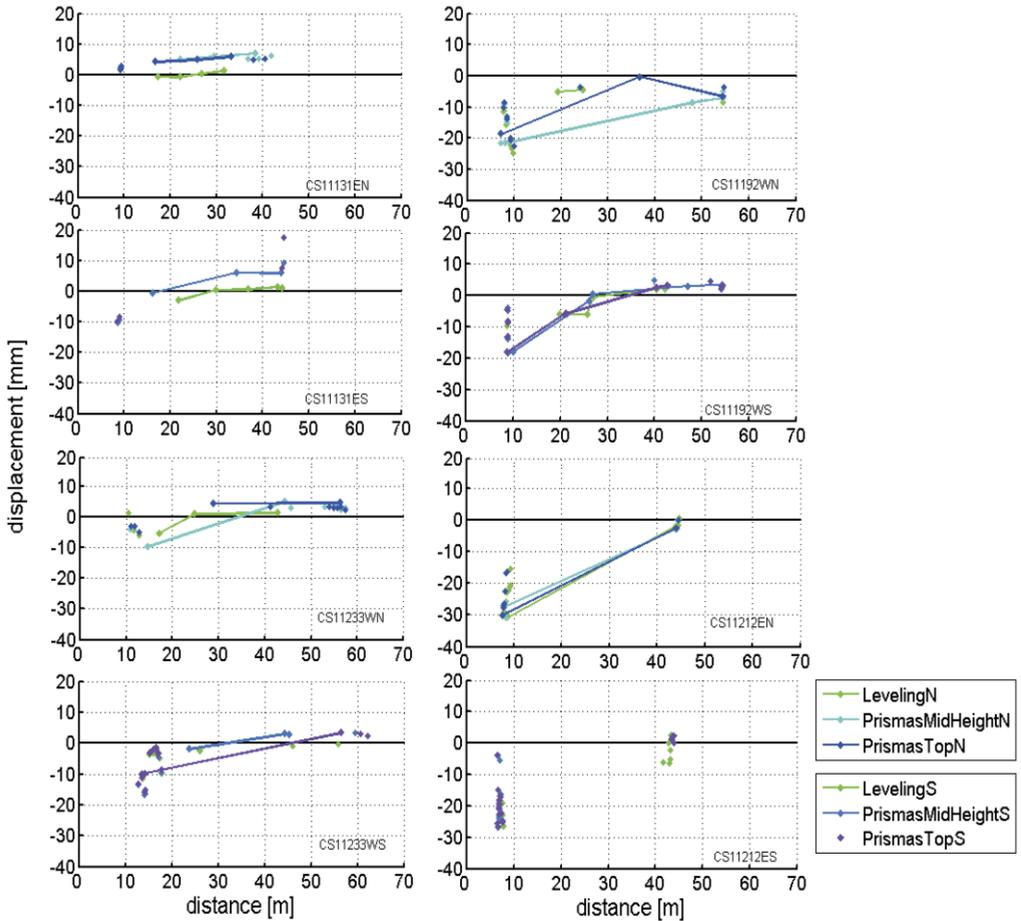
Figure 9.4 Vertical displacements from prism measurements and manual levelling for Rokin Station from 2002 - 2010
