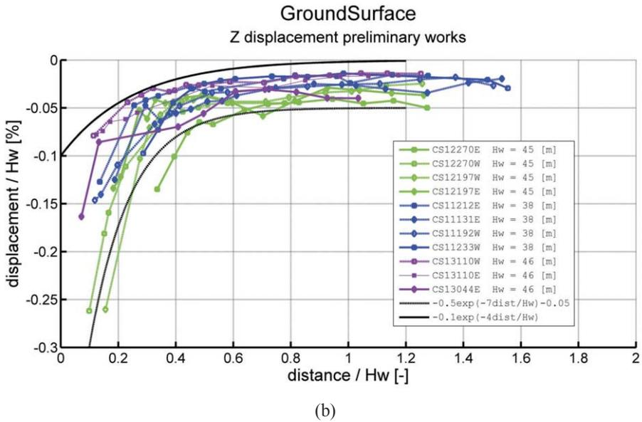
Figure 5.6 Measured surface displacements (a) and normalized surface displacements with wall depth Hw (b) for Amsterdam deep stations during preliminary activities
