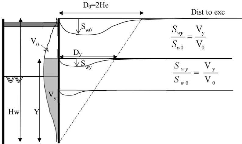
Figure 11.1 Proposed influence area for vertical soil displacements, modified from original Aye et al. (2006).
