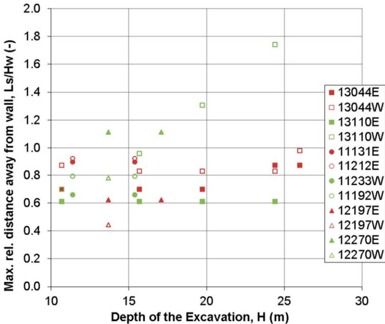
Figure 5.12 Maximum distance away from the wall to which the displacement is found normalized with the depth of the wall due to the excavation stages for the three stations
