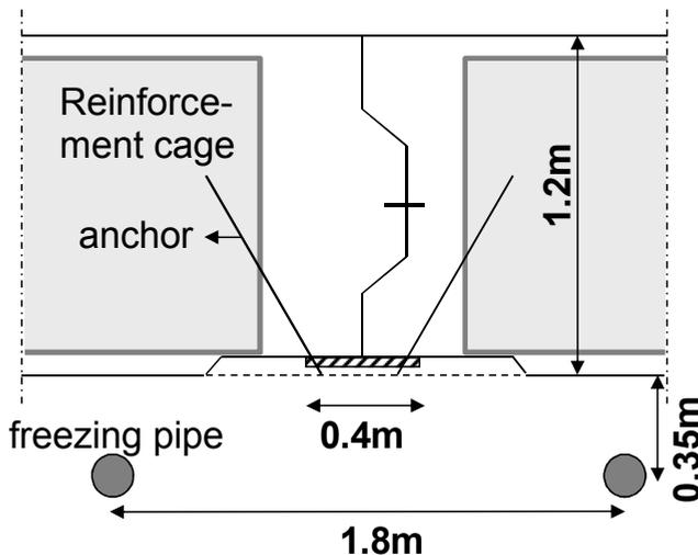
Figure 10.18 Cross section of diaphragm wall with location of freezing pipes and reinforcement cages. Steel plates (400x600x10mm) are anchored in the wall to cover the joint, after (partial) removal of the frozen soil mass and the outer skin of the diaphragm wall.
