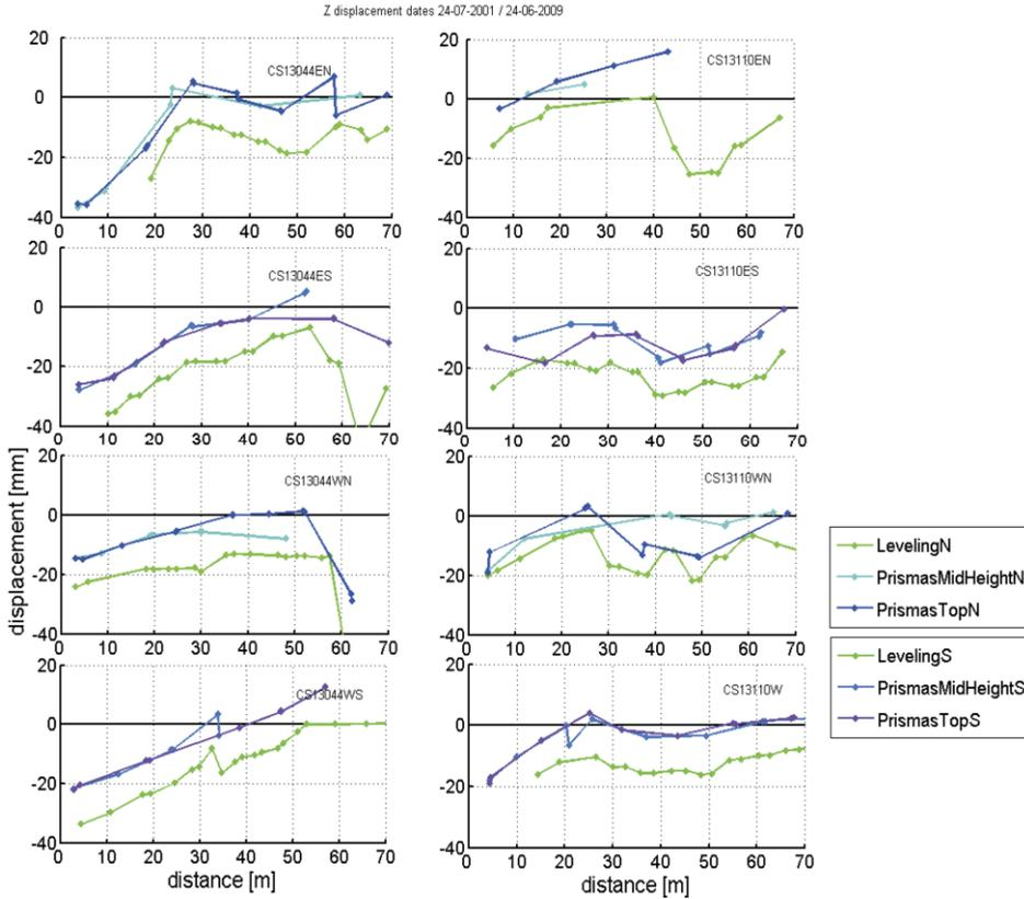
Figure 9.6 Vertical displacements from prism measurements and manual levelling for Ceintuurbaan Station from 2001-2009
