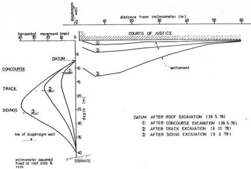
Figure 3.3 Horizontal and vertical deformations during excavation (West façade)
