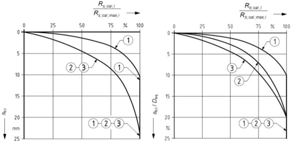
Figure 2.25 Normalised pile load curves for (1) driven piles, (2) auger piles and (3) bored piles, base load ( $R_b$ ) on the left and skin friction ( $R_s$ ) on the right
