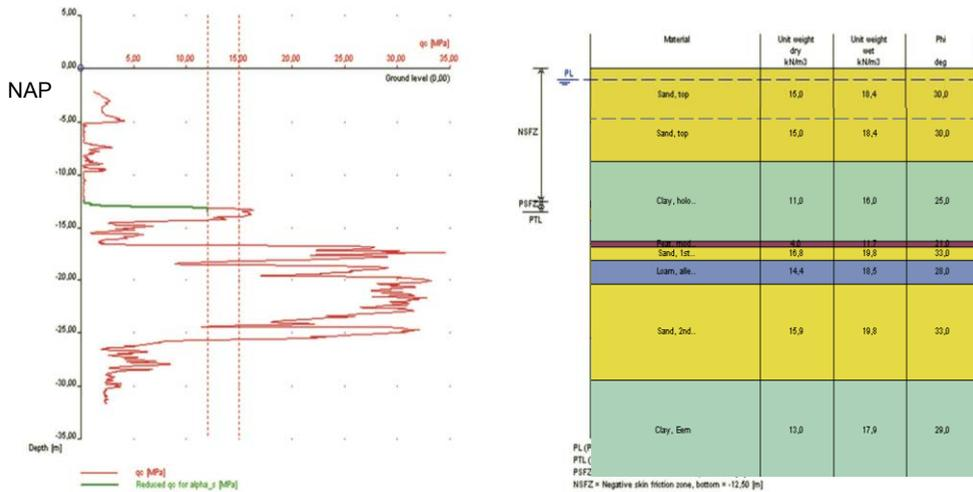
Figure 6.19 CPT and soil profile for Vijzelgracht station
