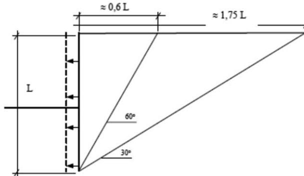
Figure 5.15 Limits of active zone according to Müller-Breslau (1906) for  $\phi'$  is  $30^\circ$
