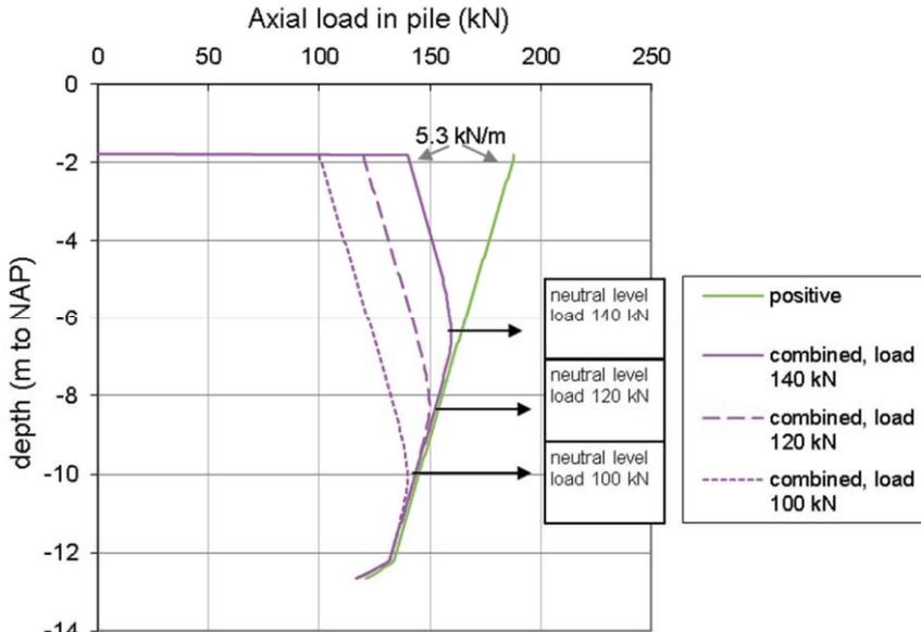
Figure 6.14 Neutral level for the old piles for different pile loads with DPileGroup.
