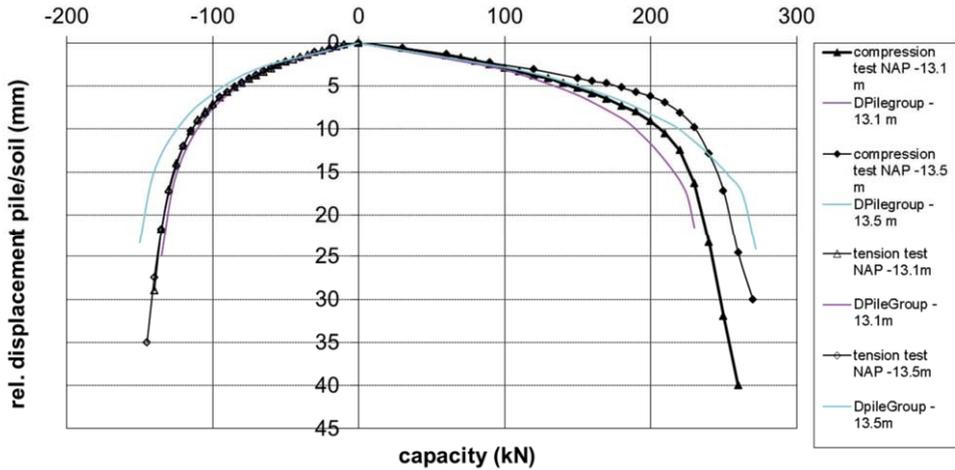
Figure 6.7 DPilegroup results based on average shaft friction and load- displacement values, compared to load displacement curves of new piles in compression and tension
