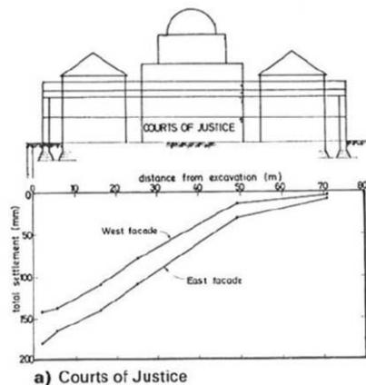
Figure 3.4 Building deformations (final stage, East and West perpendicular to excavation)
