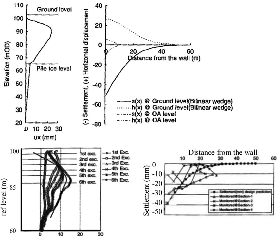
Figure 3.6 Predicted (above) and measured (below) deformations (Lee et al., 2007)
