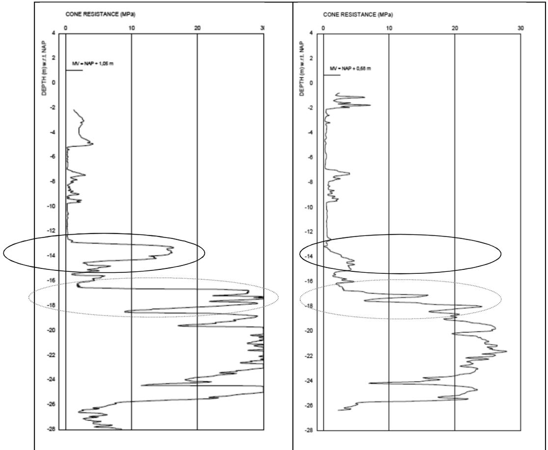
Figure 10.3 CPT before (left) and CPT after (right) first leakage incident showing large reductions in first sand layer (at -14m) and top of second sand layer (at -17m). The CPT before the incident is representative for a larger area as the first and second sand layers very consistently show  $q_c$  values of 10-20 MPa and over 20 MPa respectively.
