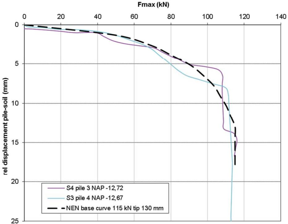
Figure 6.11 Base load displacement curves for Pile 3 and Pile 4 (old piles, not broken)
