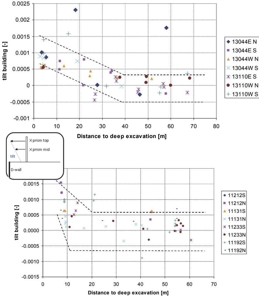
Figure 9.14 Tilt of buildings in direction of excavation during period 2001-2009 at Ceintuurbaan station (top) and Rokin (bottom)
