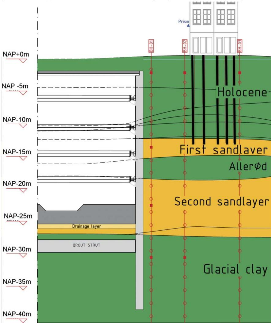
Figure 4.10 Cross section of Rokin Station (at km 11212)
