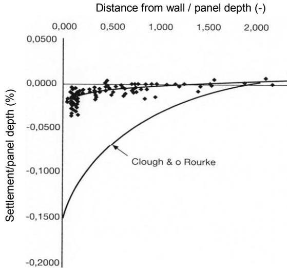
Figure 2.14 Settlement due to installation of a diaphragm wall (Ter Linde, 1999)
