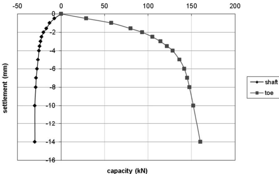
Figure 6.15 Pile load results according to TNO (1995)
