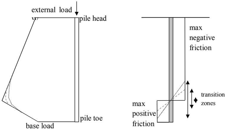
Figure 7.2 Theoretical axial load (left) and shaft friction (right) along pile for different lengths of the transition zone
