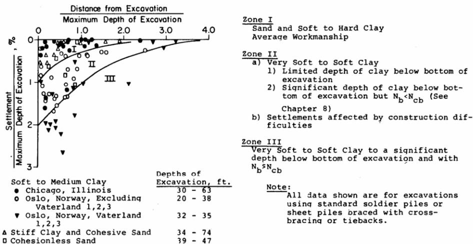
Figure 2.2 Settlements caused by all activities relating to deep excavations in various soils by Peck (1969)
