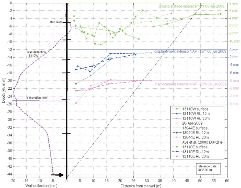
Figure 5.13 Measured deflection  $D_{wall}$  (horizontal) and ground displacement at different levels (vertical) for three cross sections at Ceintuurbaan Station. Influence zone as described by Aye et al. (2006) but with  $D_0=2H_e$  instead of  $2.5H_e$  is shown in black striped diagonal line.
