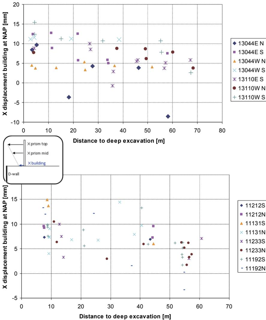
Figure 9.13 Horizontal displacement of buildings at street level during period 2001-2009 at Ceintuurbaan station (top) and Rokin (bottom)
