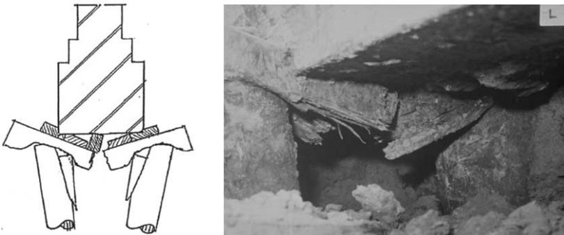
Figure 4.8 Foundation failure due to collapse of the cross beam
