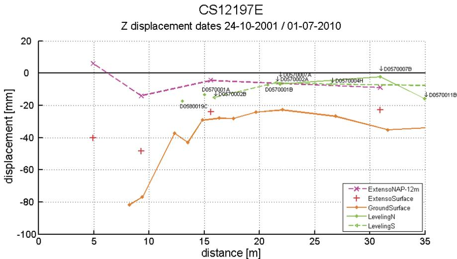
Figure 8.26 Ground and building displacements for Noorderstraat (Vijzelgracht) with distance from the deep excavation.
