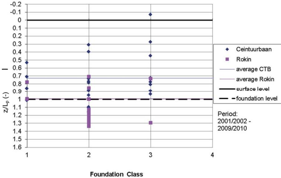
Figure 8.30 Interaction level versus Foundation Class (1: good quality , 2: reasonable, 3: moderate, 4: unacceptable)
