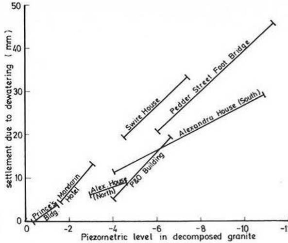
Figure 3.2 Settlement of high-rise buildings due to dewatering
