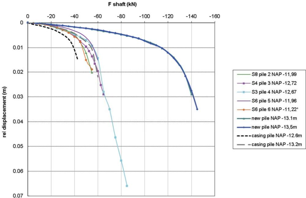
Figure 6.3 Results pile tests in compression shown in (a) for shaft + base, and in tension shown in (b) (shaft capacity)
