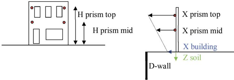
Figure 8.35 Horizontal displacement of building at street level (left: front view, right: side view)
