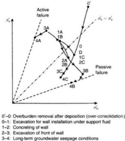
Figure 2.29 Stress changes in four locations in an over-consolidated clay with diaphragm wall; A at the active side, B at the passive side, C in the centre of the excavation and D at large distance from the excavation (Puller, 2003)
