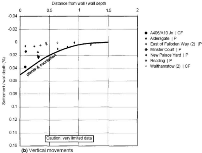
Figure 2.15 Vertical displacements due to diaphragm wall installation (Gaba et al. 2003)
