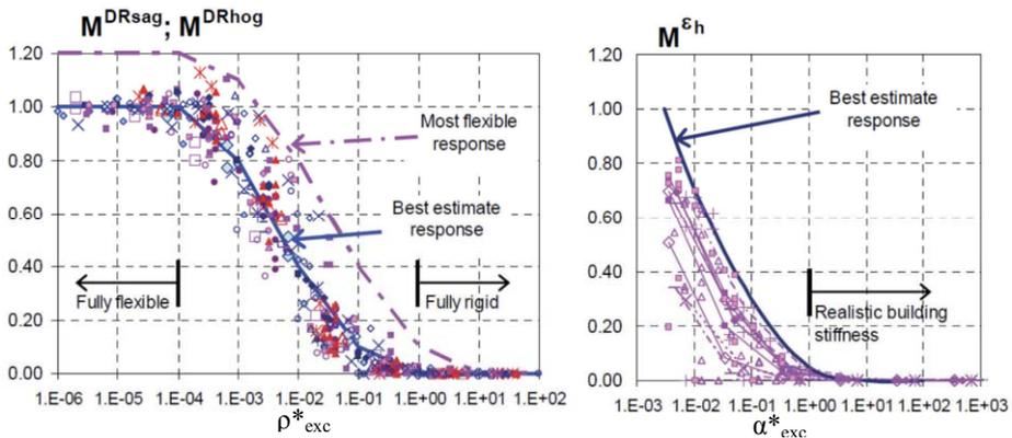
Figure 2.21 Design curves from Goh (2010) based on modified modification factors
