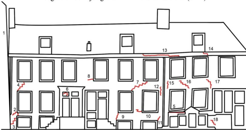
Figure 10.12 Cracks at the front façade VZG 8 -6 - 4
