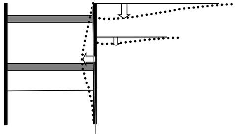
Figure 5.1 Simplified interaction between excavation and vertical ground displacement
