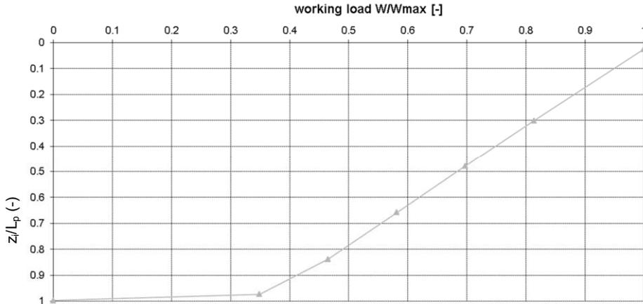
Figure 8.5 Typical  $z_i/L_p$  values for pile at Ceintuurbaan with initial negative and positive skin friction fully developed due to subsidence based on DPileGroup calculation.
