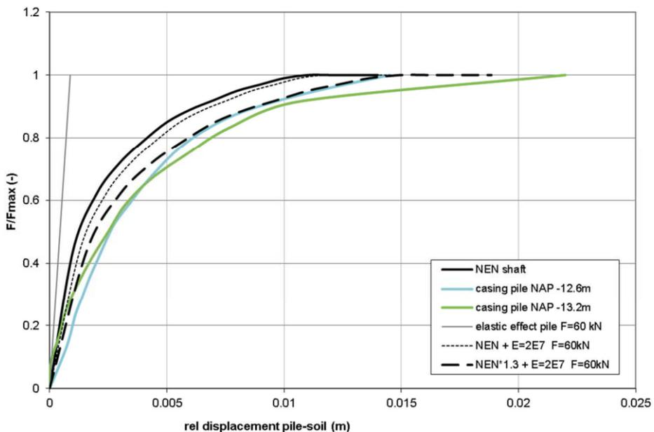
Figure 6.4 Shaft friction in sand; measured in tension test for casing pile and calculated according to Dutch code NEN for displacement piles
