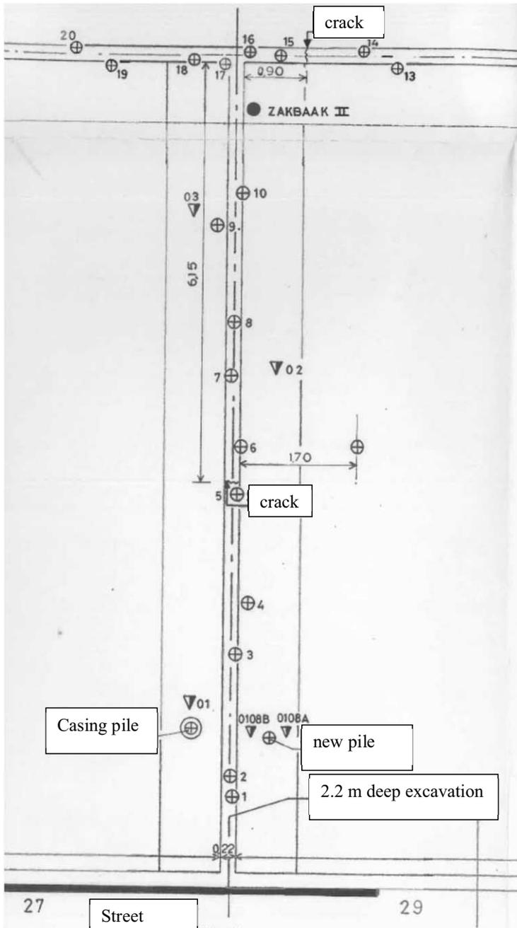
Figure D.1 Pile and CPT locations Dapperbuurt top view
