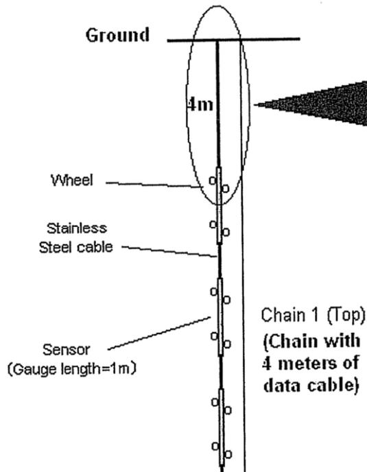
Figure 4.41 String of inclinometer sensors
