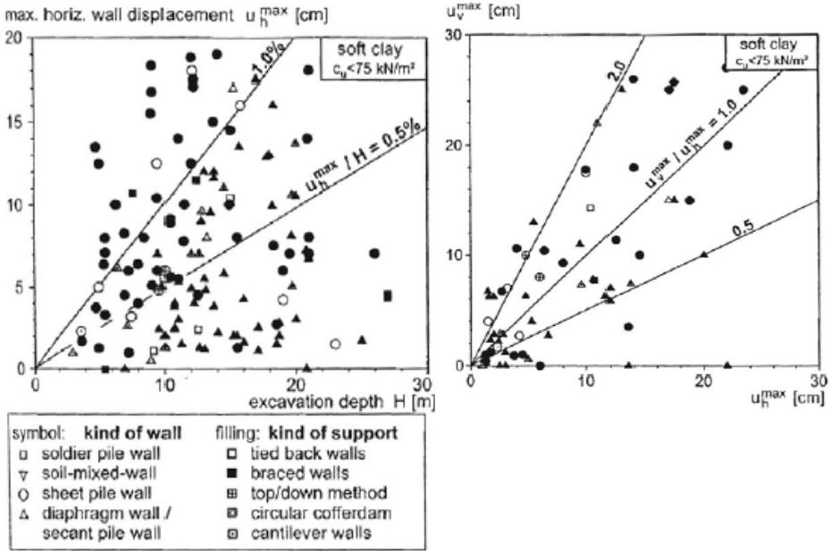
Figure 2.8 Horizontal displacement as a function of excavation depth (left) and versus vertical displacement (right) (Moormann and Moormann, 2002).
