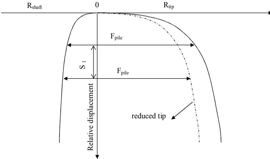
Figure 7.1 Load –displacement curve for a pile with constant load  $F_{\text{pile}}$ , and subsequent settlement  $S_1$ .
