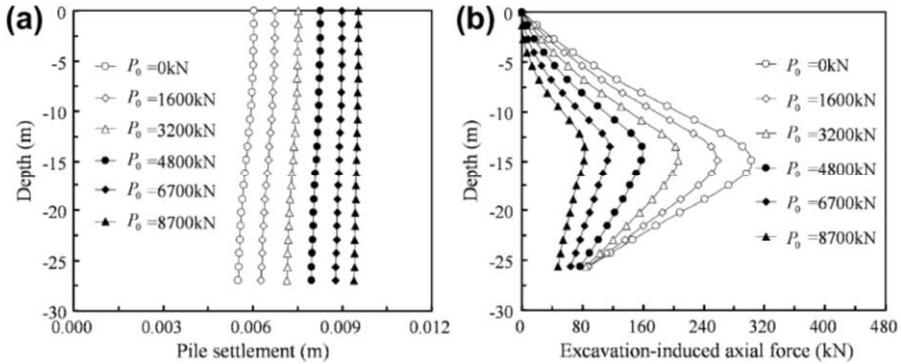
Figure 2.30 Zhang (2010) model for lateral and axial excavation induced effects with a) pile deformation with depth and b) pile axial force, both for different working loads ( $P_0$ )
