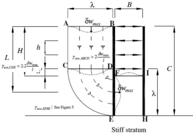
Figure 5.18 Incremental displacement field for narrow excavations (Bolton et al., 2008)
