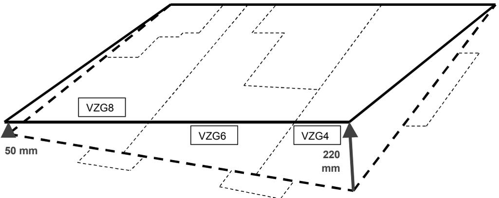
Figure 10.17 Jacking plan with main lift direction from De Nijs and Kaalberg (2010)
