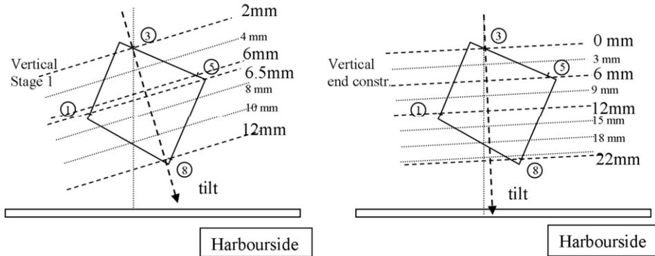
Figure 3.16 Vertical deformation of White House (left after stage 1, right at end of construction) with direction of tilt indicated
