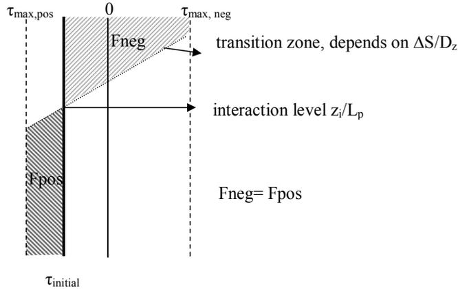
Figure 7.12 Example of development of positive and negative shaft friction due to an excavation.
