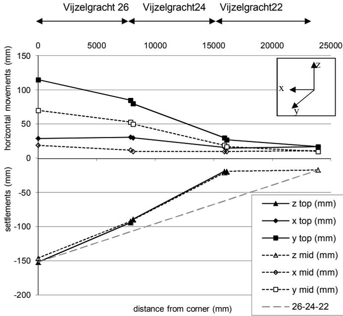
Figure 10.7 Deformations after incident June 2008 (measurements dated July, 31st 2008)
