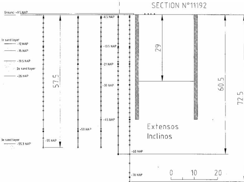
Figure 4.39 Cross section of inclinometers and extensometers (example from ABNZL)
