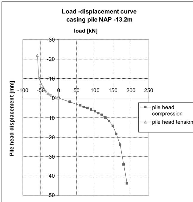
Figure D.4 Pile load test results on new piles
