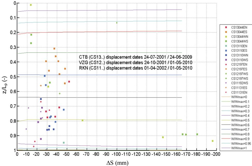
Figure 8.34 Interaction level versus ground settlement difference  $\Delta S$  (ground settlement at surface level minus ground settlement at pile tip level) and numerically determined lines of equal  $W/W_{max}$  values
