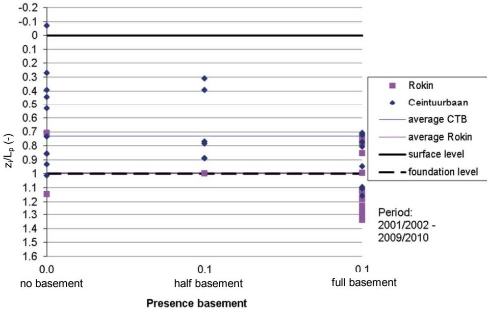
Figure 8.33 Interaction level versus presence of basement
