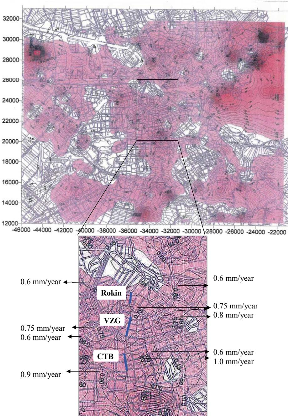
Figure 4.3 NAP –levels and their settlement in mm/year referenced to the second sand layer and their settlement in mm/year at location of deep stations (Hogenes, 1998)
