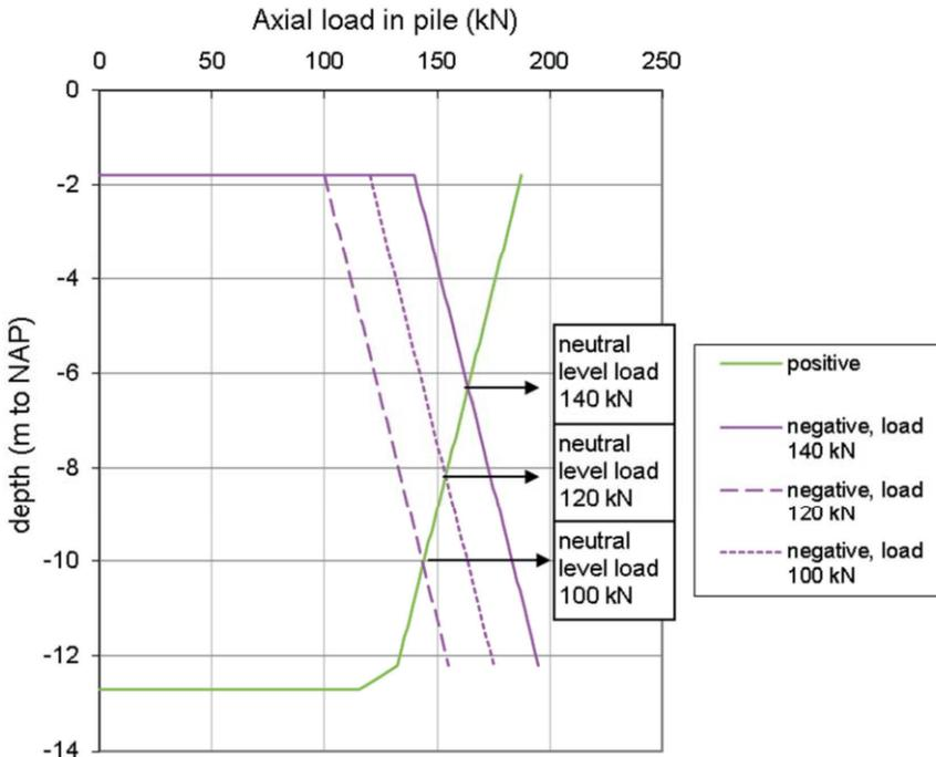
Figure 6.13 Neutral level for the old piles for different pile loads.
