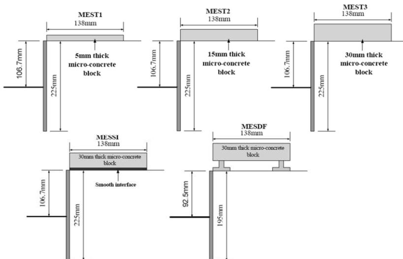
Figure 2.22 Buildings and interfaces used in centrifuge tests (Elshafie, 2008)
