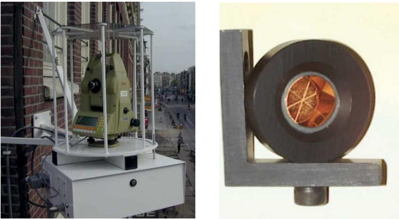
Figure 4.31 Robotic Total Station and prism
