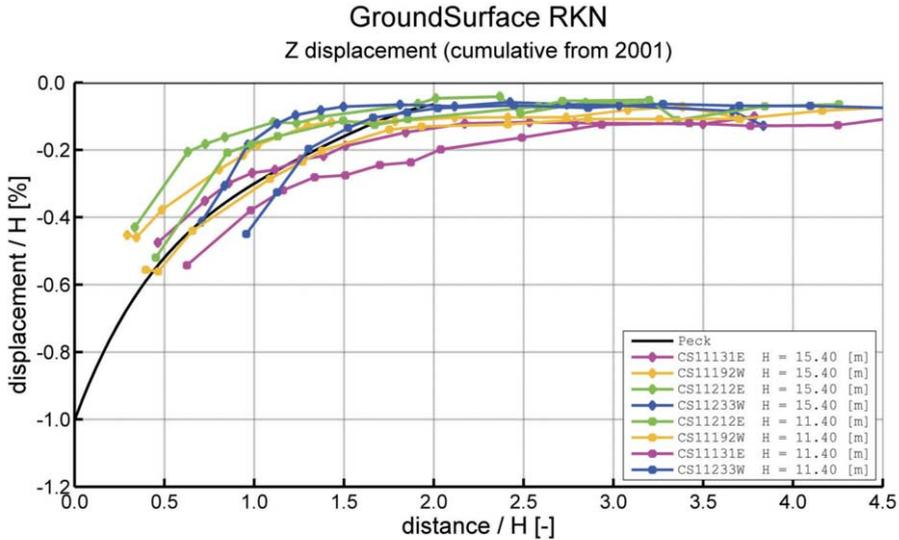
Figure 5.3 Soil displacements normalized with excavation depth  $H$ , compared with envelopes by Peck (1969) for Ceintuurbaan Station (a), Vijzelgracht Station (b) and Rokin Station (c)
