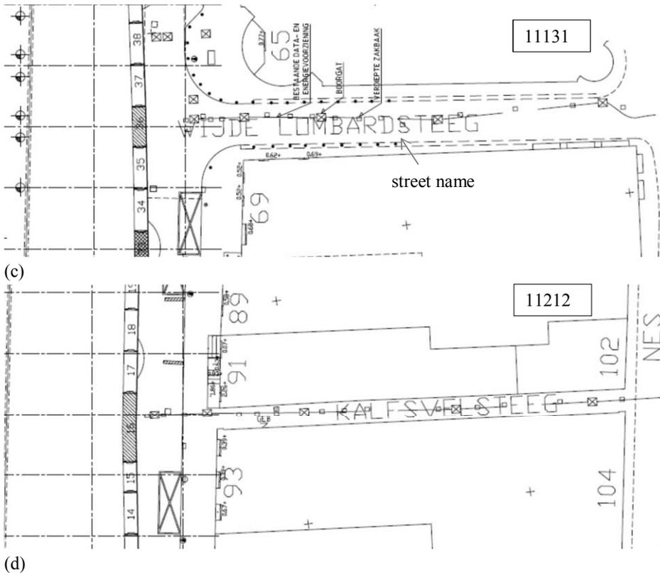
Figure 4.12 Top view of monitoring cross sections 11192, 11233, 11131 and 11212 with inclinometer/extensometer borehole locations and surface measurement points
