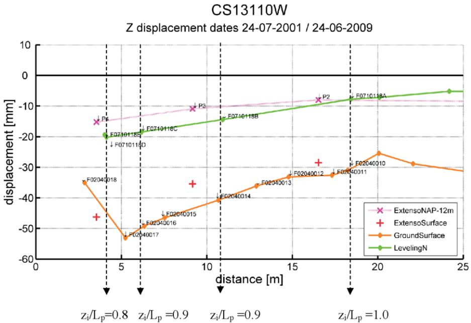
Figure 8.14 Ground and building displacements for Ferdinand Bolstraat 118 (Ceintuurbaan) with distance from the deep excavation, showing interaction levels ( $z_i/L_p$ ) derived from measurements
