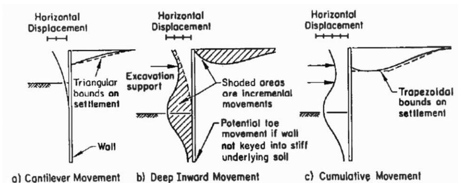
Figure 2.4 Typical profiles of movement for braced and tied-back walls (Clough and O'Rourke, 1990)
