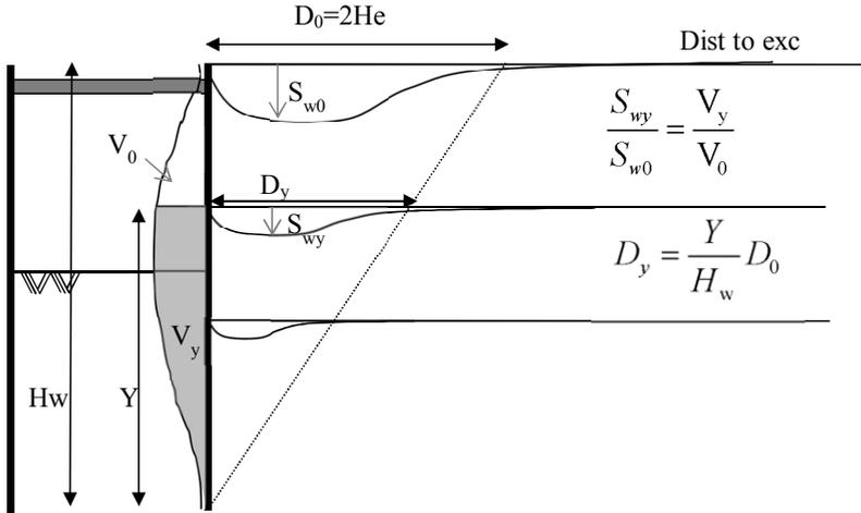
Figure 5.21 Proposed influence area for vertical soil displacements, modified from original Aye et al. (2006).
