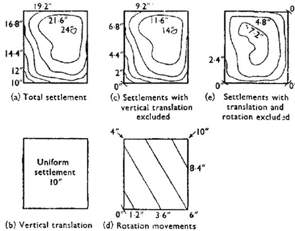
Figure 2.20 Building deformation including uniform settlement and tilt (Skempton and McDonald, 1956)
