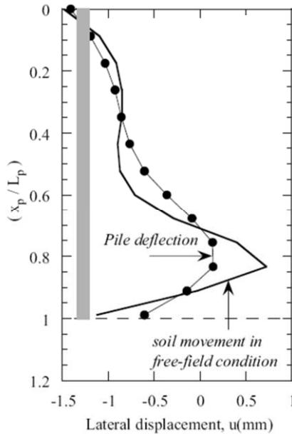
Figure 2.28 Lateral deformation of pile compared to soil with depth (Mroueh and Shahrour 2002)
