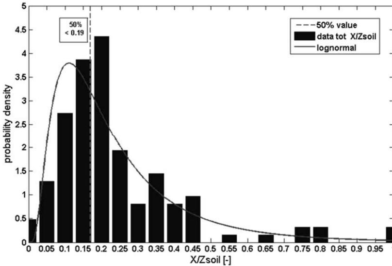
Figure 8.37 Histogram plots and best-fit lognormal distribution for probability of  $X/Z_{soil}$  values for Rokin Station and Ceintuurbaan Station combined
