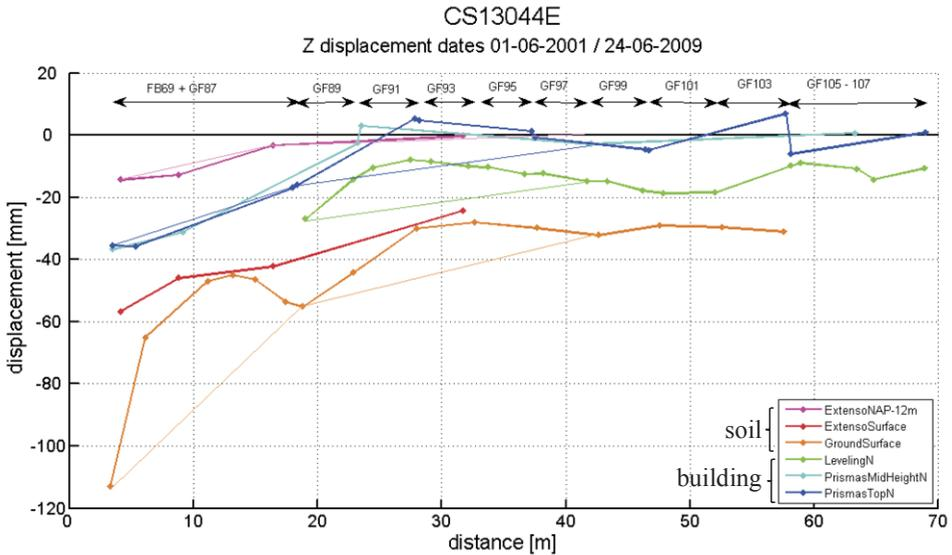
Figure 9.9 Building and soil deformations 2001-2009 Ceintuurbaan Station 13044E (other cross sections in Annex E)
