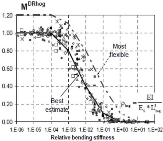
Figure 9.8 Modification factor for bending in hogging based on FE-analysis by Goh and Mair (2011)
