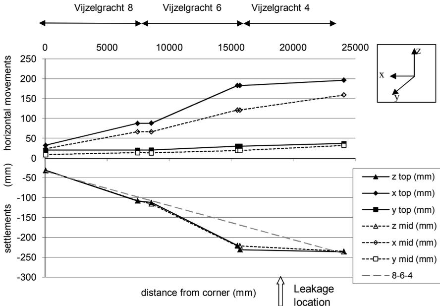
Figure 10.13 Deformations after second incident (measurements dated 29th October 2008)
