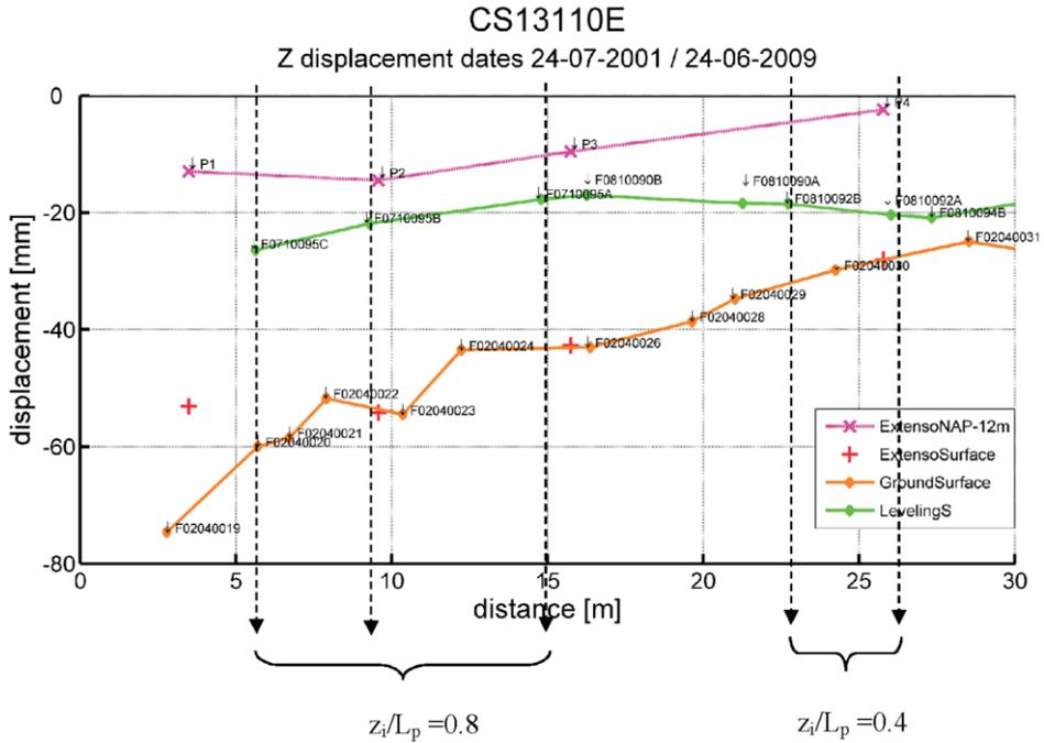
Figure 8.6 Ground and building displacements for Ferdinand Bolstraat 95 and 1e Jan van der Heijdenstraat 90-92 (Ceintuurbaan) in the period 2001-2009 with distance from the deep excavation, with interaction level  $z_i/L_p$  derived from measurements
