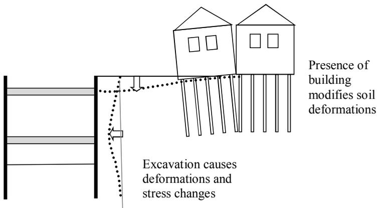
Figure 2.1 Interaction between excavation and adjacent buildings
