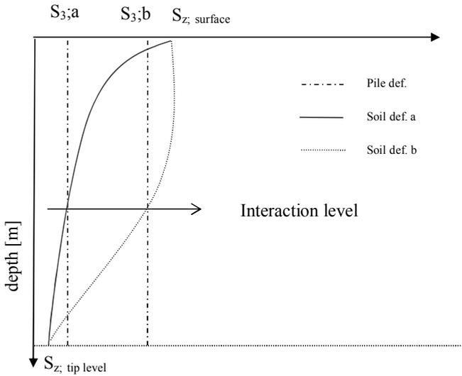
Figure 7.6  $S_3$  based on a non-linear settlement profile and known interaction level
