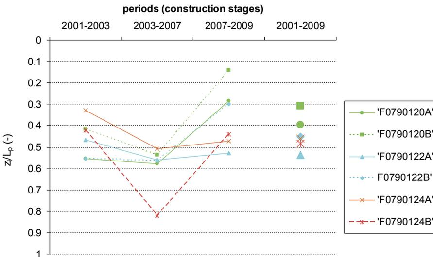
Figure 8.4 Depth  $z_i/L_p$  at which the ground and building settlement are similar for each of the construction stages for Govert Flinkstraat 120-124 (Ceintuurbaan)
