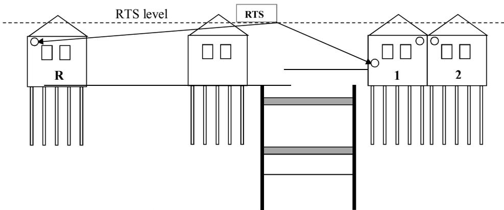
Figure 4.42 Reference levels of automatic and manual measurements
