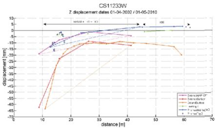
Figure E.3 Building and soil deformations 2002-2010 Rokin Station
