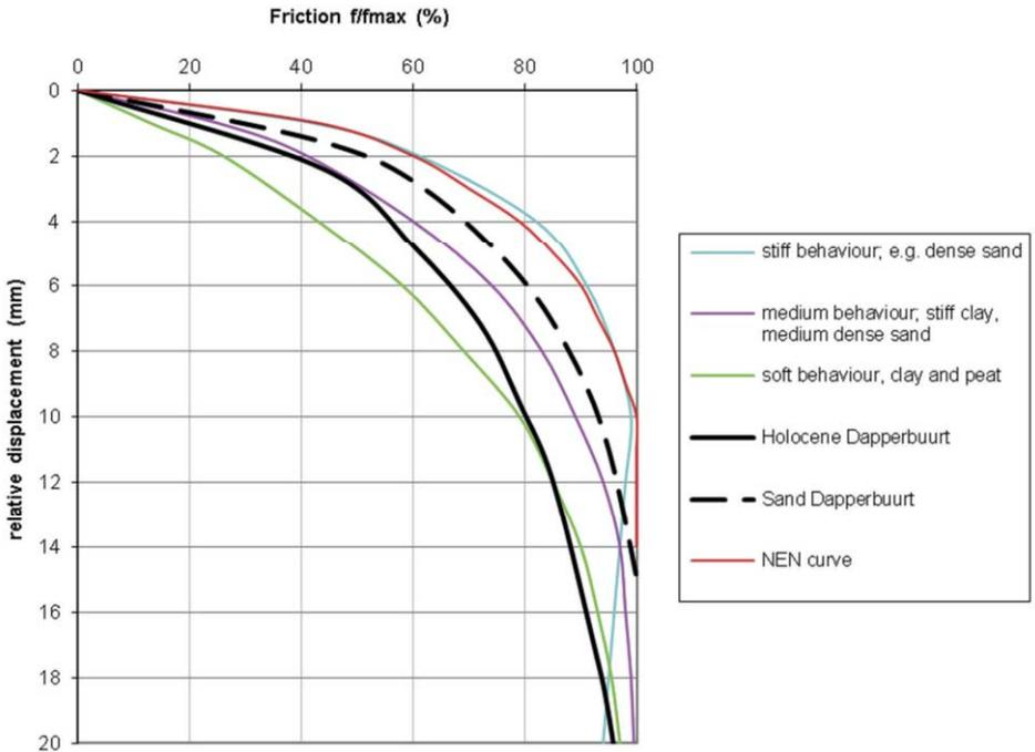
Figure 6.18 Shaft friction development based on Dapperbuurt and Van Weele and Riethoff (1982)
