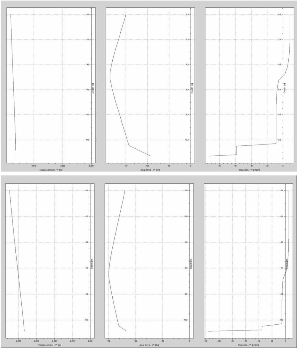
Figure D.8 Result of DPileGroup for neutral level new pile 150 kN (top) and old pile 120 kN (bottom)
