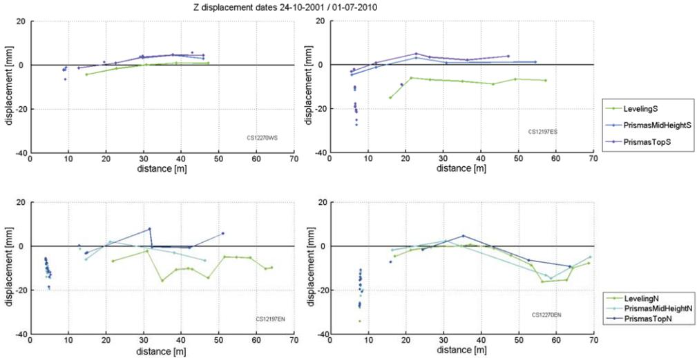
Figure 9.5 Vertical displacements from prism measurements and manual levelling for Vijzelgracht Station from 2001-2010
