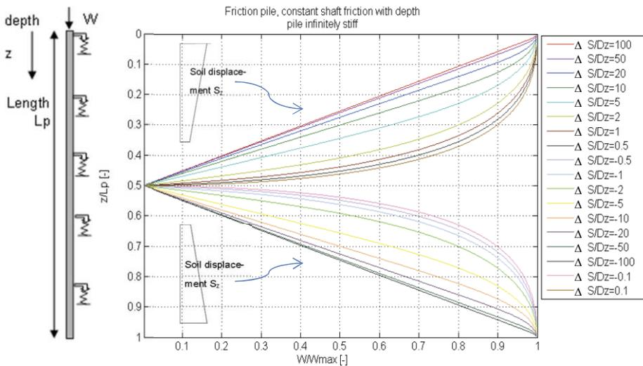
Figure 7.7 Relationship between  $z_i/L_p$  and  $W/W_{max}$  for different values of  $\Delta S/D_z$  for a friction pile with infinite stiffness and constant shaft friction with depth.
