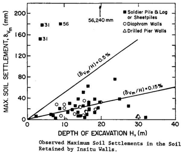
Figure 5.4 Observed maximum wall deflection and settlements for stiff clays, residual soils and sands (Clough and O'Rourke, 1990)
