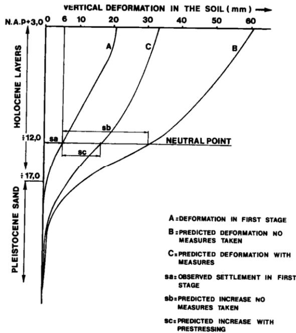
Figure 3.15 Calculated soil deformations with depth White House (Brassinga and van Tol, 1991)
