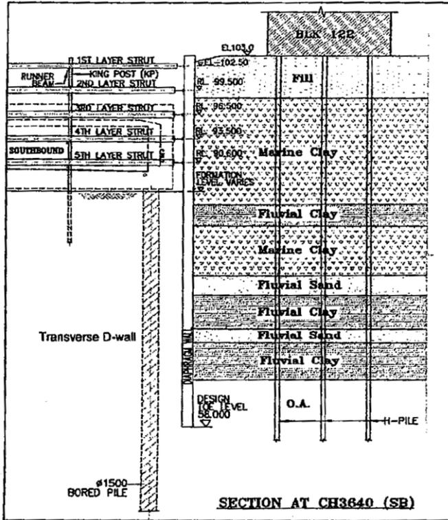
Figure 3.5 Cross section with the geological profile
