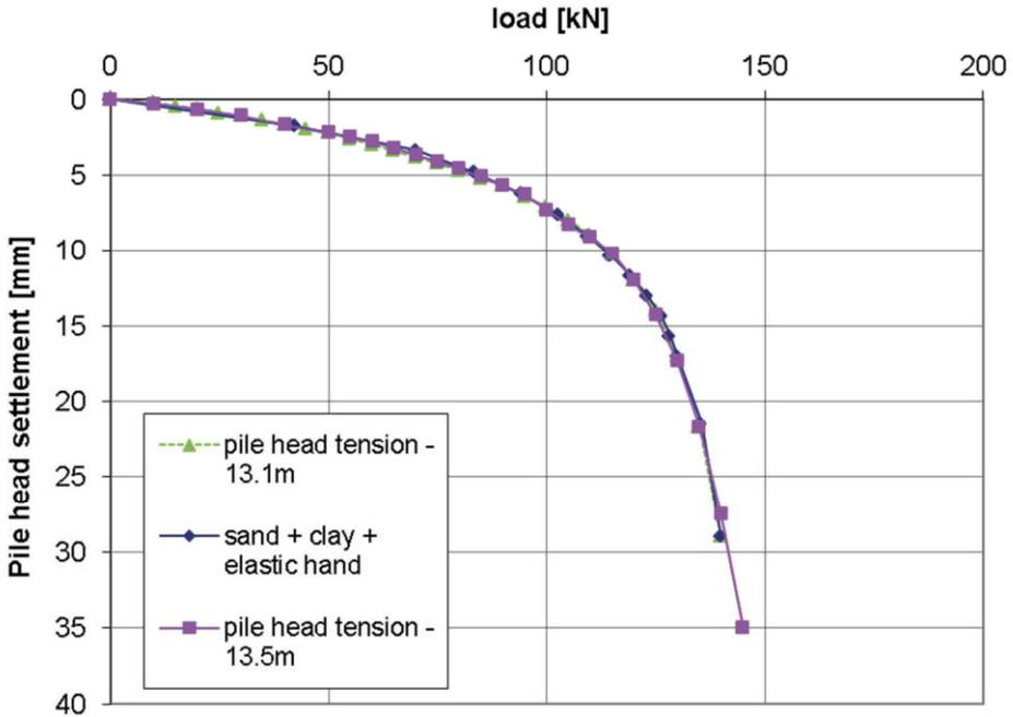
Figure 6.5 Shaft friction in new piles with NAP -13.1 m and NAP -13.5m (tension tests) and fit with NEN curve factored 2.1 times
