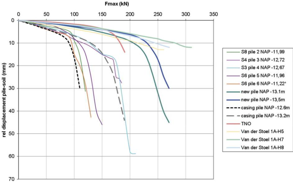
Figure 6.17 Pile test results in compression from TNO, Van der Stoel and Dapperbuurt combined
