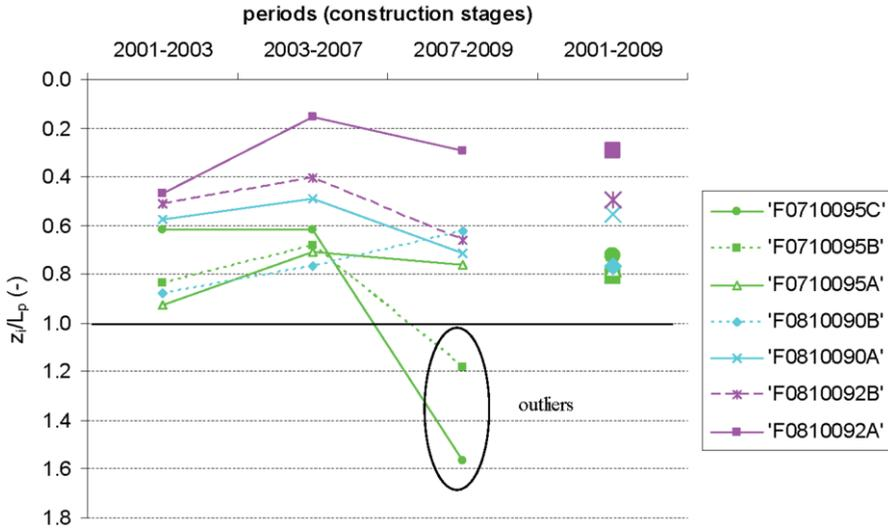
Figure 8.7 Depth  $z_i/L_p$  at which the ground and building settlement are similar for each of the construction stages Ferdinand Bolstraat 95 and 1e Jan van der Heijdenstraat 90-92 (Ceintuurbaan)
