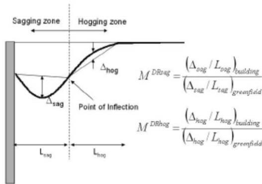
Figure 9.7 Hogging and sagging zones for deep excavation
