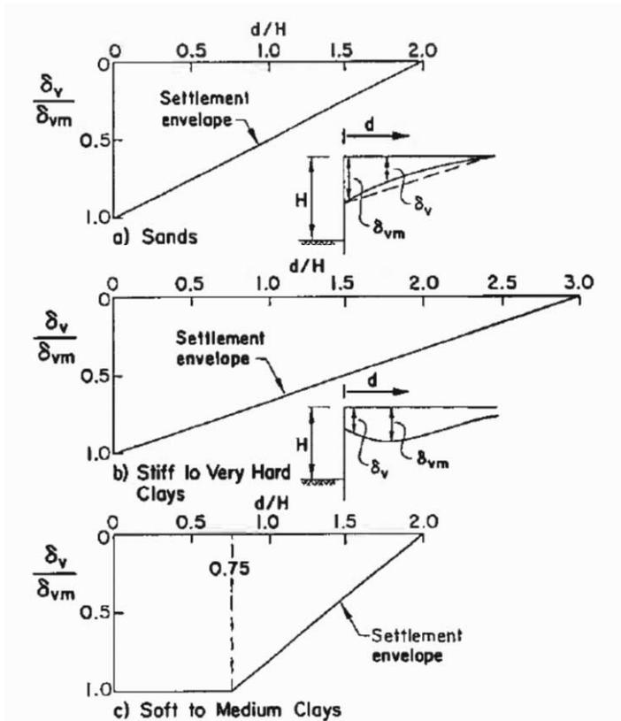
Figure 2.7 Dimensionless envelopes of settlement profiles for estimating settlement adjacent to excavations in different soil types (Clough and O'Rourke, 1990)
