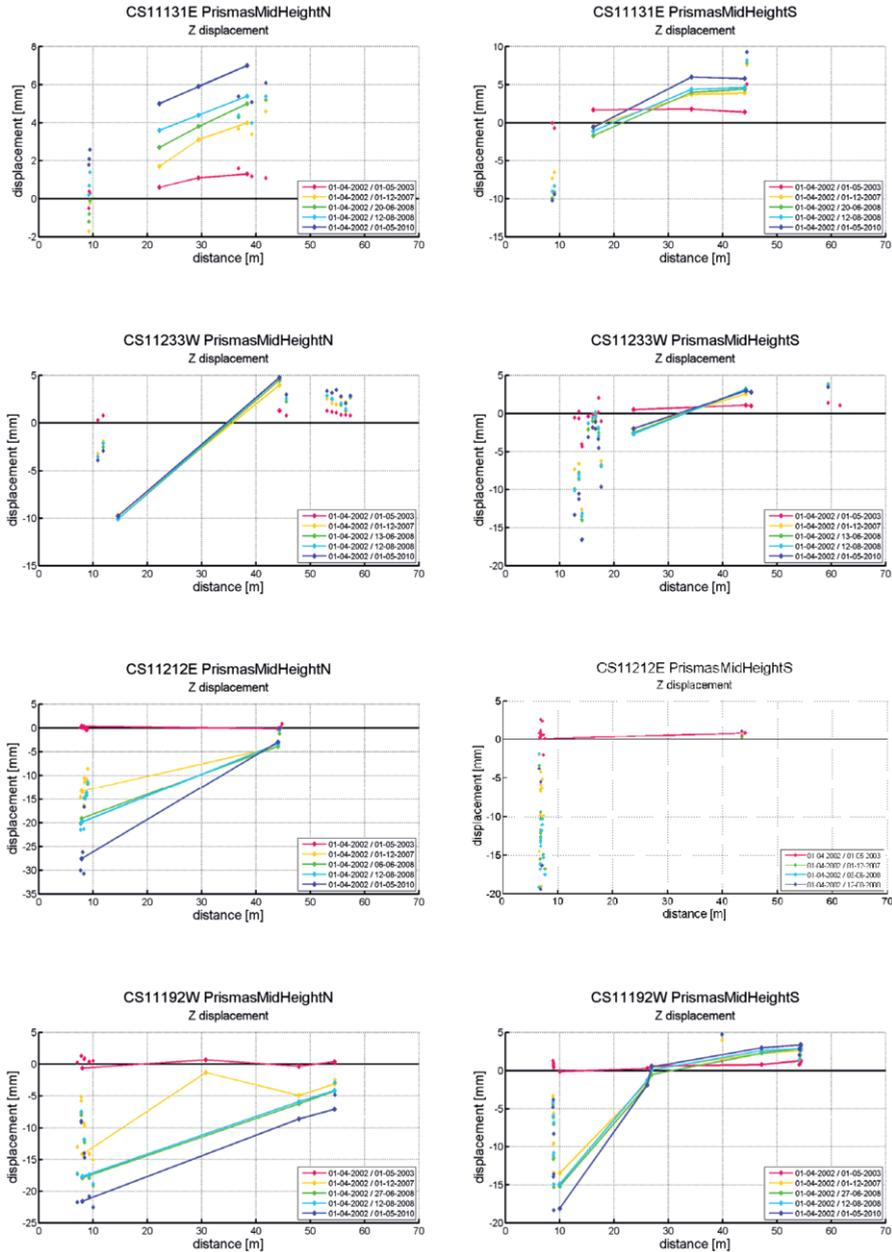
Figure 9.3 Building deformations with time Rokin Station
