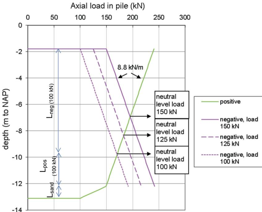
Figure 6.8 Neutral level for the new pile with pile tip at NAP -13.1 m for different pile loads.
