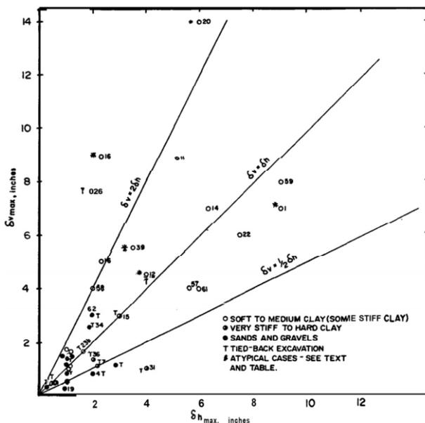
Figure 2.3 Wall deflection compared to ground settlements for soft soils by (Goldberg et al., 1976)
