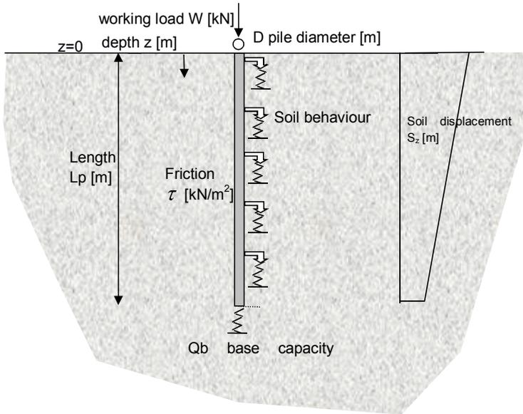
Figure 7.4 Model schematization and parameters
