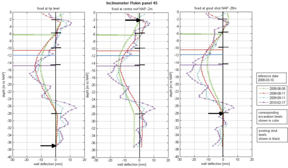
Figure 4.43 Inclinometer results with different fixation levels
