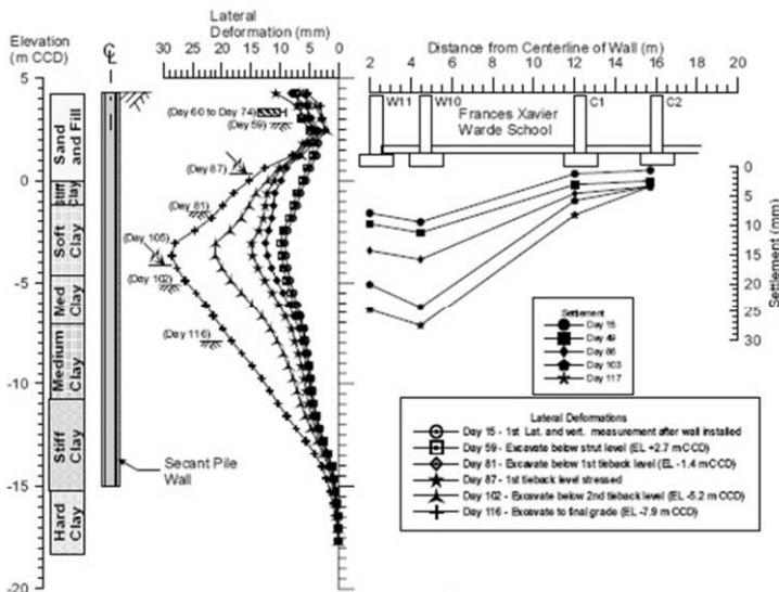
Figure 3.8 Comparing settlements and inclinometer data at the end of the excavation (Inclinometer 1)
