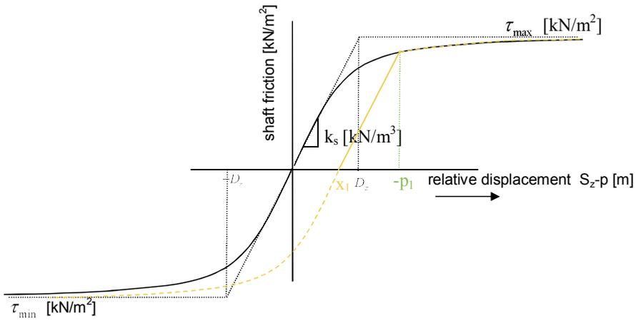
Figure 7.5 Shaft friction versus relative displacement between pile and soil
