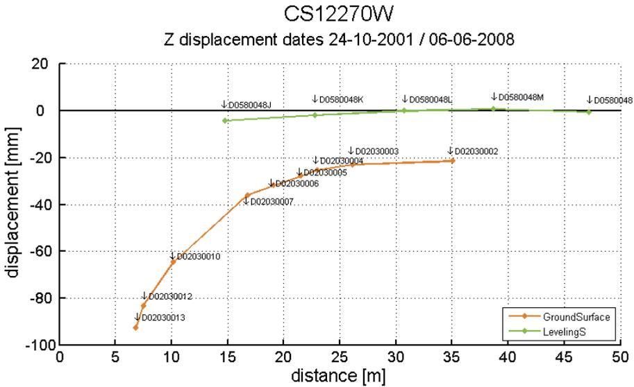
Figure 8.29 Ground and building displacements for Vijzelgracht 48 (Vijzelgracht) with distance from the deep excavation.
