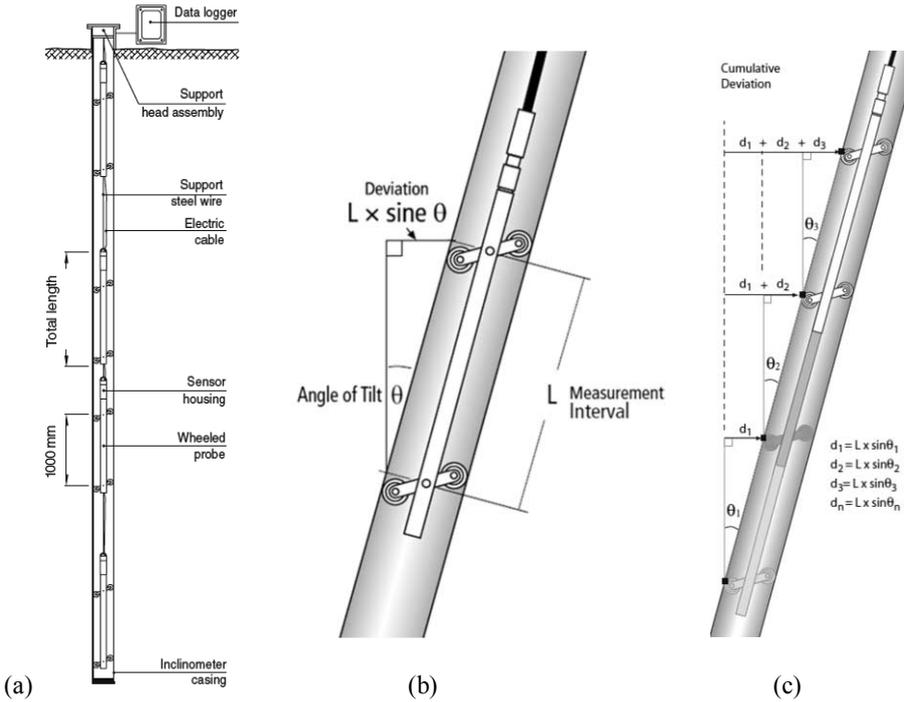
Figure 4.38 'In-place inclinometers' SISGEO (2009) (a) and Slopeindicator (2009) (b,c)
