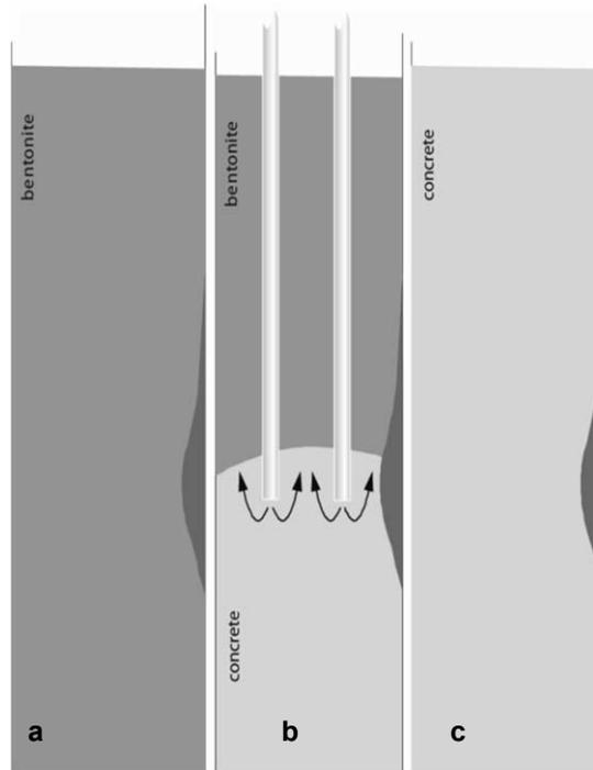
Figure 10.1 Forming of a bentonite inclusion during the concreting of a panel in three subsequent stages.
