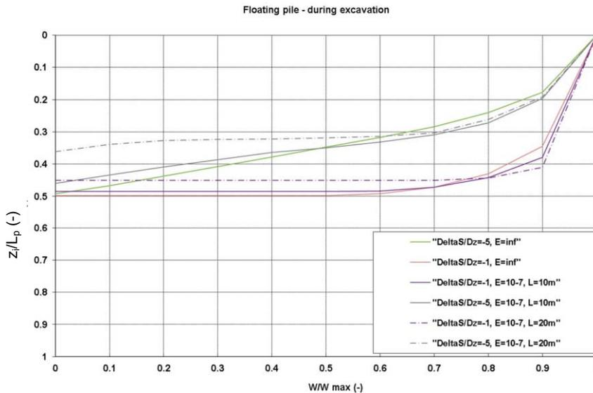
Figure 7.11 Results of  $z_i/L_p$  versus  $W/W_{max}$  with infinite and realistic stiffness for timber piles (10 m long and 20m long, D=0.2m)
