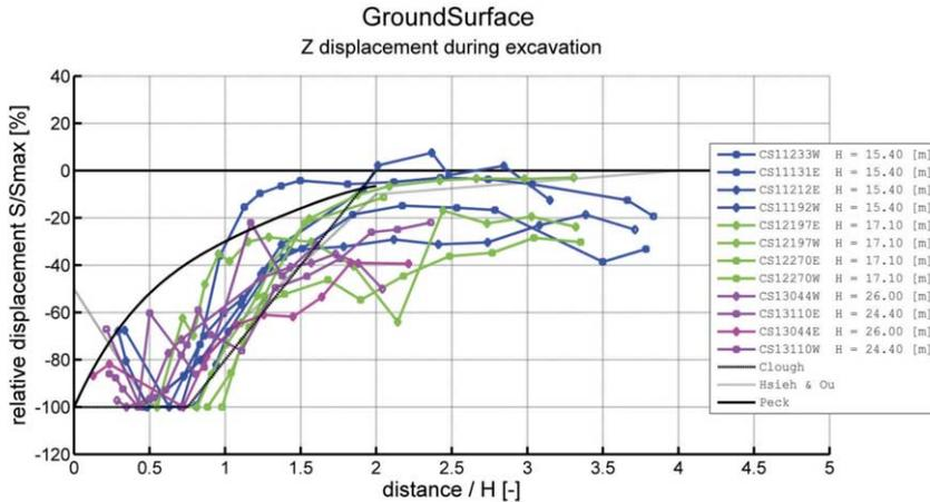
Figure 5.8 Measured surface displacements normalized with excavation depth  $H$  for three Amsterdam deep stations at the deepest excavation level available, compared to settlement envelopes proposed by Peck (1969), Clough and O'Rourke (1990) and Hsieh and Ou (1998).
