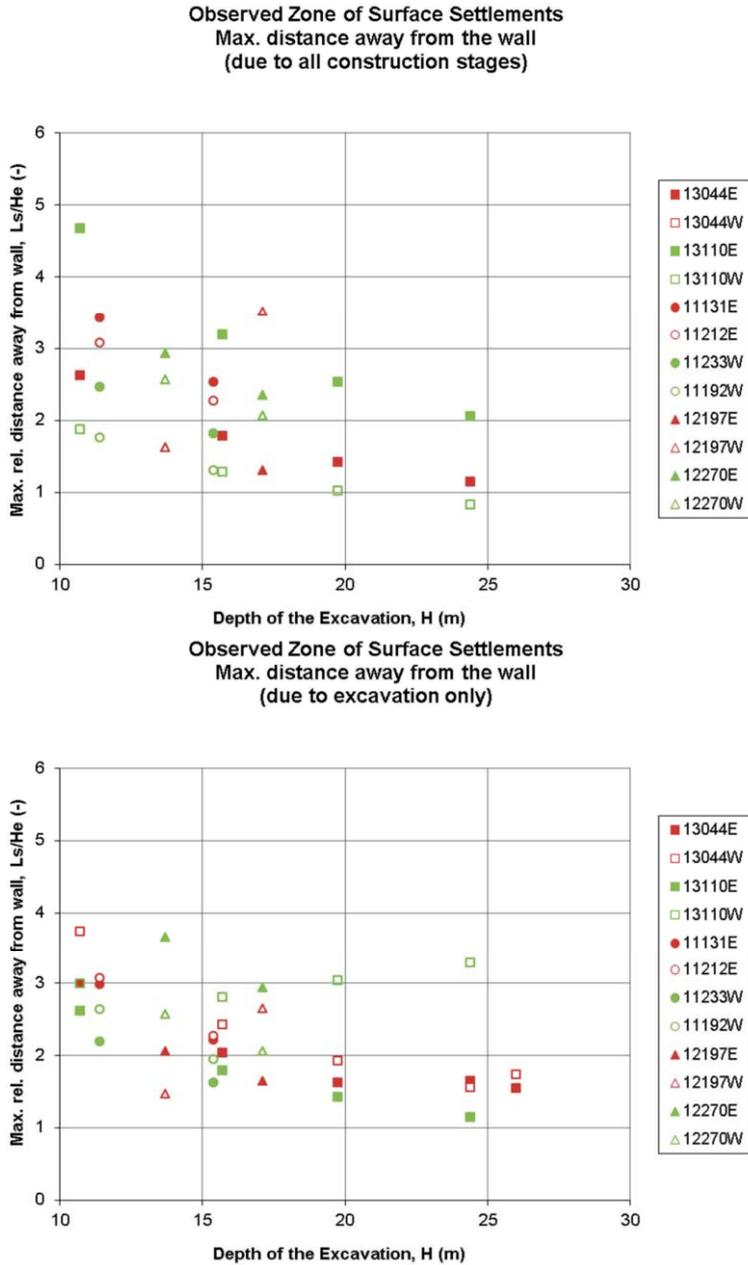
Figure 5.10 Maximum distance away from the wall (normalized with the excavation depth) to which the displacement is found in Amsterdam including preliminary activities (top) and for excavation only (bottom).
