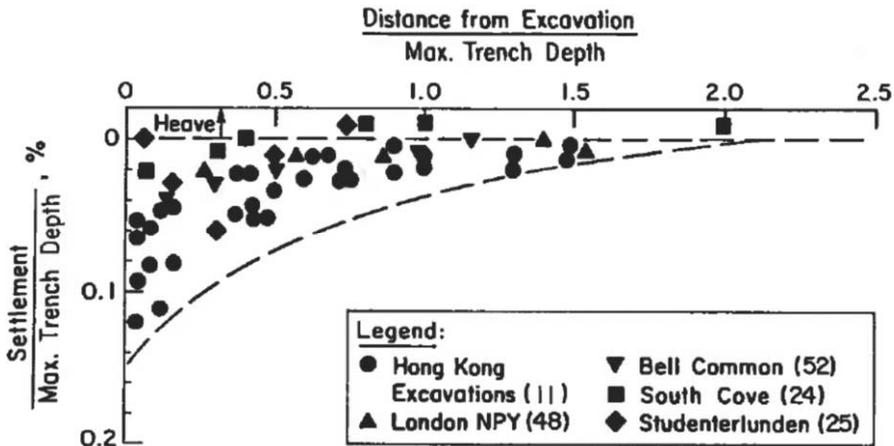
Figure 2.13 Settlement due to installation of a diaphragm wall (Clough and O'Rourke, 1990)
