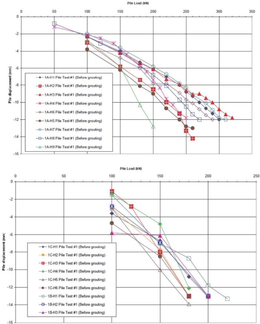
Figure 6.16 Pile load tests from Van der Stoel (2001)
