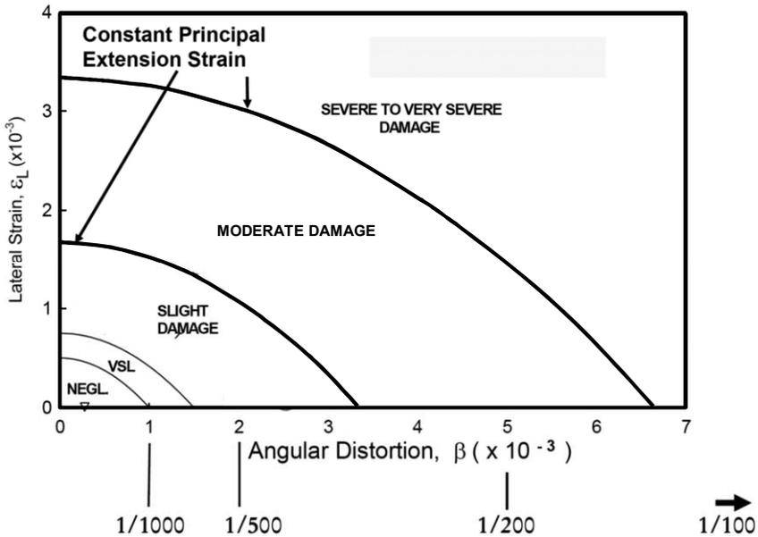
Figure 2.19 Relationship between angular distortion and horizontal strain (Cording et al. 2010)
