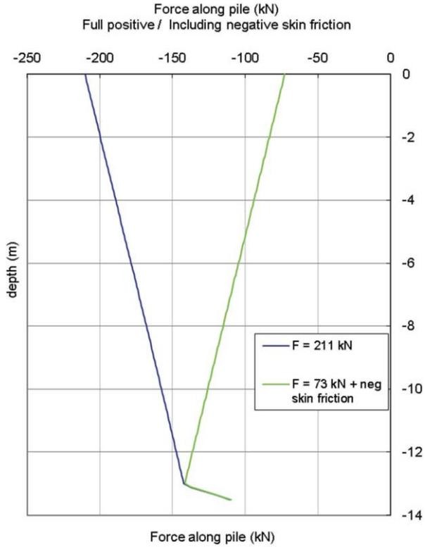
Figure 6.20 Actual timber pile with (blue) all layers positive friction and (green) negative skin friction to NAP -13m, base capacity 106 kN
