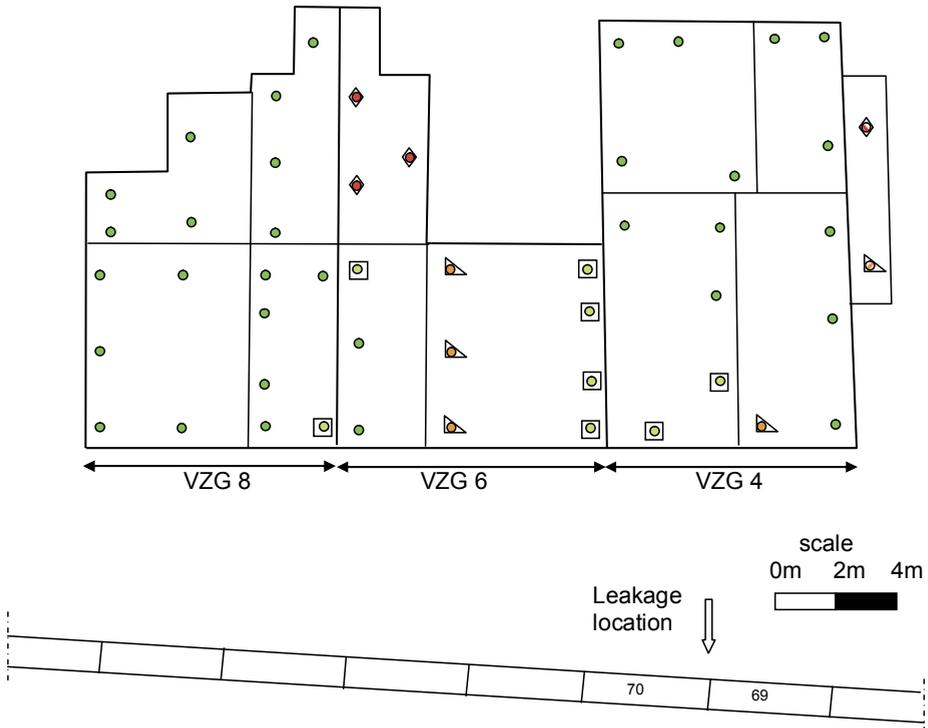
Figure 10.16 Schematic plan of Vijzelgracht 8, 6 and 4 with location of leakage and results of pile load tests ( ● piles test result = 400kN; ◻ piles test result 350-400 kN; ▽ piles test result 300-350 kN; ◆ piles test result <300 kN)
