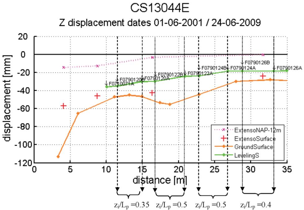
Figure 8.2 Ground and building displacements for Govert Flinckstraat (Ceintuurbaan), showing interaction levels ( $z_i/L_p$ ) derived from measurements
