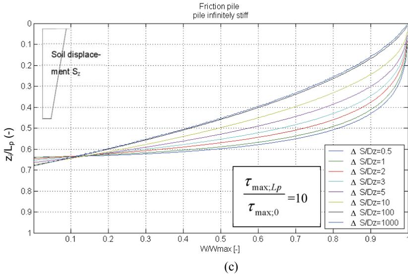
Figure 7.9 Interaction factor  $z_i/L_p$  for friction piles as a function of the initial pile load  $W/W_{max}$  for different values of  $\Delta S/D_z$  and increasing maximum shaft friction with depth
