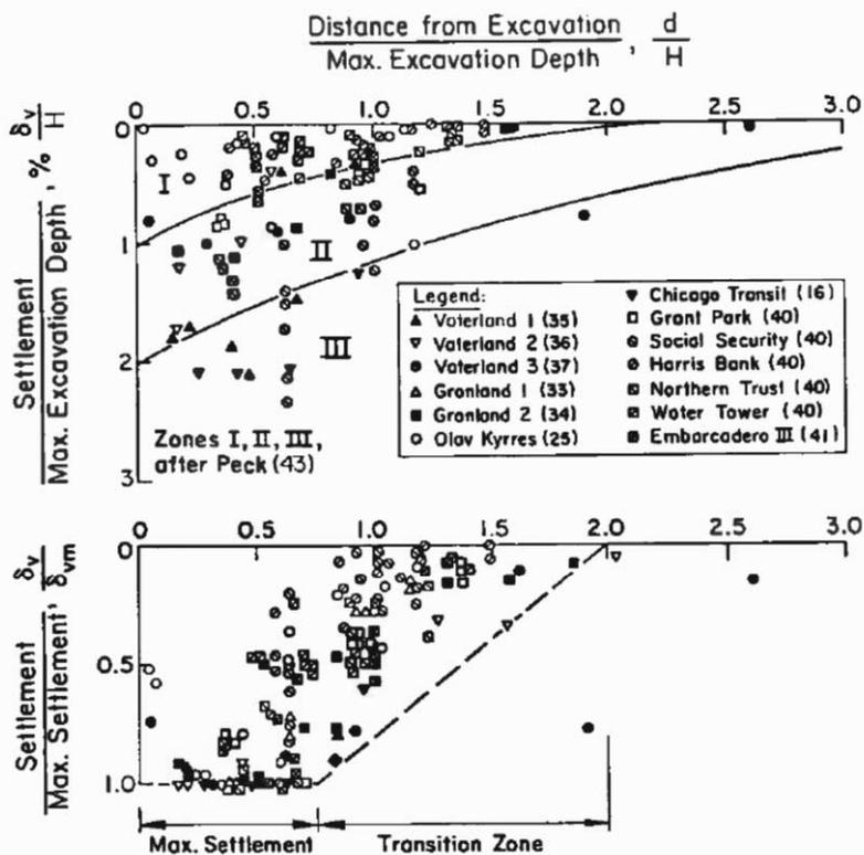
Figure 2.6 Measured settlements adjacent to excavations in soft to medium clay (Clough and O'Rourke, 1990)
