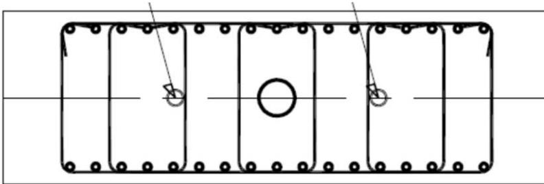
Figure 4.40 Position of inclinometer tubes in diaphragm wall panel
