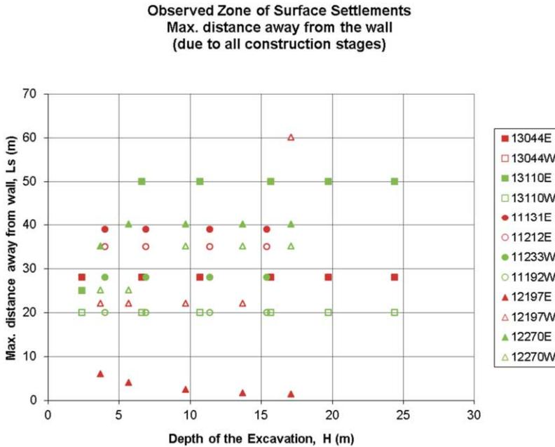
Figure 5.9 Maximum distance away from the wall to which the displacement is found in Amsterdam deep excavation, data from all construction stages.
