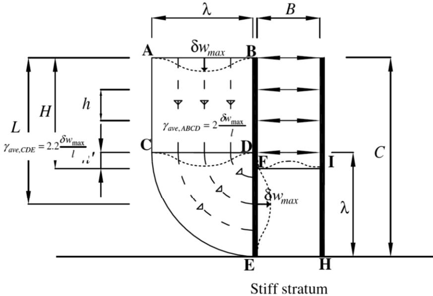
Figure 2.11 Incremental displacement field for narrow excavations (Bolton et al., 2008)
