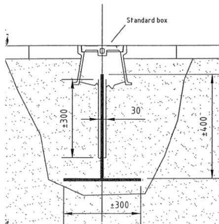
Figure 4.34 Borneo FENO settlement point (example, actual depth 800 mm instead of 400 mm)
