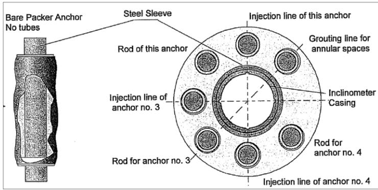
Figure 4.36 Combined inclino- and extensometer cross section (source Boart Longyear<sup>®</sup>, Interfels)
