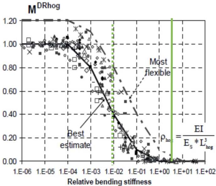
Figure 3.17 Design curves from Goh (2010) for hogging, modified modification factors with result for White House in green lines (solid for walls, dashed for slab and floors)
