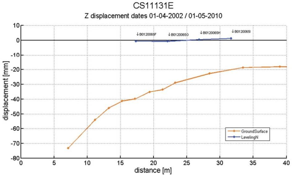
Figure 8.19 Building displacement of Rokin 65 compared to the surface settlement with distance from the deep excavation.
