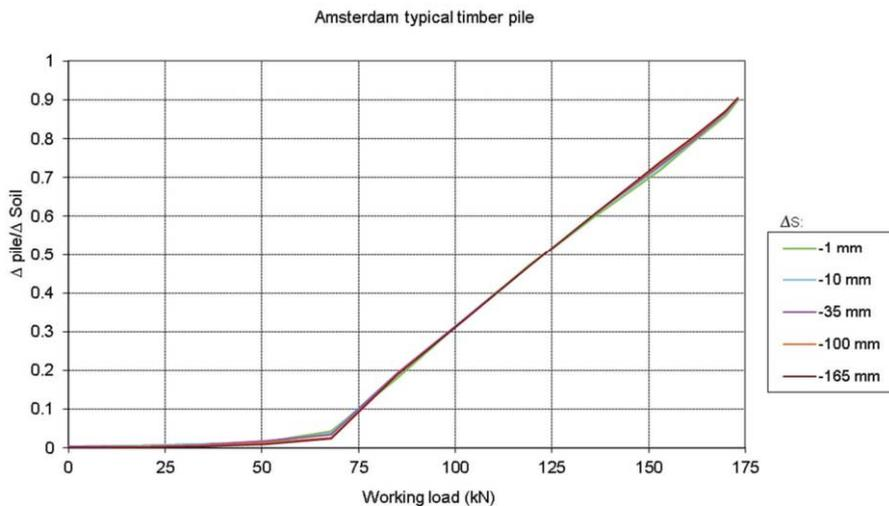
Figure 7.15 Results pile displacement over maximum soil settlement for actual soil profile in Amsterdam, assuming initial negative skin friction present
