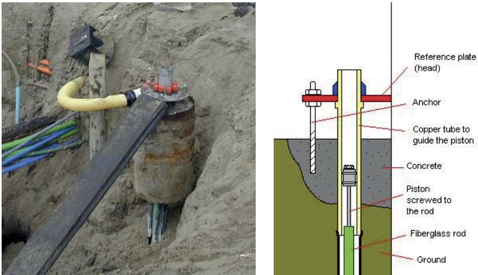
Figure 4.35 Extensometer (left) and illustration of measurement system (right)
