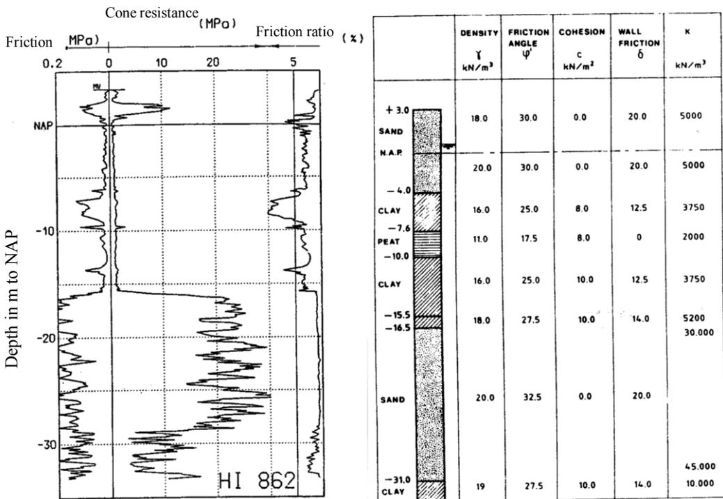
Figure 3.9 Typical CPT near White House and soil parameters used for design (Brassinga and van Tol, 1991)
