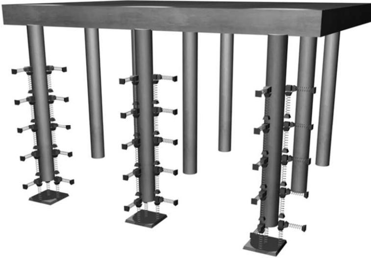
Figure 7.3 Cap interaction model D-PileGroup, modified from Bijmagne and Luger (2010)
