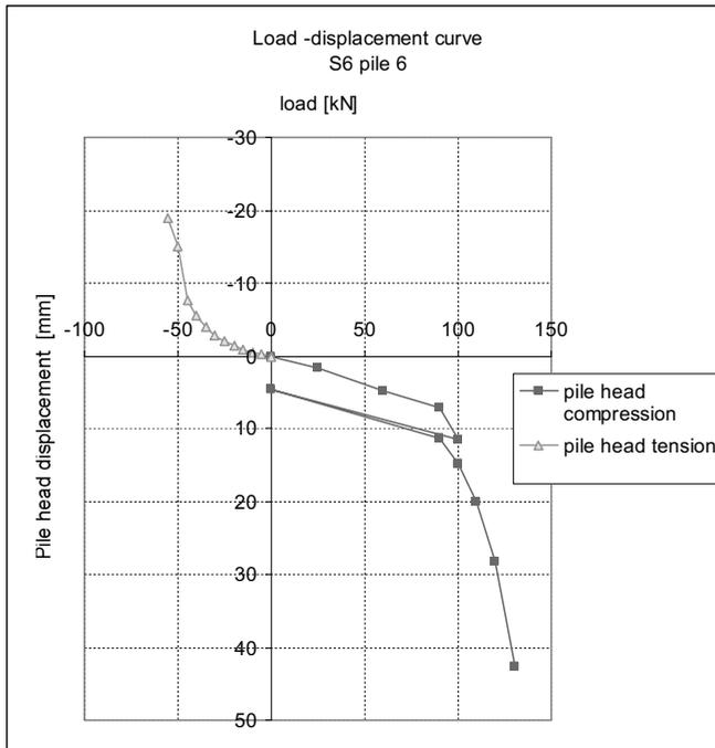
Figure D.3 Pile load test results old piles 2, 3, 4, 5 and 6
