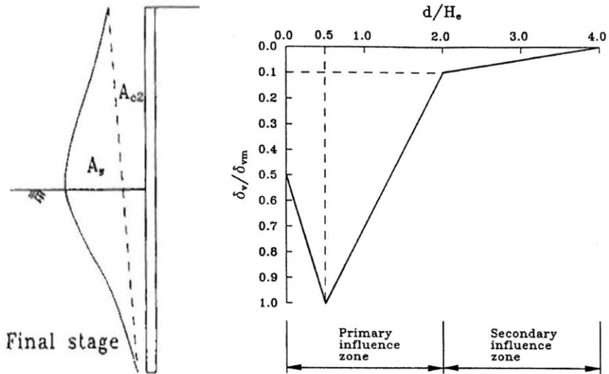
Figure 2.10 Shape of settlement trough by Hsieh and Ou (1998) for deep inward wall deflection
