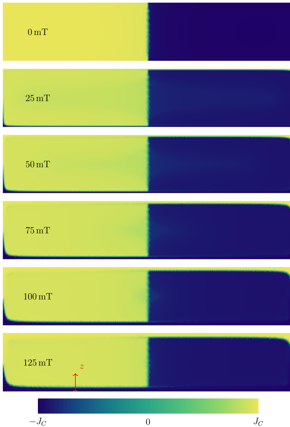
Fig. 4.13 The current density distribution after 10 cycles of crossed-field with varying amplitudes at 8 Hz. The arrow in red corresponds to the z -axis in Figure 4.14 (a).
