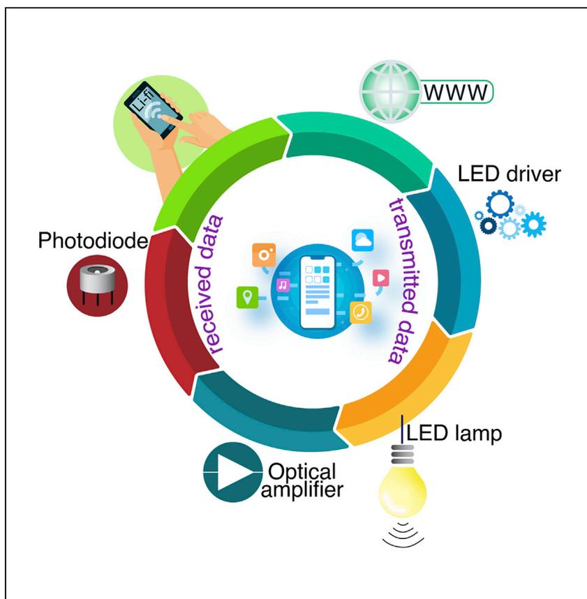
Challenges in visible-light communication (VLC) include mitigation of signal attenuation and fading control. Here, Bastos et al. present a compact and flexible optical fiber amplifier for advanced VLCs and improve the communication reliability demonstrated for pre-amplifier and relay node scenarios and simulated in a realistic environment.
