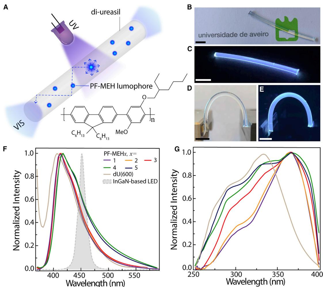
**Figure 2. Optical Properties of PF-MEH-Di-Ureasil Cylindrical Fibers**
