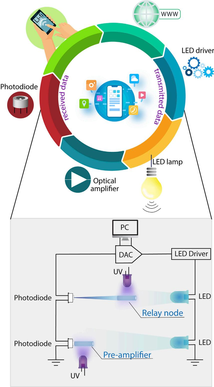
**Figure 1. Scheme of the VLC System**
