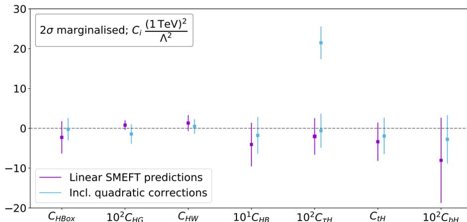
**Figure 21.** Marginalised 95 % credible intervals for each of the indicated operator coefficients resulting from a fit to Higgs signal strength data using nested sampling. We compare the effects of including quadratic contributions from dimension-6 operators (blue) to the case of linearised SMEFT predictions (purple).
