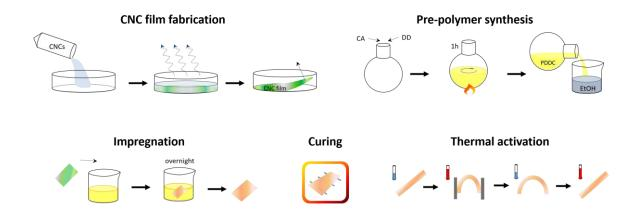
**Figure S1.** Fabrication procedure for the CNC/PDDC-HD hybrid structure and thermal activation steps.
