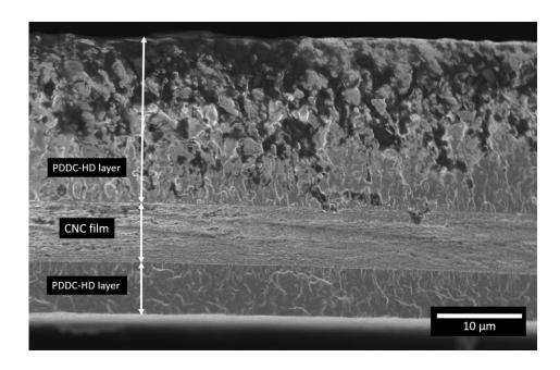
**Figure S2.** SEM image showing the layered structure of the CNC/PDDC-HD hybrid material. The CNC thin film is sandwiched between two layers of PDDC-HD as a result of the impregnation process.
