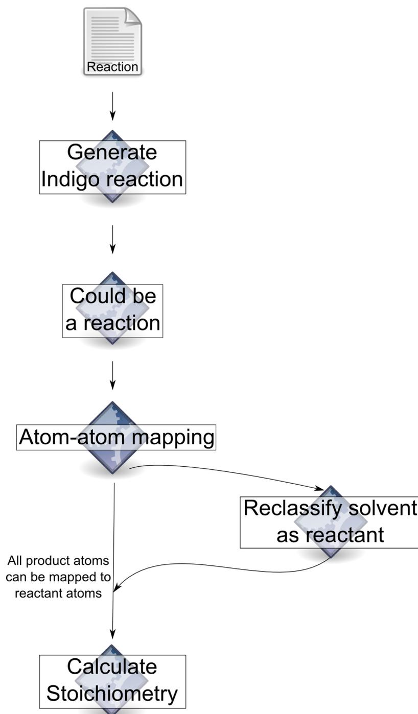
**Figure 4-10** Schematic of processes employed in converting putative reactions to atom-mapped reactions
