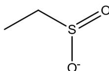
**Figure 3-125** Due to resonance this structure is achiral
