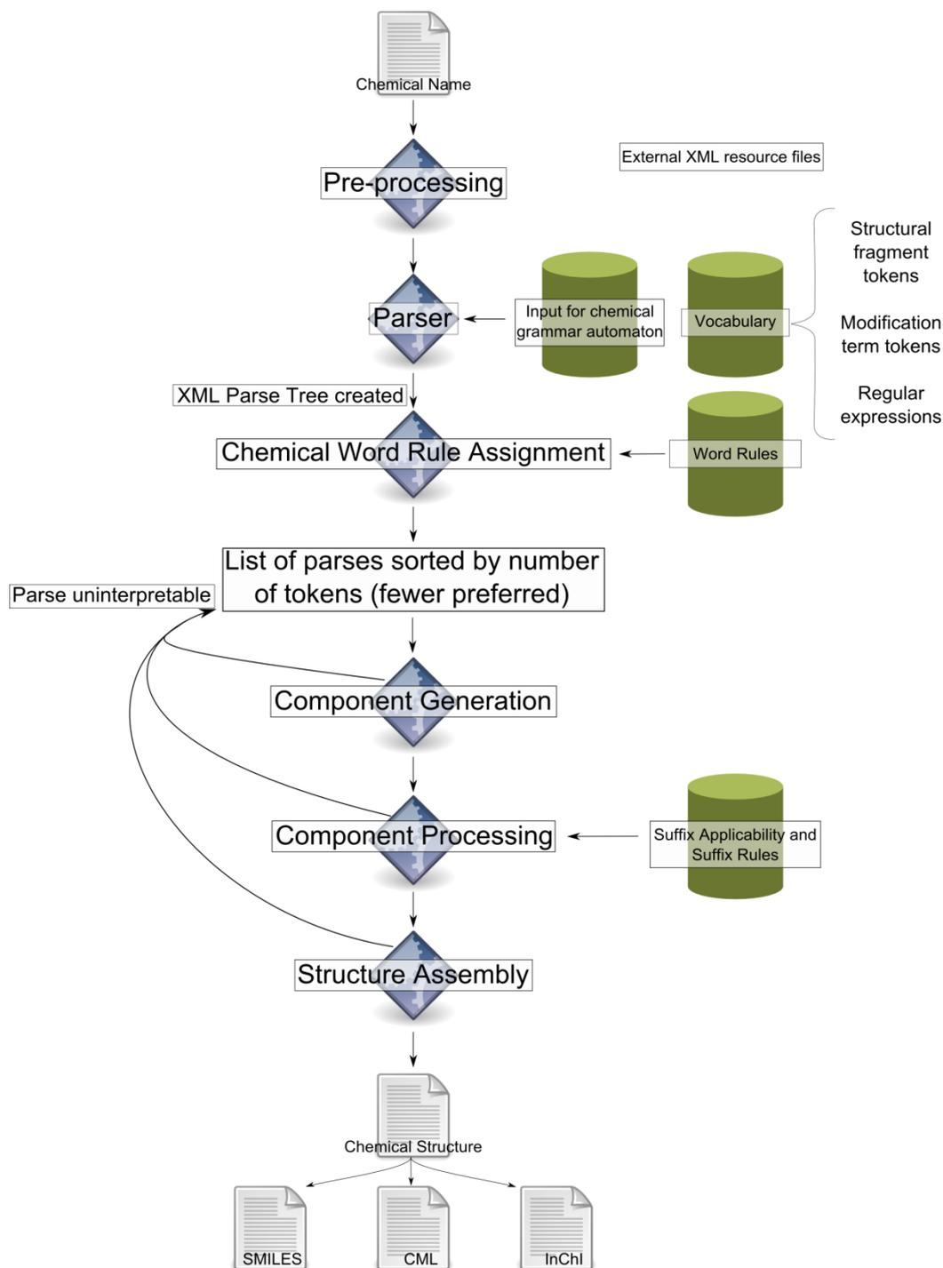
**Figure 3-5** Components of OPSIN's architecture, showing the process from chemical name through to a structure
