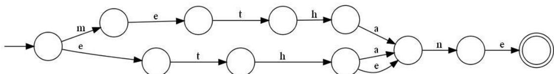
**Figure 2-10** A finite state automaton that matches “methane”, “ethane” and “ethene”
