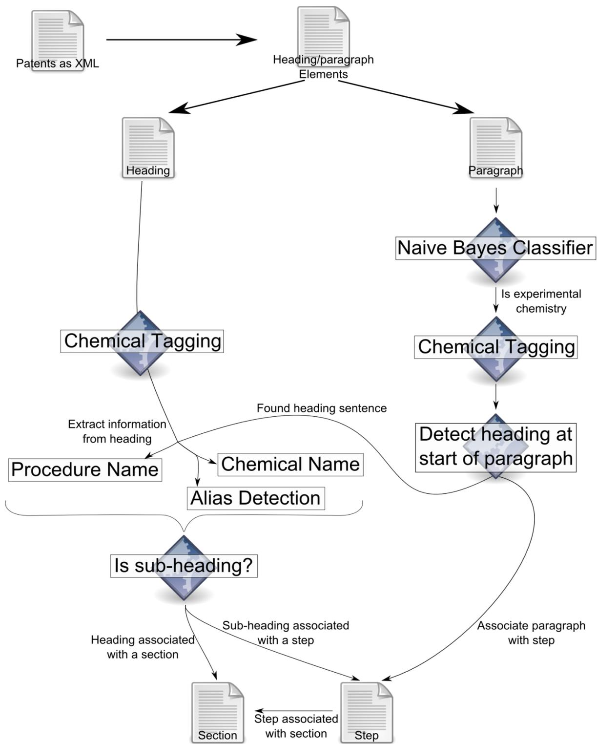
**Figure 4-2** Schematic of processes employed in the segmentation of a document in steps, step headings and section headings
