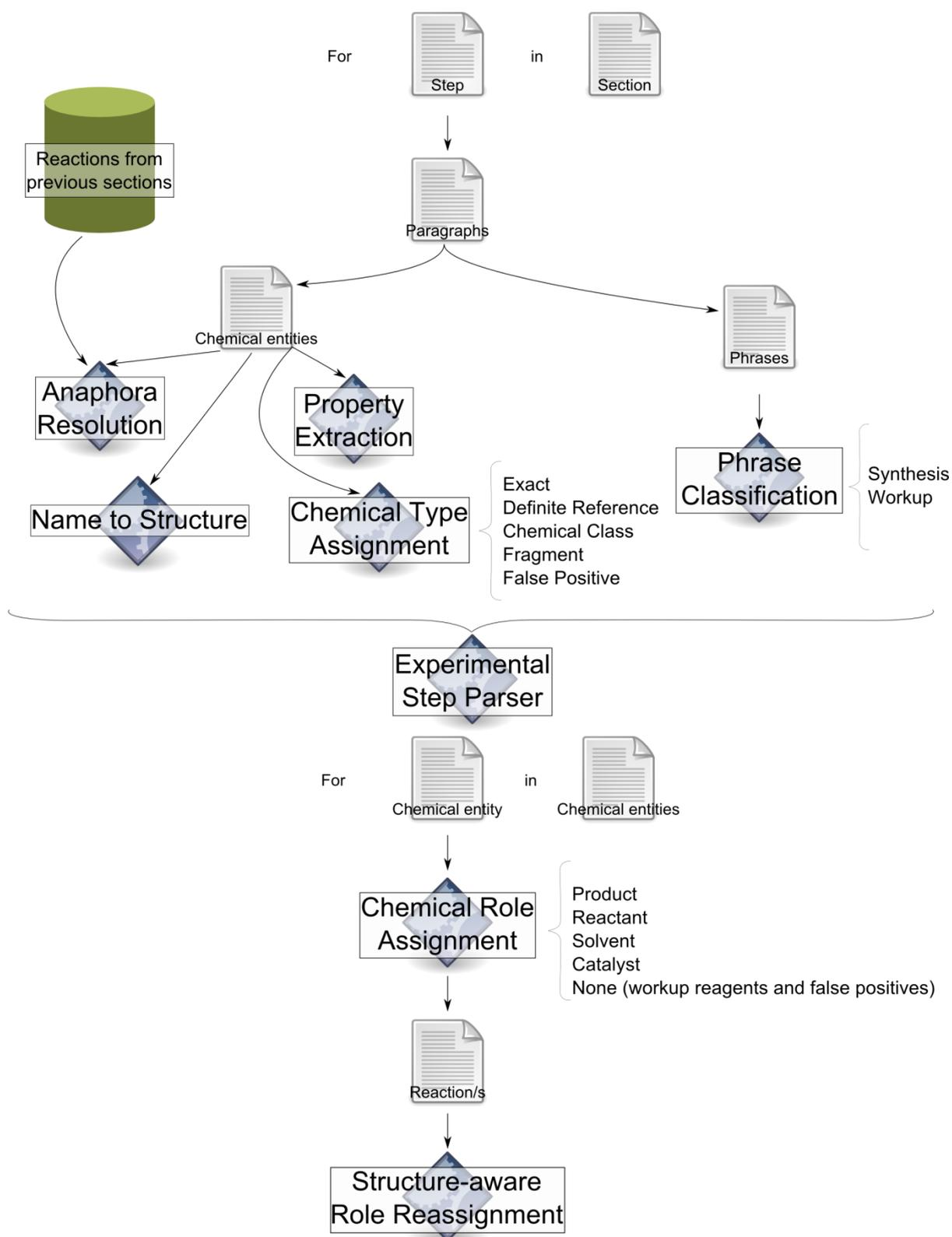
**Figure 4-5** Schematic of processes employed to extract from reactions from an experimental chemistry section.
