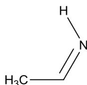
**Figure 3-141** (Z)-ethanimine: C(/C)=N/[H] Note that without mentioning the hydrogen it is not possible to express this stereochemistry
