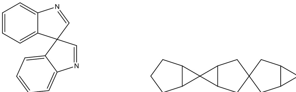
**Figure 3-95** Examples of spiro systems with repeated ring systems: 3,3'-spirobi[indole] (left) and 3,3':6',6''-dispiroter[bicyclo[3.1.0]hexane] (right)
