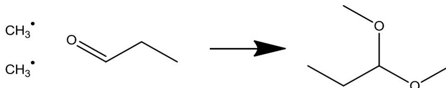
**Figure 3-113** propanal dimethyl acetal, constituent parts (left) and final structure (right)
