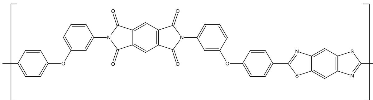
**Figure 3-114** poly[(benzo[1,2-d:4,5-d']bis[1,3]thiazole-2,6-diyl)-1,4-phenyleneoxy-1,3-phenylene(1,3,5,7-tetraoxo-1,2,3,5,6,7-hexahydrobenzo[1,2-c:4,5-c']dipyrrole-2,6-diyl)-1,3-phenyleneoxy-1,4-phenylene]
