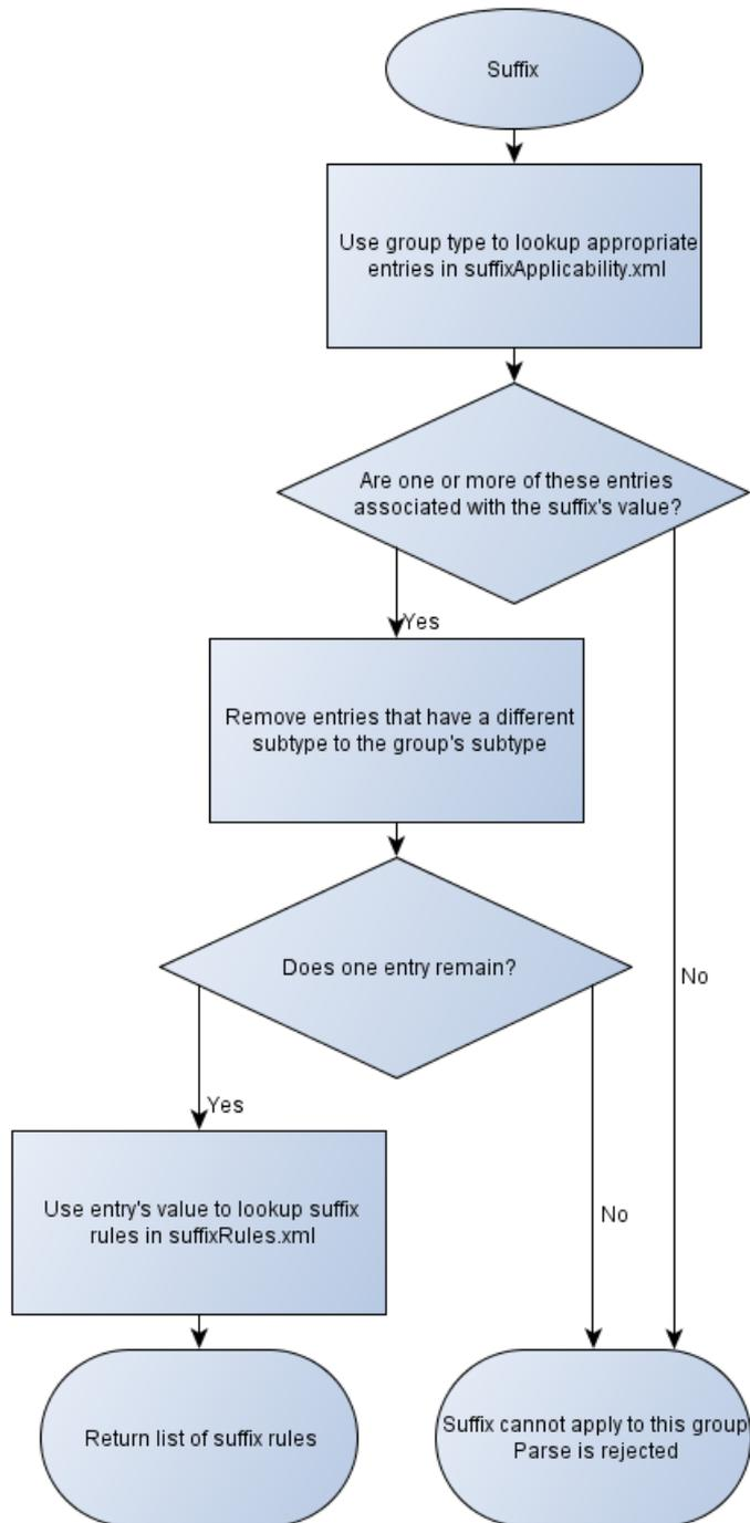
**Figure 3-50** Flowchart for handling suffixes. The group in question is the group to which the suffix will apply.
