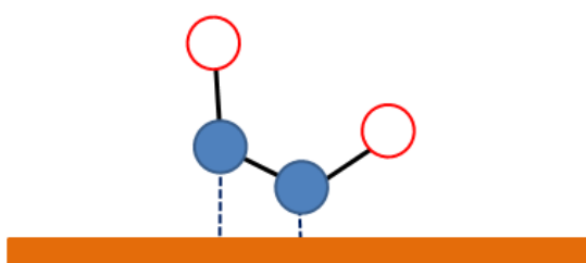
Fig. 4.29 Simple visual representation of the (\text{NO})_2 dimer having a tilt along the horizontal axis of the N-N bond.
