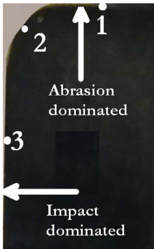
Fig. 13. The cross section sample 'B' shown in Fig. 13 of the impact-tumbler sample. Abrasion predominates in region '1', and impact damage in regions '3', with region '2' representing a transition area.
