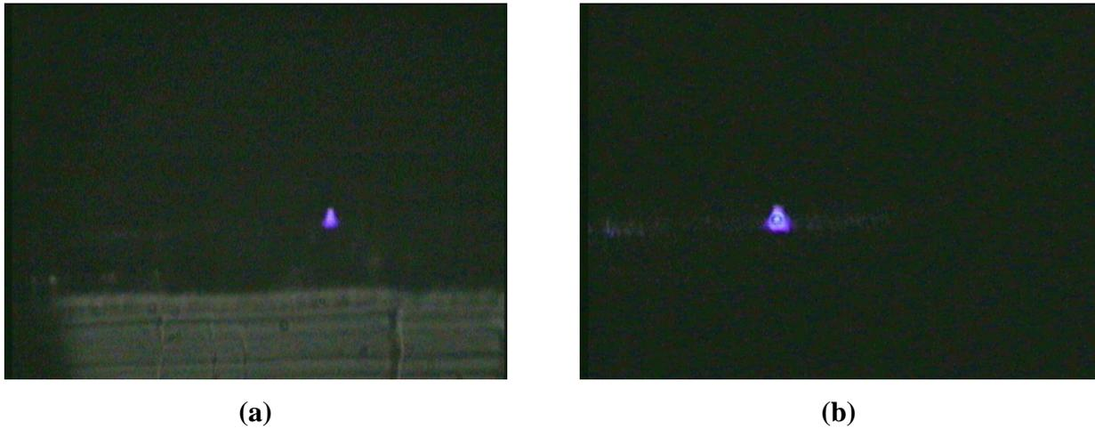
Figure 5.28 – Intensity field profile of (a) 2.5x3 and (b) 3x3  $\mu\text{m}$  siloxane ridge waveguide captured on a CCD camera at 50x magnification
