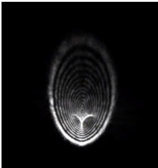
Figure 5.10. The tilted laser-beam shape.
