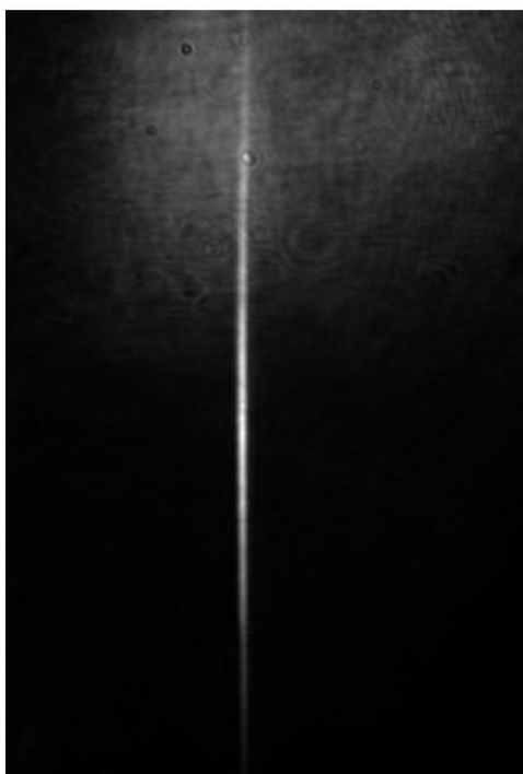
Figure 5.12. The image of Oxazine 725 excited by the light sheet
