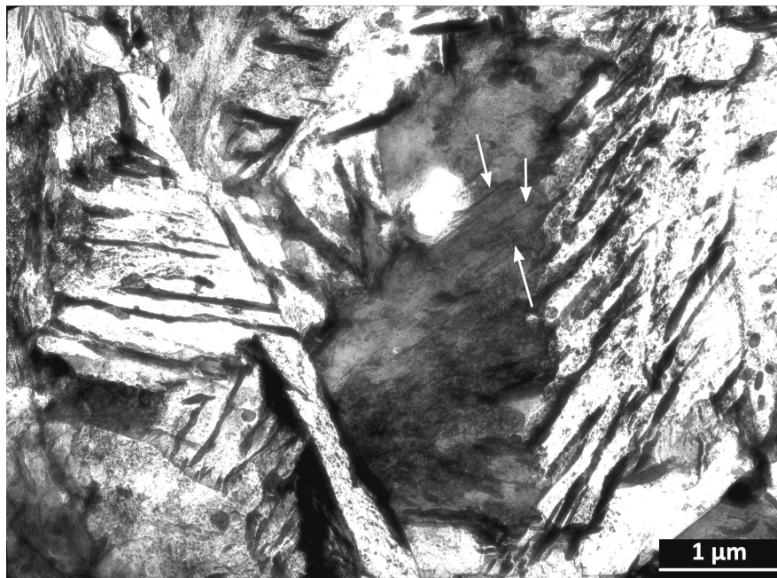
Figure 4.18: Transmission electron micrograph of Alloy A transformed at 300°C showing a region of martensite. Note the thin, faint twins.
