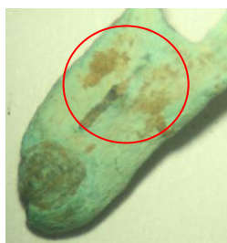
Figure 5a- Fragment 2: cuprite layer exposed along the mid rib (circled red)
