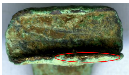
Figure 5b – Fragment 2: exposed metal (circled red)
