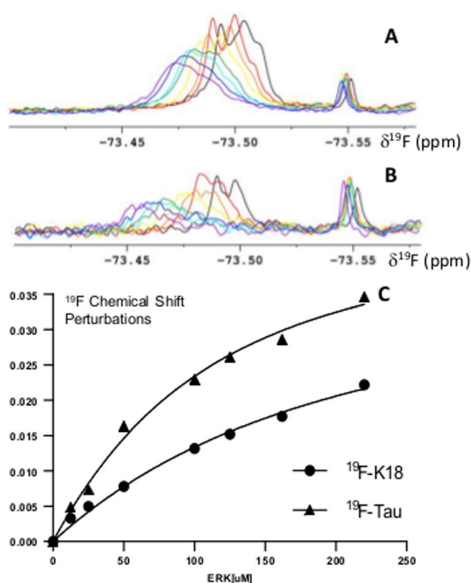
**FIGURE 7. Determination of  $K_D$  of Tau/ERK2 interaction.** Shown are superimposed one-dimensional Fluor NMR spectra of CF3-Tau-(244–372) (*A*) and CF3-Tau (*B*). *C*, saturation curves based on the chemical shift perturbation of the Fluor signal of CF3-Tau and CF3-Tau-(244–372). The signal of only one CF3-Cys was monitored along the titration, the second one being broadened.
