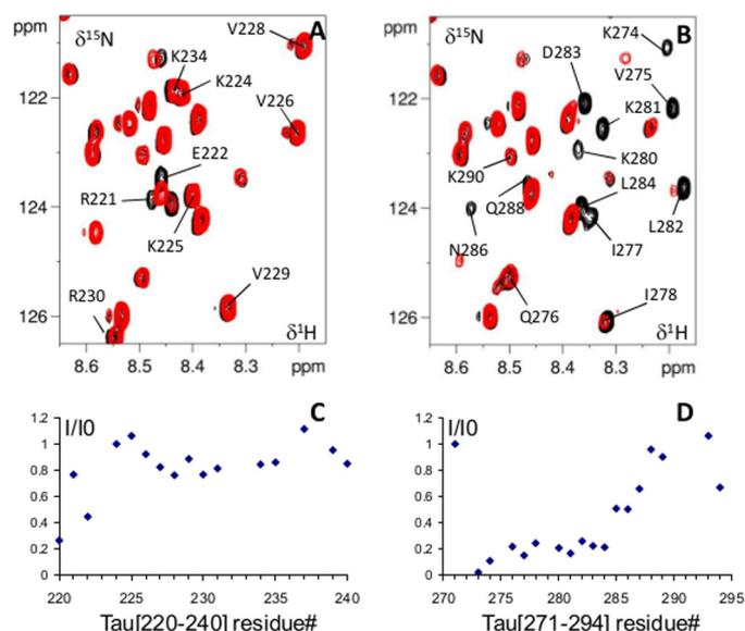
**FIGURE 8. Interaction of Tau peptides with ERK2.** *A* and *B*, detail of overlaid  $^1\text{H}$ ,  $^{15}\text{N}$  HSQC two-dimensional spectra of  $^{15}\text{N}$ -His-SUMO Tau-(220–240) (*A*) and  $^{15}\text{N}$ -His-SUMO Tau-(271–294) (*B*) free in solution (in black) or with 1 molar excess of ERK2 (superimposed in red). Relative intensities ratio  $I/I_0$  for corresponding resonances in these spectra are shown in *C* and *D*, respectively.
