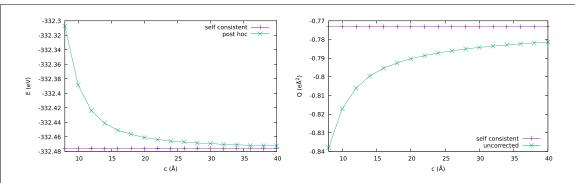
**Figure 3.** The energy (left) and quadrupole moment (right) from a single layer of graphene with a charge of +2e per unit cell (two atoms) as the cell length (vacuum separation) is varied. For the energy a *post hoc* correction is shown as well as a self-consistent correction. For the quadrupole, no *post hoc* correction was applied.
