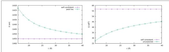
**Figure 5.** The energy (left) and quadrupole moment (right) computed for four layers of graphene with a charge of +2e per unit cell (eight atoms) as the cell length (vacuum separation) is varied. For the energy a *post hoc* correction is shown as well as a self-consistent correction. For the quadrupole, no *post hoc* correction was applied.
