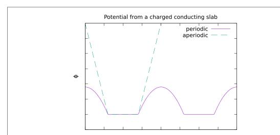
**Figure 2.** The potential arising from a uniformly charged conducting slab with and without periodic boundary conditions. The thickness of the slab is 40% of the periodic repeat distance in the direction normal to the slab.
