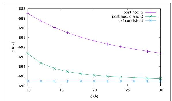
**Figure 6.** The energy from two layers of SiC with a charge of +2e per unit cell (four atoms) as the cell length (vacuum separation) is varied. A simple *post hoc* correction depending just on the charge is shown, a *post hoc* correction including the quadrupole moment, and a self-consistent correction. The self-consistent line shows noise, and the variation between its greatest and least value is less than 0.5 meV.
