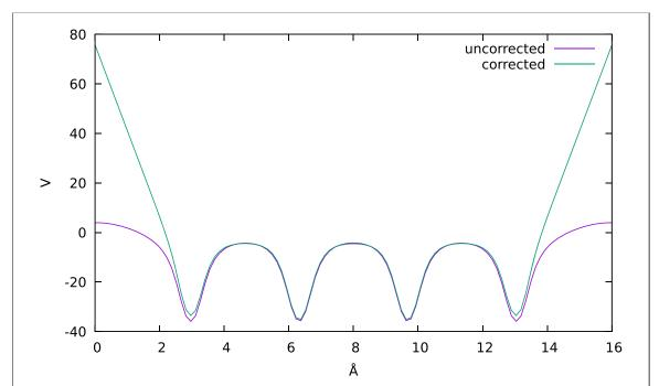
**Figure 4.** The potential arising from four layers of graphene, with a charge of +2e per unit cell (eight atoms). A standard uncorrected DFT calculation is shown, along with the potential after the correction discussed in this paper. The uncorrected potential has been shifted to align the two potentials in the centre of the slab.
