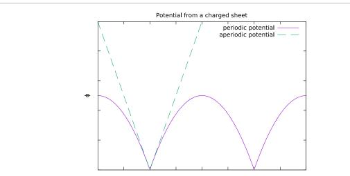
**Figure 1.** The potential arising from a uniformly charged sheet with and without periodic boundary conditions. Two repeat units are show in the periodic case.
