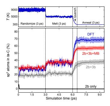
FIG. 7. Top: Exemplary temperature profile during a DFT-MD melt-quench simulation to yield a 216-atom structure of ta-C. Bottom: Concentration of  $sp^3$  atoms during these cycles, measured by counting atomic neighbors up to a cutoff distance of 1.85 Å. DFT benchmarks are compared to GAP results using different combinations of descriptors; areas of light shading indicate standard deviations.
