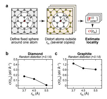
FIG. 3. (a) Schematic overview of the procedure used here for locality tests. (b,c) Results for diamond and graphite, respectively, obtained by displacing all atoms outside  $r_{\rm fix}$  randomly and inspecting the standard deviation of the force on the central atom.
