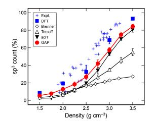
FIG. 10. Count of "sp<sup>3</sup>" (fourfold coordinated) carbon atoms in quenched *a*-C structures as a function of density. Ten independent melt-quench cycles were performed at each density for the empirical and GAP models; three independent ones were done for DFT. Data for the Brenner potential are taken from Ref. 15. Experimental data have been collected from Refs. 77–79. Error bars represent standard deviations. Lines between data points are only guides to the eye.
