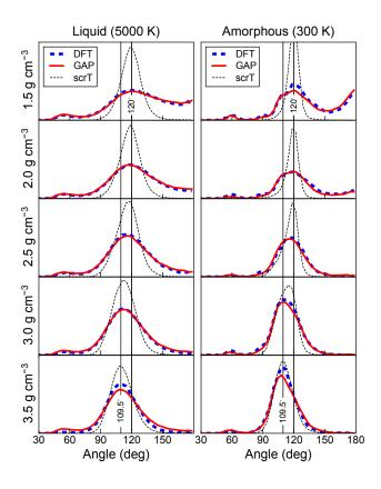
FIG. 9. As Fig. 8, but for angular distribution functions. Thin vertical lines mark angles of  $109.5^{\circ}$  and  $120^{\circ}$ , corresponding to ideal sp<sup>3</sup> (diamond-like) and sp<sup>2</sup> (graphite-like) motifs, respectively. The scaling of the vertical axes is arbitrary.
