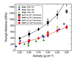
FIG. 13. Young's modulus of *a*-C as a function of density. Experimental values are taken from Ref. 81 (green), Ref. 82 (blue), and Ref. 83 (yellow), respectively. Lines between data points are guides to the eye.
