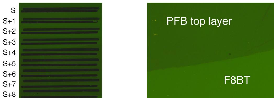
(a) Aligned F8BT film with Au/Al electrodes (line width=1.5mm).
