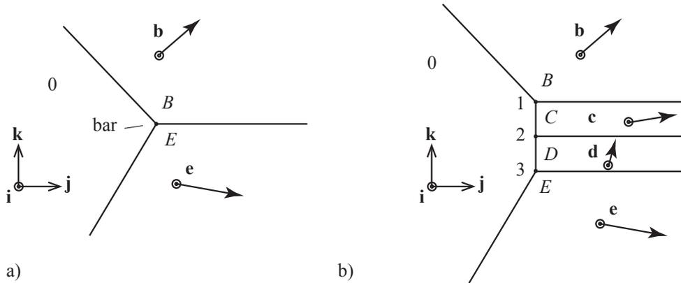
Figure 4: a) A section through a bar that is the common edge of three cells. b) Thickening the face BE to consist of two thin prismatic cells C and D over which a general stress function may be applied.
