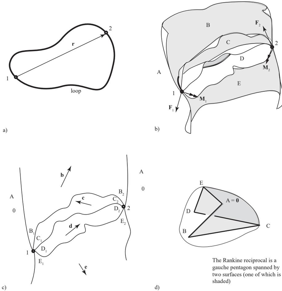
Figure 6: a) A general loop. b) A section giving two cut ends 1 and 2. c) A general stress function over 5 cells for which the loop is a common boundary. d) The Rankine reciprocal is a gauche pentagon.
