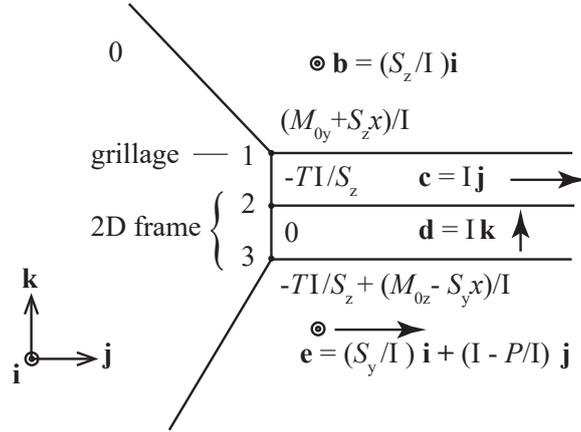
Figure 5: A stress function that creates a general stress resultant in the bar. The stress function consists of a grillage system and a 2D frame system.
