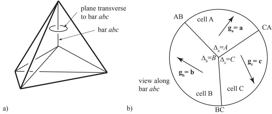
Figure 2: A plane transverse to bar  $abc$  which is the common edge of cells A, B and C. b) The stress function definition on that plane. Note in particular that the gradient vectors need not lie in that plane.
