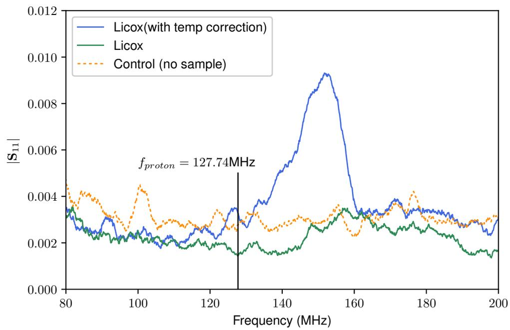
Figure 2: Modulus of the complex reflection coefficient  $S_{11}$  as a function of frequency. The proton Larmor frequency for 3T is indicated by the vertical line.
