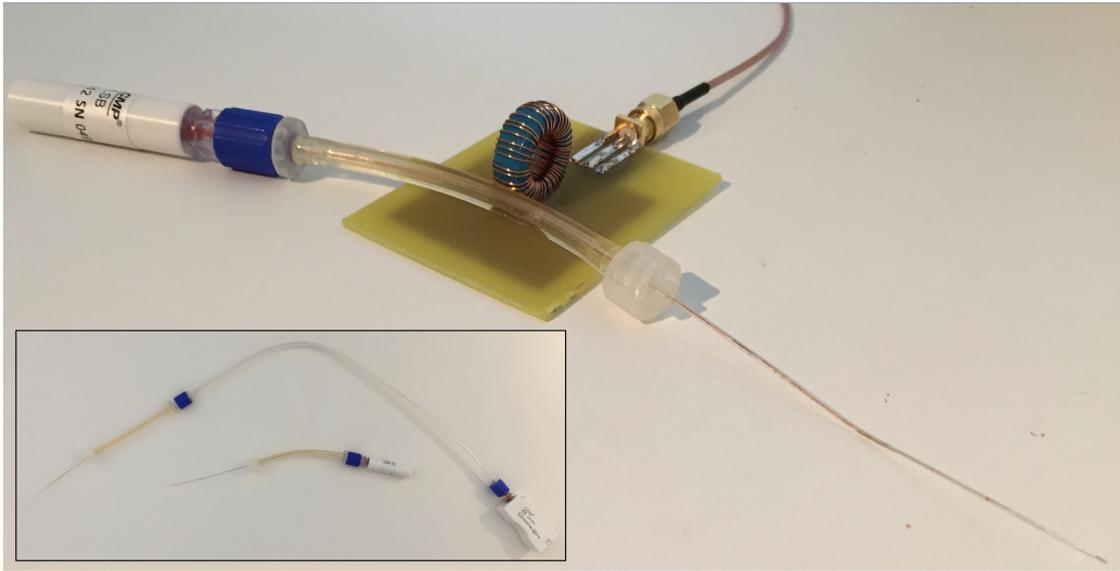
Figure 1: Experimental apparatus. The inductor is constructed from a ferrite toroid wound with approximately 40 turns of 30SWG enameled copper wire. Coupling to the probe was achieved through proximity. Pictured is a Model CC1SB  $P_{bt}O_2$  probe without integrated temperature sensing. The inset shows the CC1SB (lower device) and CC1P1 next to each other. The difference in lengths is apparent.
