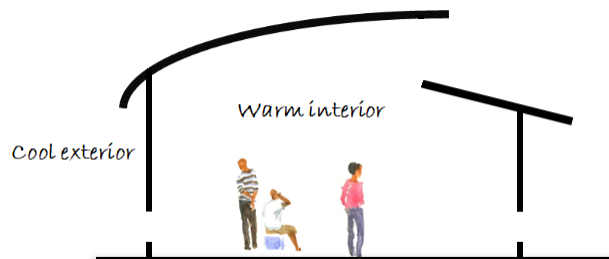
FIGURE 2: Sketch of a building in elevation showing a large upper vent.
