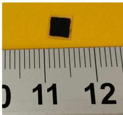
**Figure 4-30.** The transparent AH pellet with carbon paste on the surface as electrodes. This electrode sample was then subjected to electric measurements.
