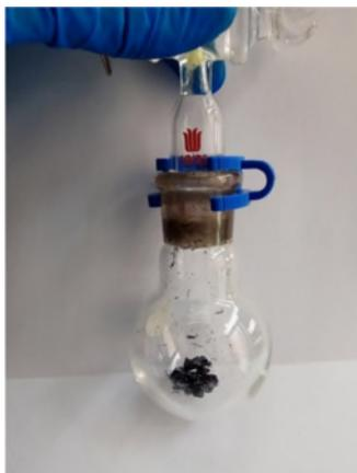
**Figure. 1** Collection of products in Schlenk Flask under inert gas protection, due to the phosphorene is easily to be oxidized in air.
