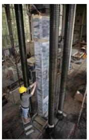
Figure 6 Column strengthening
