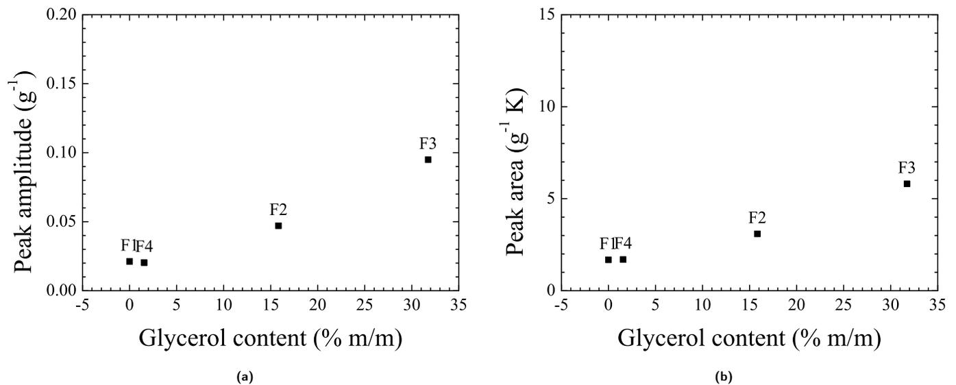
**Fig. 3** (a) The amplitude and (b) area of the fitted mean ( $n = 2$ )  $\tan \delta$   $\beta$ -transition peak based on DMA as a function of the glycerol content of formulations F1, F2, F3 and F4, respectively. Values were determined on  $t_0$  samples stored at 278 K.
