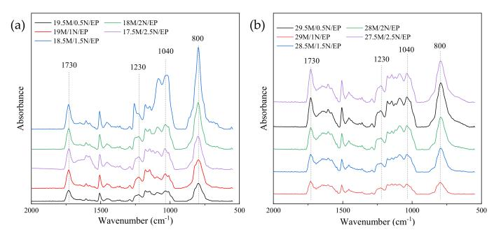
**Figure 19.** Partial enlarged view of baseline correction of the micro/nano SiC/EP infrared spectra. (**a**) 20 wt% SiC/EP; (**b**) 30 wt% SiC/EP.
