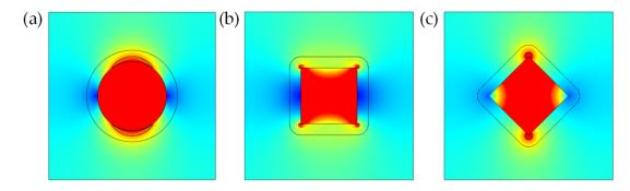
**Figure 13.** Cloud iamge of conductive heat flux after ImageJ processing. (a) Filler particle is small sphere; (b) Filler particle is horizontally placed cube; (c) Filler particle cube is rotated 45°.
