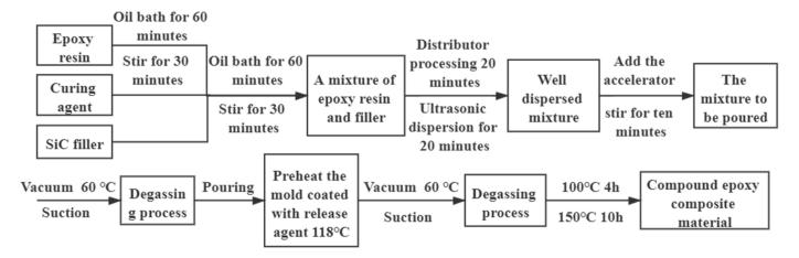
Figure 1. Epoxy composite preparation process.
