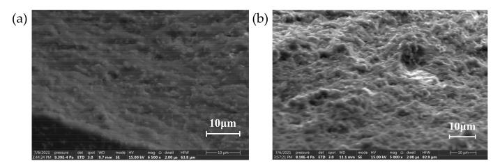
Figure 20. The cross-sectional microscopic electron microscope image of the micro-nano composite system. (a) 29.5% m-SiC/0.5%n-SiC/EP; (b) 27.5% m-SiC/2.5%n-SiC/EP.
