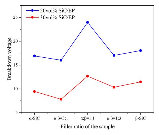
Figure 5. Average breakdown strength of composite material.
