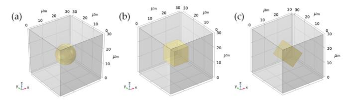
**Figure 11.** The geometric model of a composite material filled with a single particle. (**a**) A single spherical particle; (**b**) A single cubic particle placed horizontally; (**c**) A single cubic particle rotated  $45^{\circ}$ .
