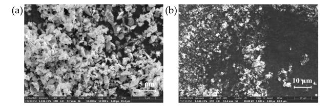
Figure 3. Electron microscopy of micron and nanometer SiC particles. (a) 1.5 μm β-SiC; (b) 50 nm β-SiC.
