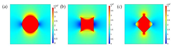
Taking the cross section parallel to the *xz* plane and  $y = 15 \mu m$  to study the conductive heat flux of the filler and its surrounding matrix, as shown in Figure 12:
