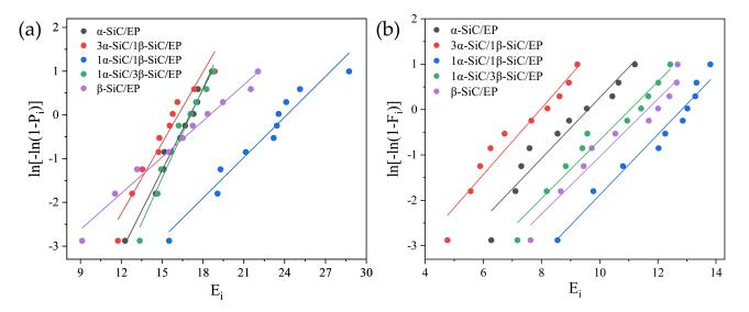
Figure 4. Weibull distribution of composite material breakdown strength. (a) 20 vol% SiC/EP; (b) 30 vol% SiC/EP.
