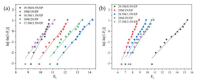
**Figure 16.** Weibull distribution of micro-nano composite SiC/EP breakdown strength. (**a**) 20 wt% SiC/EP; (**b**) 30 wt% SiC/EP.
