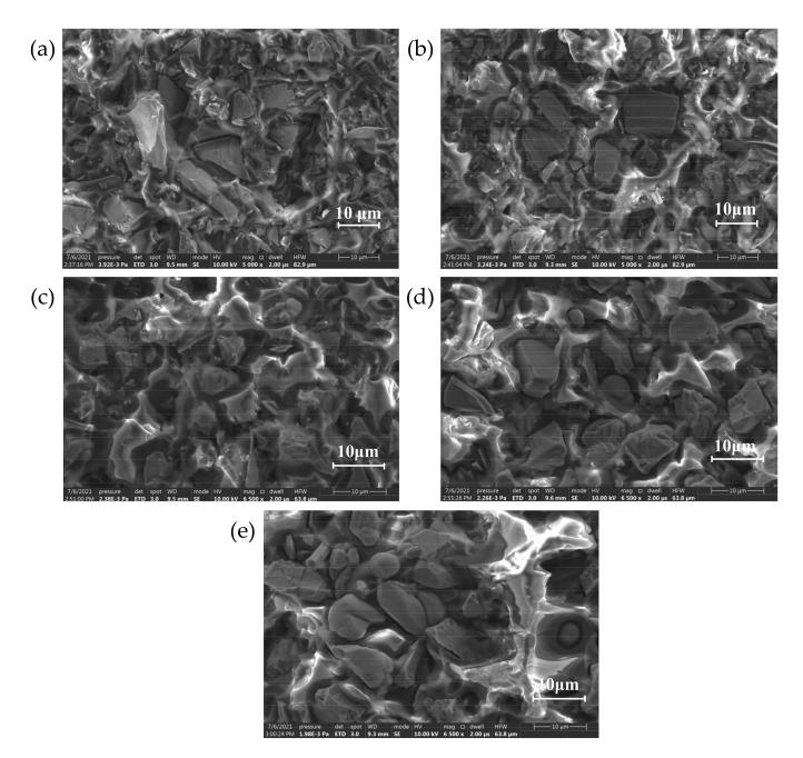
**Figure 8.** Sectional electron micrograph of SiC/EP composite material. (a)  $\alpha$ -SiC/EP; (b)  $\alpha$ -SiC: $\beta$ -SiC = 3:1; (c)  $\alpha$ -SiC: $\beta$ -SiC = 1:1; (d)  $\alpha$ -SiC: $\beta$ -SiC = 1:3; (e)  $\beta$ -SiC/EP.
