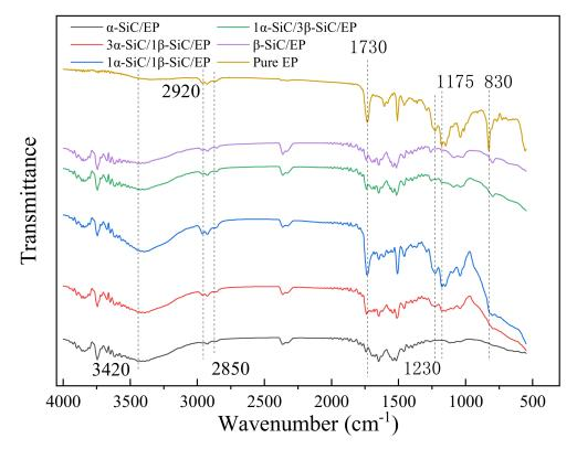
Figure 6. Infrared spectrum of SiC/EP composite material.
