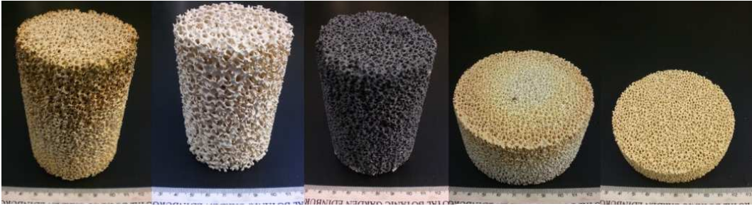
Figure 2.4: Porous foams used for the reforming layer. Specifications in Table 2.1 as burners A, B, C, E and F from left to right.
