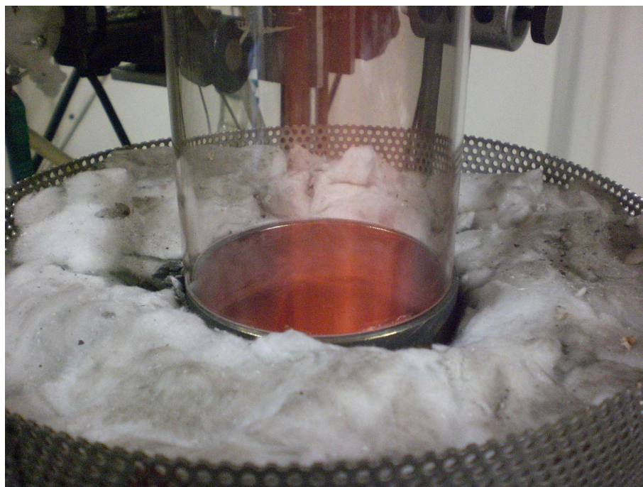
Figure 4.7: Flame on the top of the reforming layer of burner A in diesel reforming at P=7 kW and \varphi=3.0 .
