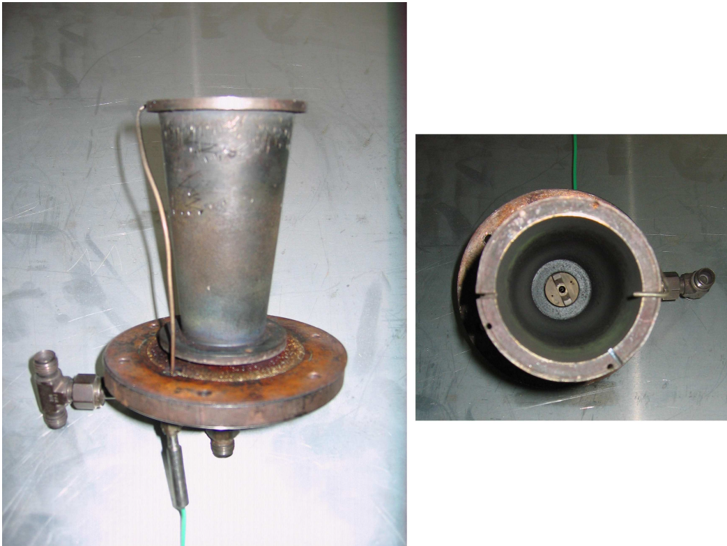
Figure 2.7: Front and top view of the fuel pre-vaporizer. The T_1 thermocouple on top of the cone, the air and fuel inlet and the nozzle are visible in the two photographs.
