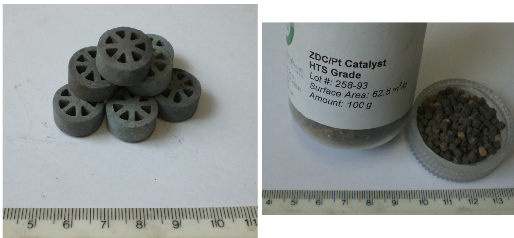
Figure 2.14: (a) Süd-chemie G 90-EW steam reforming catalyst wheels; (b) Fuelcellsmaterial.com ZDC/Pt catalyst pellets.
