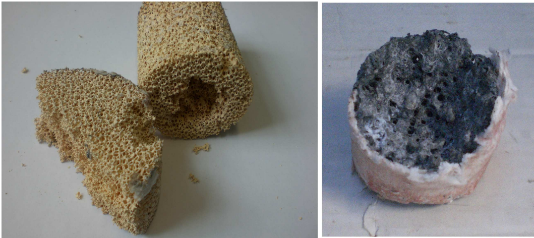
Figure 2.5: Foam failures: (a) ZrO_2 foam cracking after thermal cycles; (b) SiC , Al_2O_3 , SiO_2 compound foam melted after high-temperature operations. The alumina paper wrapping is evident at the side of the cylindrical piece.
