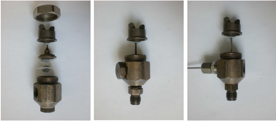
Figure 2.6: Exploded view of the DELAVAN AL-15 nozzle. (a) original version; (b) modified nozzle; (c) modified nozzle with water line.
