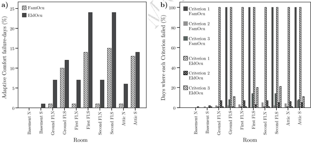
**Fig. 5.** Summertime (May-to-September) Adaptive Comfort [16,32] failure-days (a); and Criterion 1-3 failure-day breakdown (b).
