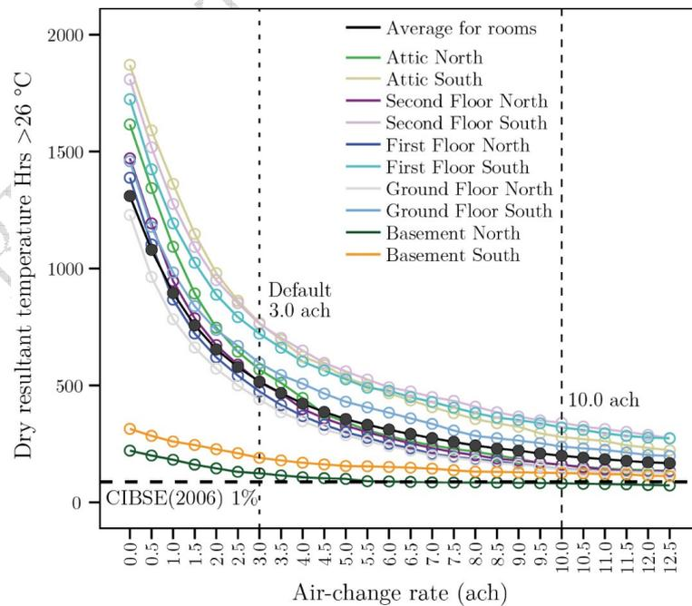
**Fig. 4.** Overheating hours of exceedance (DRT  $>26^{\circ}\text{C}$ ) variation with increasing air-change rate.
