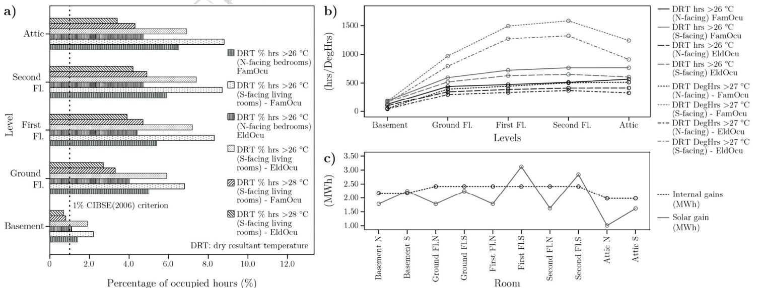
**Fig. 3.** Summertime overheating hours of exceedance by profile, floor level, and room (a); CIBSE hrs  $>26^\circ\text{C}$  and EST degree-hrs  $>27^\circ\text{C}$  by floor level, room, and profile (b); and thermal gains by floor level and room for FamOcu profile (c).
