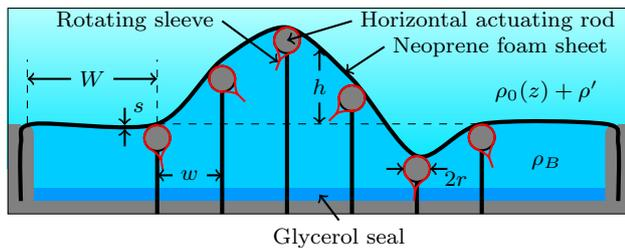
**Fig. 2** Longitudinal view of a wave maker shown schematically with six horizontal rods. The cavity underneath the surface of this wave maker is filled with dense, homogeneous salt water of density,  $\rho_B$ , with a Boussinesq stratification above the wave maker. A layer of glycerol (dark blue) in the base of the cavity inhibits the ingress of salt down the vertical shafts. The dimensions shown are used in Sect. 3
