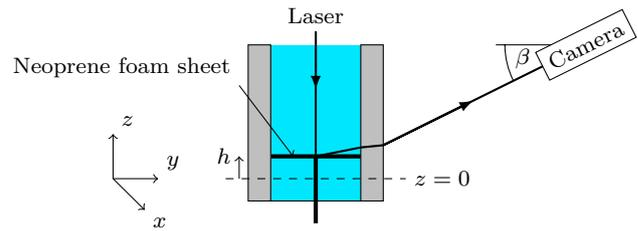
**Fig. 9** Apparatus for optically measuring height of wave maker. A line laser illuminates the centreline of the wave maker from above, which is recorded through the transparent side wall of the tank by a camera
