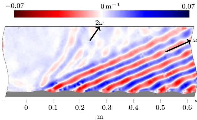
**Fig. 13** Clean horizontal gradient field of the normalised density perturbation  $\frac{1}{\rho_{00}} \frac{\partial \rho'}{\partial x}$  for a sinusoid of amplitude 0.005 m with  $k_0 = 60 \text{ rad m}^{-1}$  and  $\omega = 0.6 \text{ rad s}^{-1} \approx 0.41 \text{ N}$
