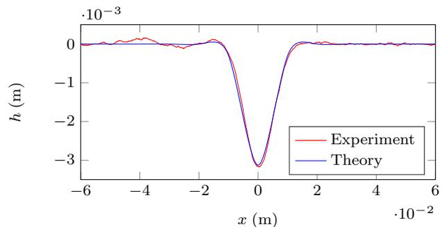
**Fig. 10** Comparison of theory with profile recorded on the apparatus for one rod of the wave maker displaced down by  $3.81 \times 10^{-3}$  m. The prediction has a small RMS error of  $4 \times 10^{-5}$  m and exhibits the small humps around  $x = \pm 1.3 \times 10^{-2}$  m, which result from the bending stiffness
