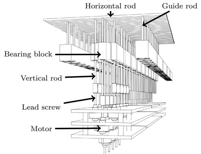
**Fig. 3** Perspective drawing of the arrangement of the wave maker linear actuators. The vertical rods are driven up and down, which determines the instantaneous height of each horizontal rod. The neoprene foam sheet of the wave maker is attached to these horizontal rods, so its shape is determined by their heights. The motors are staggered across three horizontal and three vertical planes to enable a tight rod separation of 10 mm
