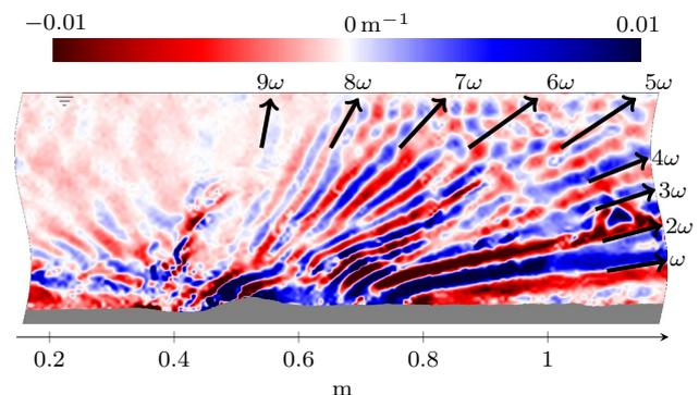
**Fig. 12** Horizontal gradient of the normalised density perturbation  $\frac{1}{\rho_{00}} \frac{\partial \rho'}{\partial x}$  for a sinusoid of amplitude 0.018 m with a  $\cos^2 x$  envelope,  $k_0 = 20 \text{ rad m}^{-1}$  and  $\omega = 0.19 \text{ rad s}^{-1} \approx 0.108 \text{ N}$ . The narrow active zone produces a broad spectrum of waves with both positive and negative wavenumbers, including nine harmonics
