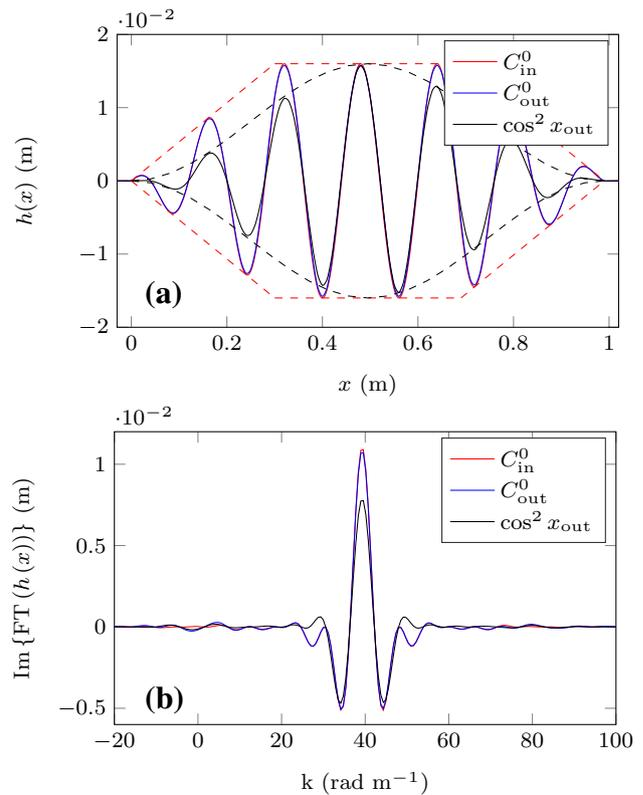
**Fig. 11** Instantaneous shapes and spectra for two classes of amplitude envelope for a travelling sinusoid with  $k_0 = \frac{2\pi}{\frac{1}{6} \times 0.96} \approx 39.3 \text{ rad m}^{-1}$ . The red line shows the input that produces the blue output waveform; there is very little difference (RMS error =  $4.7 \times 10^{-4} \text{ m}$ ), except for a slight reduction in amplitude due to the elasticity in the rod attachments
