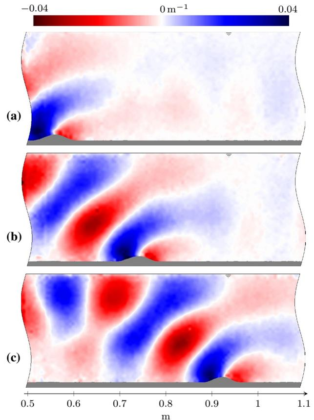
**Fig. 14** Horizontal gradient of the normalised density perturbation  $\frac{1}{\rho_{00}} \frac{\partial \rho'}{\partial x}$  for a solitary sinusoidal hump of height 0.0075 m and width 0.09 m moving at  $0.17 \text{ m s}^{-1}$ . Each image is separated by 5 s, and  $N = 1.45 \text{ rad s}^{-1}$
