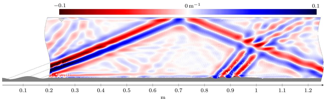
**Fig. 15** Vertical gradient of the normalised density perturbation  $\frac{1}{\rho_{00}} \frac{\partial \rho'}{\partial z}$  for two incident wave beams,  $\omega_{p'} = 0.55 \text{ rad s}^{-1} \approx 0.37 \text{ N}$  generated on the left and  $\omega_{q'} = 2.2\omega_{p'}$  generated on the right end of the
