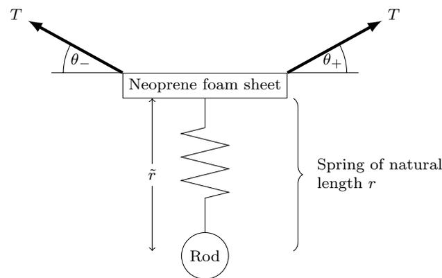
**Fig. 5** Model of forces determining the separation between the neoprene foam sheet and a horizontal metal rod. The upper tensions are those applied on this element by neighbouring elements of the sheet. The hook-and-loop fastening that connects the rod to the sheet is modelled as a spring, which is either in tension or compression proportional to its displacement
