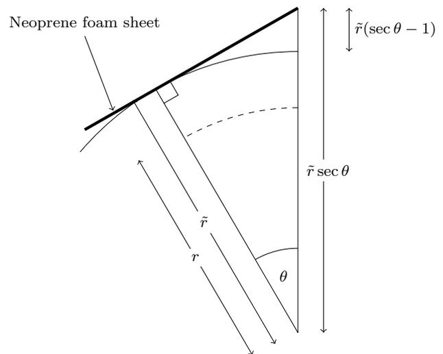
**Fig. 6** Variable contact point of the sheet with the rod. For a rod of radius  $r$ , the neoprene foam sheet sits at a position given by a larger, variable virtual radius  $\tilde{r}$ , due to elasticity in the hook-and-loop attachment. Assuming the bending of the sheet is negligible, its height above the centre of the rod increases by  $\tilde{r}(\sec \theta - 1)$  as the contact point moves away from the top in either direction
