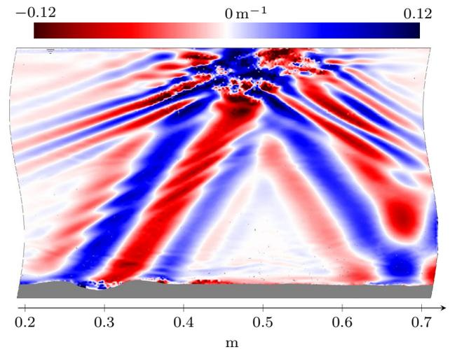
**Fig. 17** Vertical gradient of the normalised density perturbation  $\frac{1}{\rho_{00}} \frac{\partial \rho'}{\partial z}$  showing the breaking of an internal wave (top-centre) of angular frequency  $\omega = 1.5 \text{ rad s}^{-1} \approx 0.84 \text{ N}$ , incident from the bottom-left. New internal waves are emitted from the breaking zone at lower frequencies, both to the left and to the right
