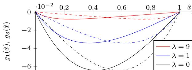
**Fig. 7** Curvature basis functions for the surface of the wave maker shown at various shape parameters,  $\lambda$  using a unit rod spacing ( $d = 1$ ). The solid lines show the basis function  $g_1$  and the dashed lines show its reflection,  $g_3$ . The curves become cubic in the large bending stiffness case when  $\lambda = 0$
