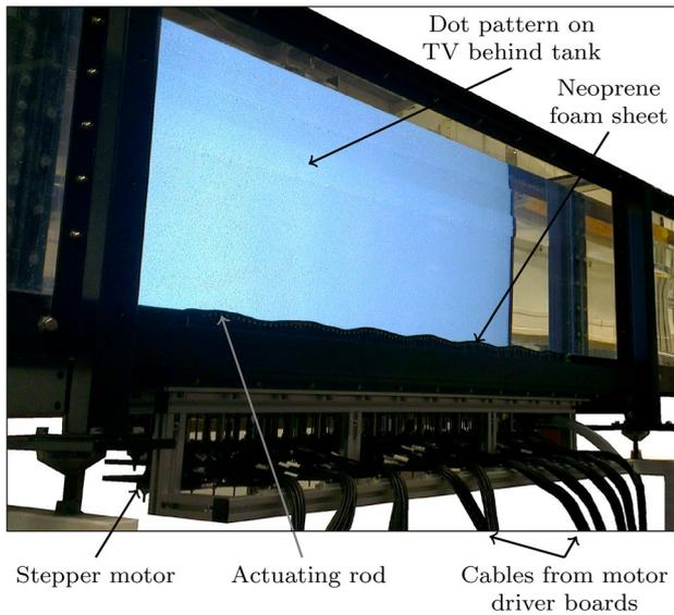
**Fig. 1** Arbitrary spectrum wave maker mounted in the base of the tank. The 100 horizontal actuating rods determine the shape of the neoprene foam sheet. They are driven up and down by an array of stepper motors underneath the wave maker. Each motor is powered via its own driver board, which are all out of the field of view. Behind the tank is the dot pattern on the TV screen used for Synthetic Schlieren
