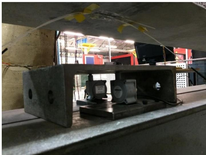
Figure 7-8 The FBGS cables and wire gauges attached on the cement sheath at the bottom centre part of the specimen.
