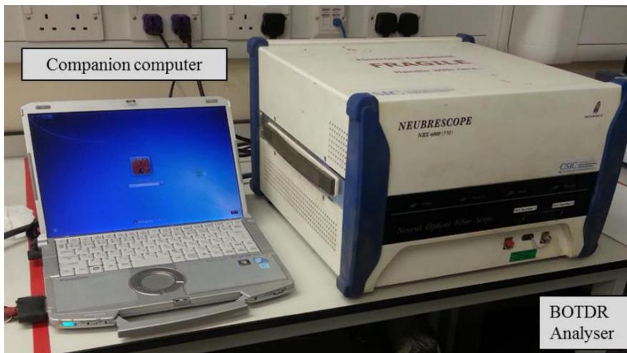
Figure 7-2 The NeubreScope NBX-5000 analyser for BOTDR measurements [After Chunge (2014)].
