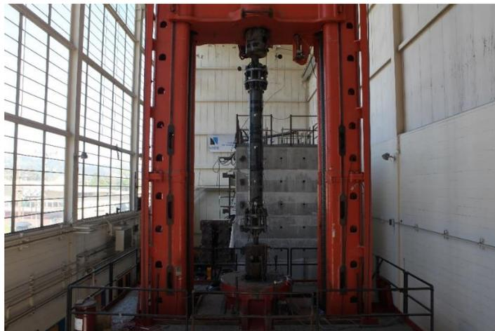
Figure 6-8 The large-scale specimen set up in a loading frame.
