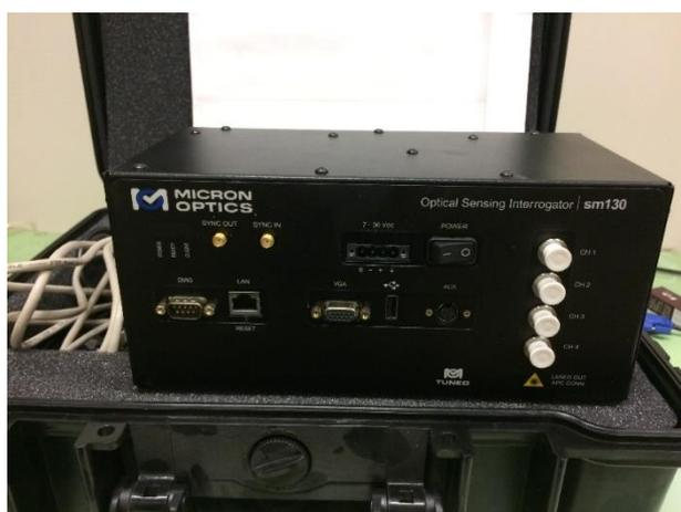
Figure 7-3 The Optical Sensing Interrogator | sm130 for FBGS measurements.
