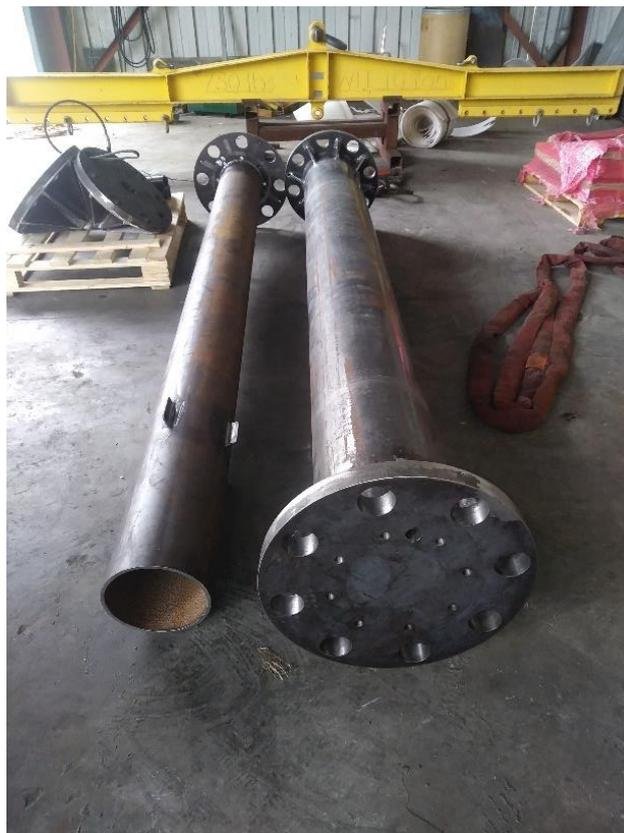
Figure 6-4 The inner casing (left) and the outer casing (right) subassemblies of the large-scale specimen.
