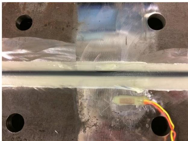
Figure 7-6 A fibre optic cable (Fujikura cable) and a strain gauge installed to the steel box section.
