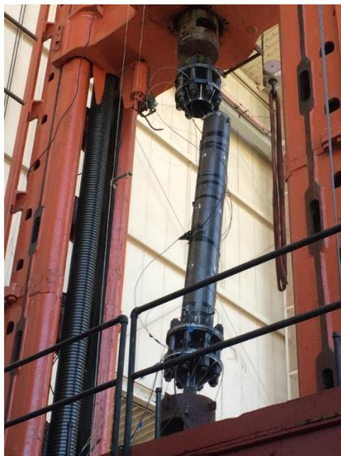
Figure 6-10 Failure of the specimen at the top part of the outer casing.
