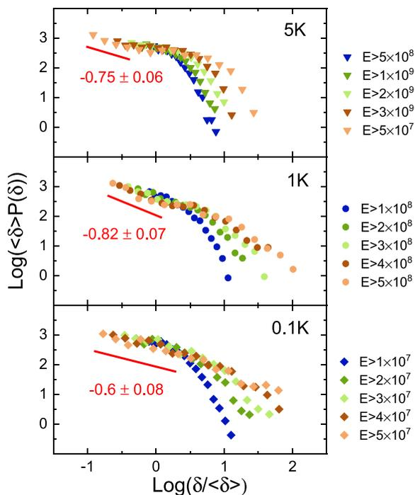
**FIG. 4.** Rescaled probability distribution of waiting time at  $T = 0.1 \text{ K} \sim 5 \text{ K}$ . It follows the power law with the exponents  $-0.8 \sim -0.6$ . The data collapses onto the same line for a short waiting time with different energy thresholds. No scaling behavior exists for a long time period.
