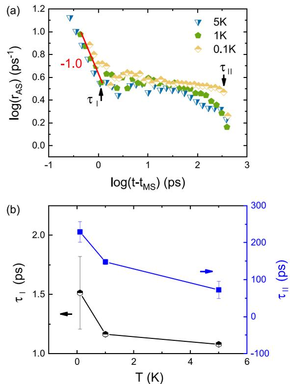
**FIG. 3.** (a) Event rates of jerk generation as a function of time interval at  $T = 0.1$  K ~ 5 K. They follow typical Omori laws with the slope around  $-1$ . Here, two characteristic time constants could be identified as  $\tau_I$  and  $\tau_{II}$ , which correspond to the starting point and ending point of the plateau. (b) The variation of  $\tau_I$  and  $\tau_{II}$  as a function of temperature. Both time constants decrease with the increase in temperature.
