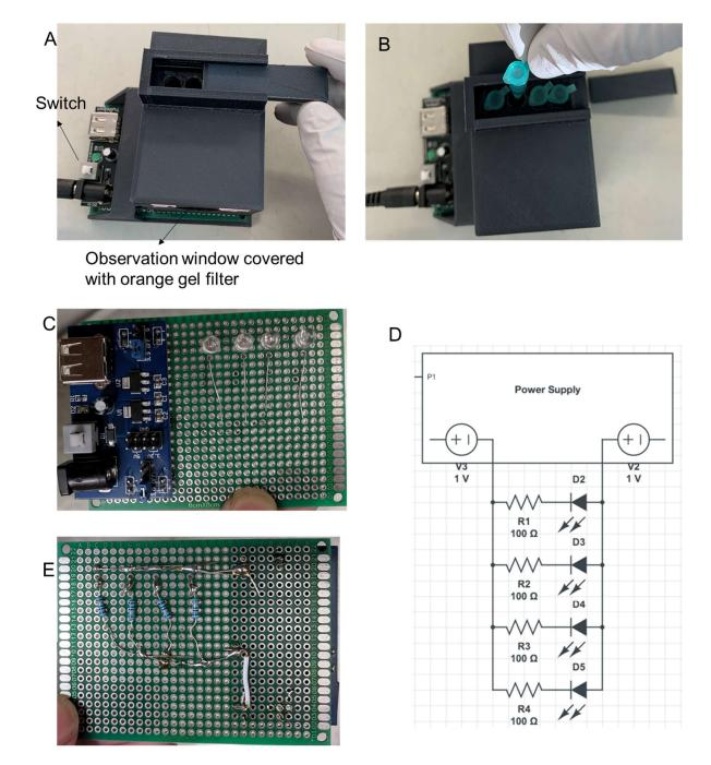
**S14 Fig. Design and construction of fluorescence visualization box.** (A) Visualization box with 3D printed tube chamber and LED circuit board. (B) Image showing placement of LAMP-OSD tubes inside the visualization box. (C) Top view of the LED circuit board. (D) Circuit design. (E) Bottom view of the circuit board. Detail instructions available at https://github.com/Jose-4625/LAMP-BOX-ECO/tree/master/VisBox.
