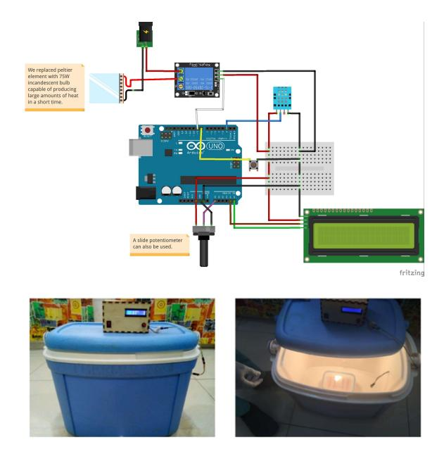
**S3 Fig. DIY incubator built from locally sourced materials.** Top panel: Arduino scheme to control the DIY bioreactor. Bottom panel: DIY incubator final assembly.
