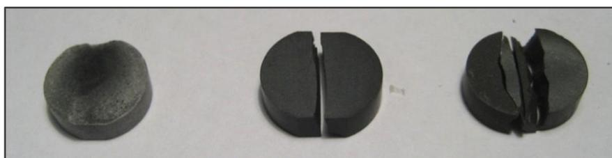
Figure 5.7: Examples of failure modes for diametral compression specimens: shear (left), tensile (middle), triple cleft (right).
