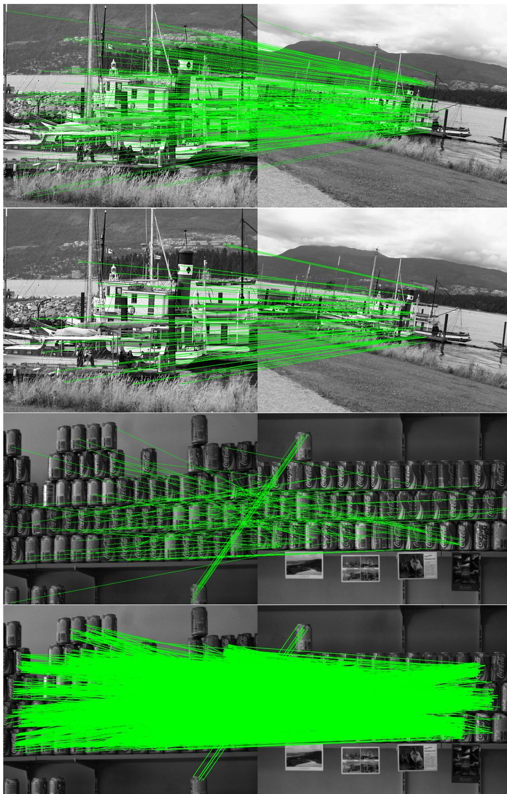
**Fig. 2.** Comparison of the proposed method with SIFT second nearest neighbour criterion. **1st row:** SIFT. **2nd row:** proposed method. **3rd row:** SIFT. **4th row:** proposed method.
