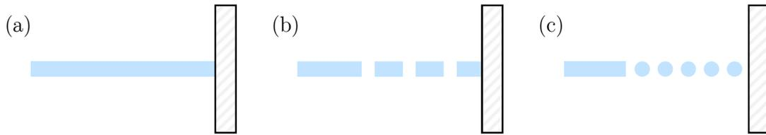
**Figure 5.1:** Schematic of different jet impingement conditions: (a) a coherent continuous jet, (b) a series of rectangular pulses, and (c) complete jet breakup into droplets.
