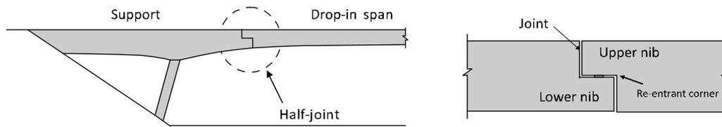
Figure 1: Half-joint principle for reinforced concrete bridges
