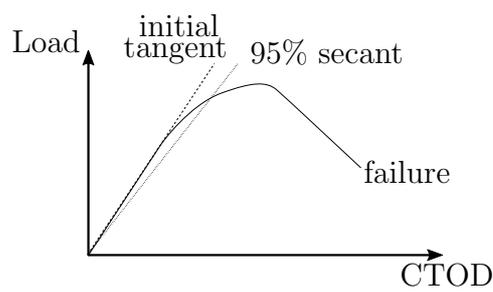
Figure 9.6: Schematic CTOD test data for Alloy 8, showing 95% secant and point of failure.
