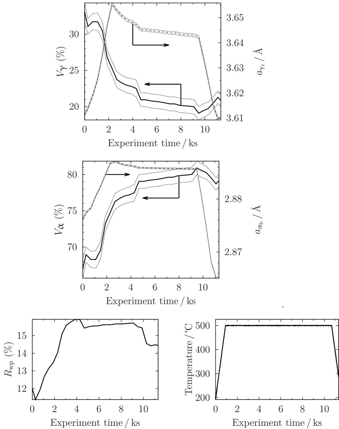
Figure 8.13: Rietveld analysis results for time-resolved synchrotron X-ray diffraction with *in-situ* tempering of Alloy 9 transformed at 275 °C. Grey lines represent  $\pm$  one standard error. Arrows indicate the the relevant axis for each dataset.
