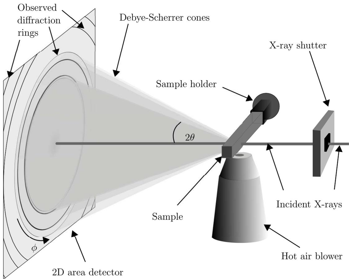
Figure 4.16: Experimental geometry for experiments at DESY
