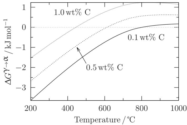
Figure 2.13: Molar driving force for the transformation from austenite to ferrite at a fixed composition,  $\Delta G^{\gamma \rightarrow \alpha}$  as a function of temperature for Fe-0.1 wt% C, Fe-0.5 wt% C and Fe-1.0 wt% C [25, 26]
