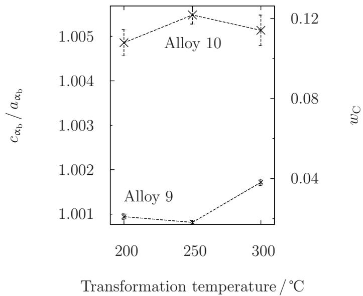
Figure 10.6:  $c_t/a_t$  in Alloy 9 and Alloy 10. The values follow the expectation that Alloy 10 will display more tetragonality than Alloy 9, but the temperature dependence of both alloys is not as expected.
