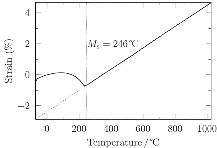
Figure 7.11: Dilatational strain in Alloy 8 cooled at  $10^\circ\text{C s}^{-1}$  in a TA Instruments DIL805A/D dilatometer with  $M_s$  according to the offset method with 5 vol.% transformation [288].
