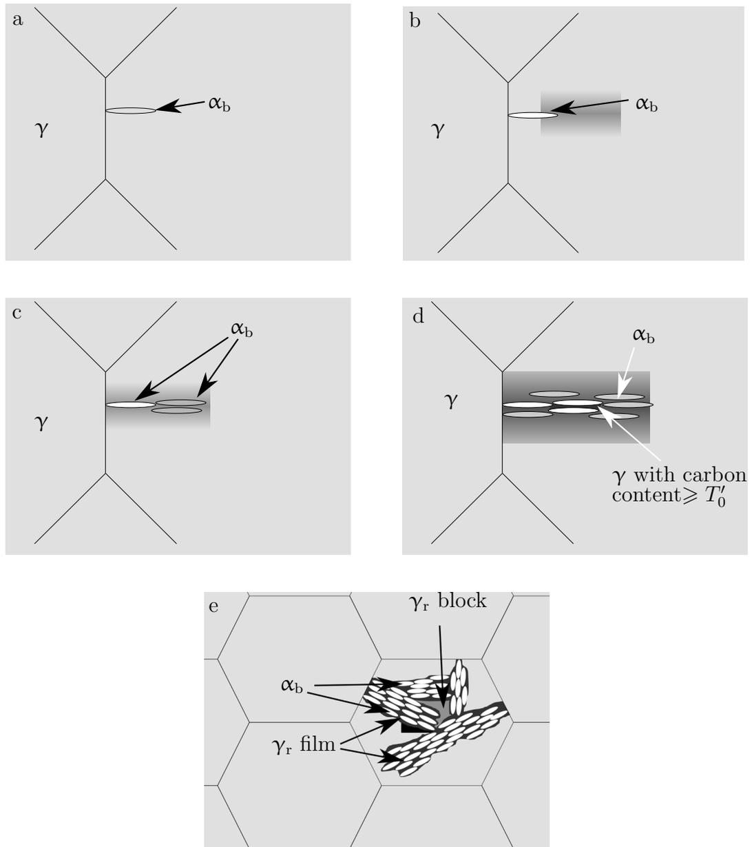
Figure 2.15: Schematic depiction of the formation of carbide-free bainite. White indicates no carbon content, black represents  $x_{T_0}$ . (a) nucleation of the first ferrite sub-unit. Ferrite inherits the carbon content of the parent austenite but then carbon partitions back into austenite (b). (c) this localised carbon enrichment together with work hardening stifles the sub-unit but more nucleate to (d) form a packet. (e) the convergence of packets leads to the formation of blocky austenite.
