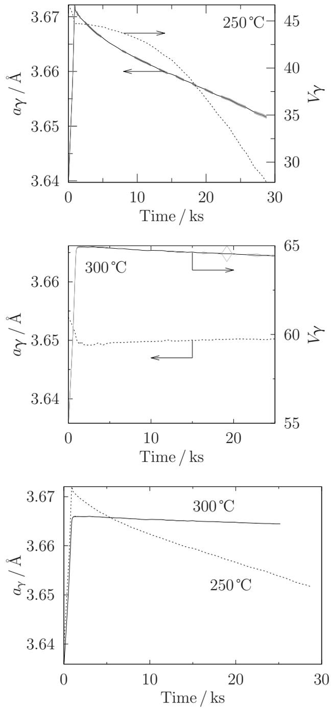
Figure 4.25: Comparison of austenite lattice parameters and volume fractions of Alloy 1 transformed at (a) 250°C and (b) 300°C and tempered at 450°C; (c) austenite lattice parameters from (a) and (b).
