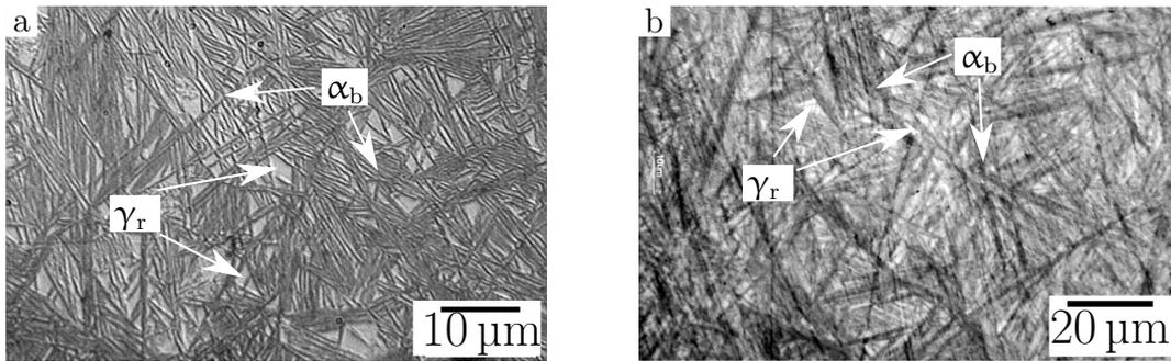
Figure 4.8: Alloy 1 tempered at 400 °C for (a) 10 d and (b) 30 d. Tempering for has little visible effect on the structure.
