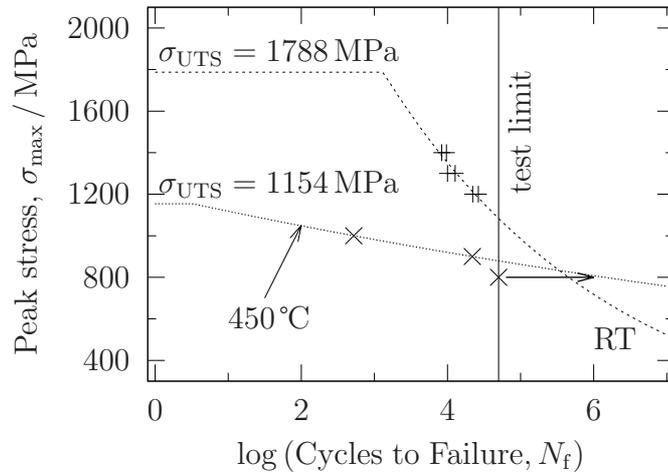
Figure 9.10: Fatigue results for Alloy 8 showing data at ambient temperature (“RT”, +) and 450°C (×). The horizontal lines are the measured  $\sigma_{UTS}$  at the relevant temperature (section 9.1 and the curves are fitted to the data according to the modified Basquin equation (equation 9.5).
