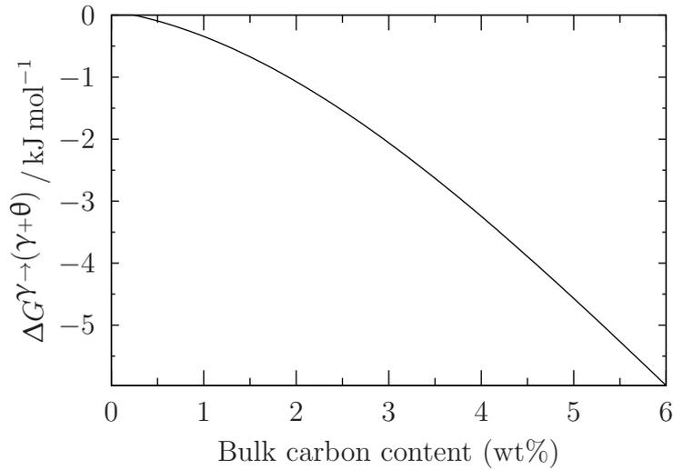
Figure 5.1: Driving force for the precipitation of cementite in austenite in Fe– $x$  wt% C at 400°C calculated using MatCalc thermodynamic modelling software [247, 293]. Decreasing the carbon content is calculated [116] to reduce the driving force for the nucleation of cementite in austenite, which is the limiting step in thermal decomposition of nanocrystalline steels [116, 134].
