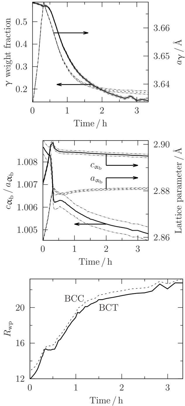
Figure 10.4: Lattice parameter and volume fraction of (a) austenite, (b) ferrite and (c)  $R_{wp}$  in Alloy 1 transformed at 300°C. The results are entirely consistent with tetragonal bainitic ferrite and the lower initial value of  $c_{\alpha_b} / a_{\alpha_b}$  than is seen in figure 10.4 suggests a lower dissolved carbon content than is seen following transformation at 200°C. Thin dashed lines represent  $\pm$  one standard error.
