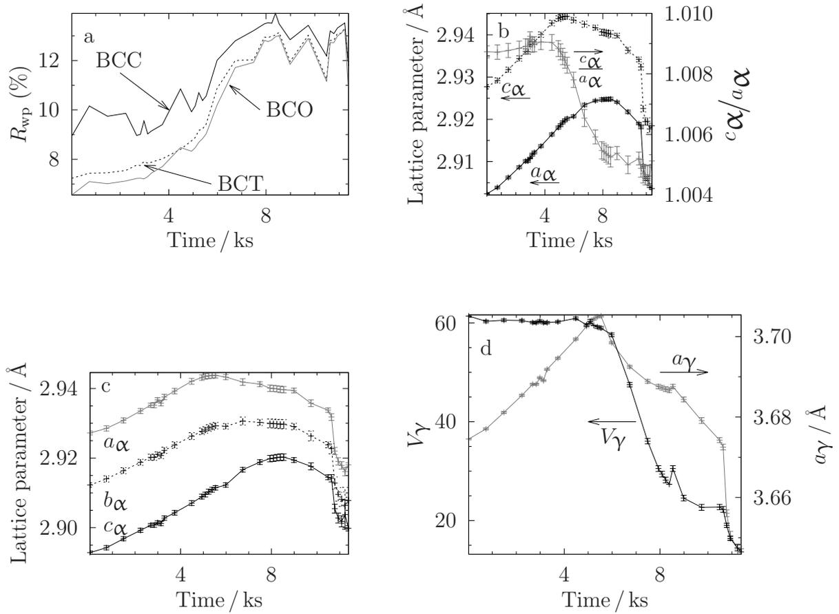
Figure 10.1: (a)  $R_{wp}$ , (b) lattice parameters in body-centred tetragonal ferrite, (c) lattice parameters in body-centred orthorhombic ferrite, (d) austenite volume fraction and lattice parameter for Alloy 2 during heating at  $5\text{ }^{\circ}\text{C s}^{-1}$ . The results are all consistent with a starting crystal structure of BCT in ferrite, which is lost during prolonged tempering. Error bars on the points represent one standard error.
