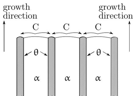
Figure 2.4: Schematic representation of the growth direction and diffusion directions during the pearlite transformation
