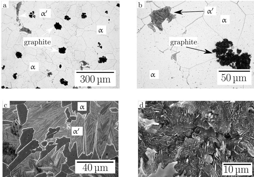
Figure 7.21: Alloy 8 after isothermal transformation at 800°C for 4.5 h. (a) and (b) optical micrographs. (c) scanning electron micrograph of martensite plates in ferrite and (d) a graphite nodule.
