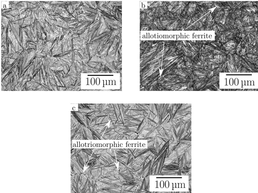
Figure 7.12: Martensitic structure formed in Alloy 8 cooled to ambient temperature at (a)  $10^{\circ}\text{C s}^{-1}$ , (b)  $5^{\circ}\text{C s}^{-1}$  and (c)  $2^{\circ}\text{C s}^{-1}$ . Cooling at  $10^{\circ}\text{C s}^{-1}$  results in no visible allotriomorphic ferrite. Allotriomorphic ferrite does form at the lower cooling rates.
