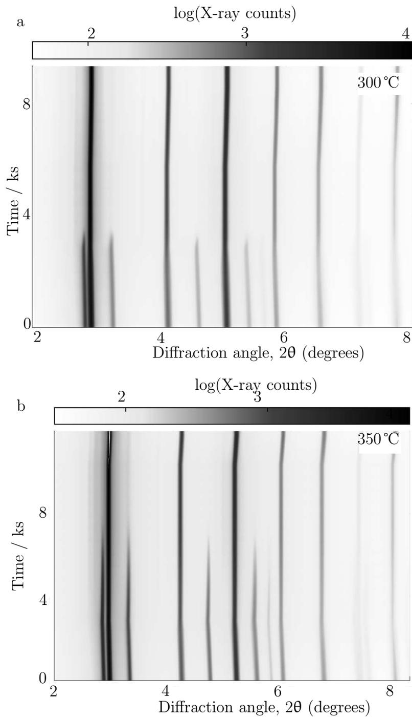
Figure 8.5: Time-resolved synchrotron X-ray diffraction results for Alloy 8 transformed at (a) 300°C and (b) 350°C.
