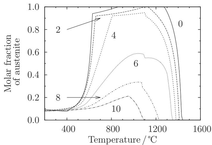
Figure 5.5: Phase fraction of austenite in the system Fe-1.0C-10.0Ni- $x$  Al [26, 199].
