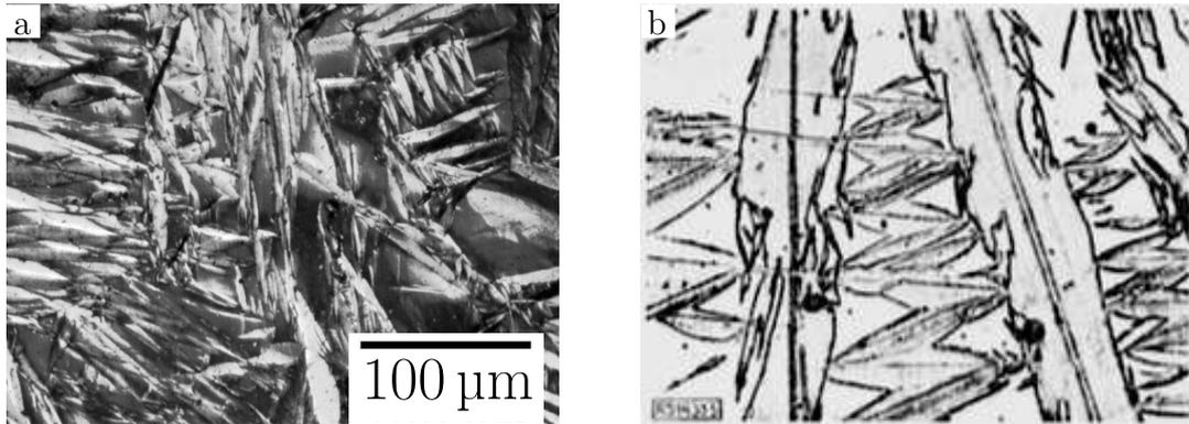
Figure 2.11: Optical micrographs of martensite, (a) Fe–30 wt% Ni–0.4 wt% C. Adapted from [14, micrograph 846]; (b) zig-zag arrangement of martensite in Fe–29 wt% Ni [32] (no scale bar provided).
