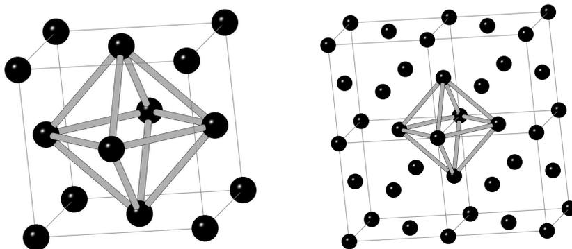
Figure 2.24: Octahedral interstices in a face-centred cubic crystal. Left: at the body centre and right: at the edge-centres. After Cohen [236, figure 7].
