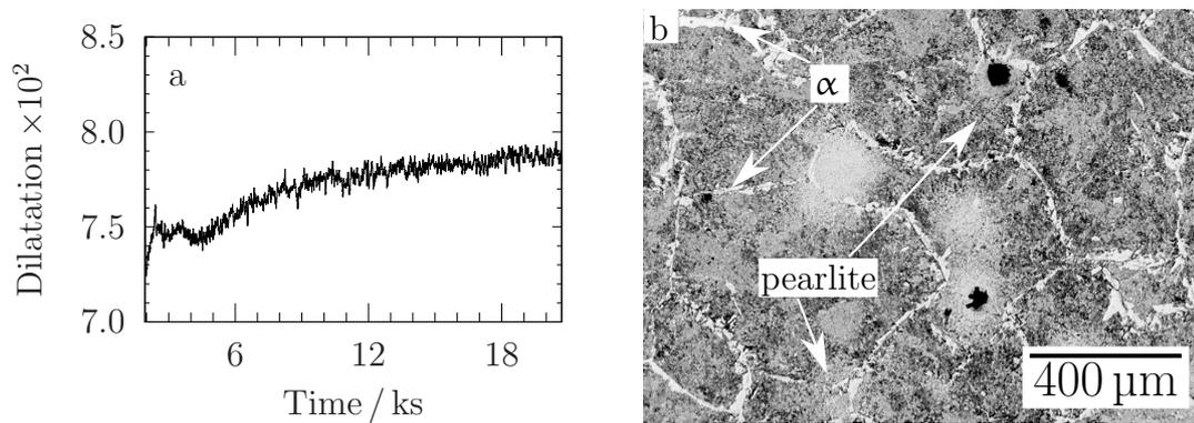
Figure 7.27: (a) dilatational strain measured during isothermal holding of Alloy 8 at 600°C for 5.5 h—the strain does not become horizontal before the end of the isothermal hold, consistent with a transformation in progress at the time of quenching; (b) microstructure formed after 24 h at 600°C. The dilatational strain was found to become horizontal before the end the isothermal hold, suggesting the transformation had ceased before quenching, consistent with a mixture of ferrite and pearlitic
