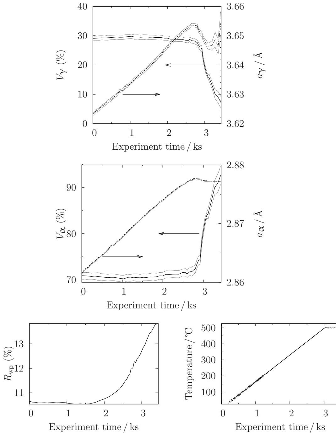
Figure 8.8: Rietveld refinement results for Alloy 8 transformed at 350°C and investigated using synchrotron XRD with *in-situ* heating. Grey lines represent  $\pm$  the standard error for each measurement.
