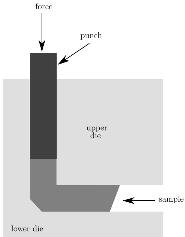
Figure 2.17: Schematic of equal-channel angular extrusion [after 97, figure 5]
