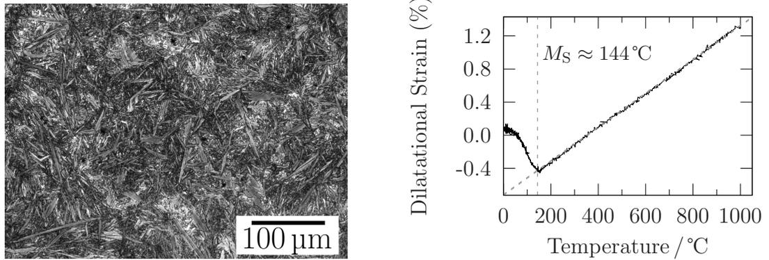
Figure 7.13: (a) microstructure and (b) dilatational strain profile of Alloy 9 austenitised and then cooled at  $10^\circ\text{C s}^{-1}$  to ambient temperature. Reconstructive transformations are avoided and the structure is martensitic.
