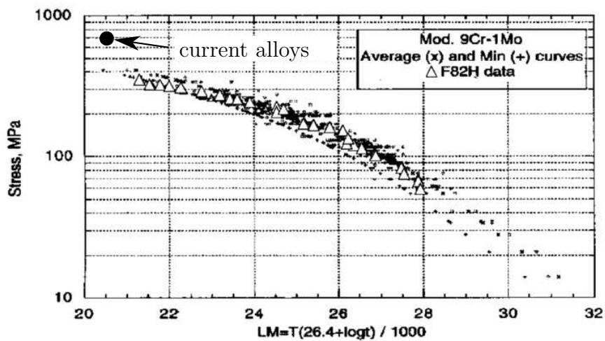
Figure 9.18: Comparison of current alloys to data for 9Cr-1Mo (wt%) (small crosses) and reduced-activation martensitic steel (triangles) collated by Jitsukawa et al. [330]. The current alloys outperform those studied by Jitsukawa et al. Figure reproduced with permission of Elsevier B. V.
