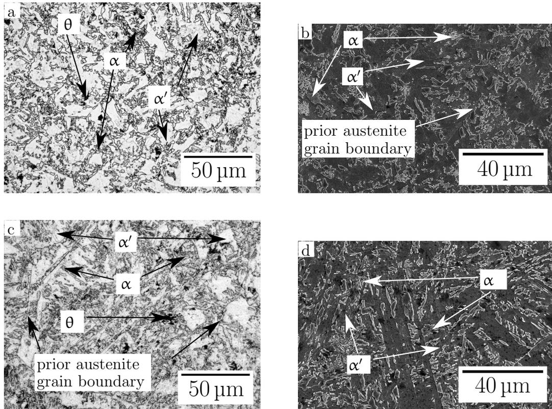
Figure 7.25: Alloy 8 transformed at (a) and (b) 600°C for 5.5 h; (c) and (d) 550°C for 6.5 h. The microstructure consists of large ferrite grains formed on prior austenite grain boundaries interspersed with regions of martensite and smaller dark regions of cementite or possibly pearlite.
