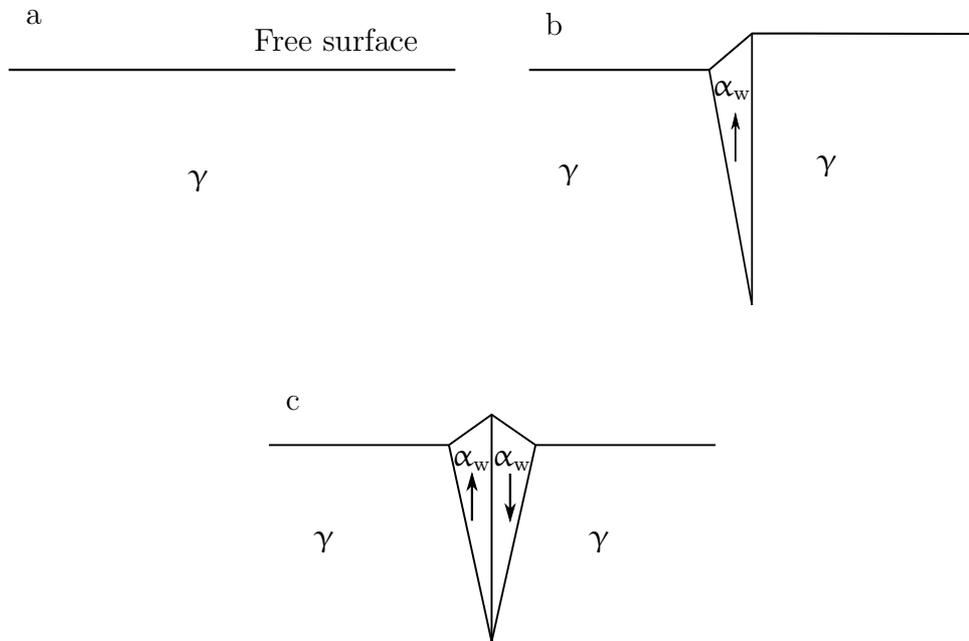
Figure 2.10: Nucleation of Widmanstätten ferrite. Arrows indicate the shear strain caused by the transformation. (a) before nucleation; (b) deformation if one ferrite plate forms and (c) deformation if two ferrite plates nucleate back-to-back.
