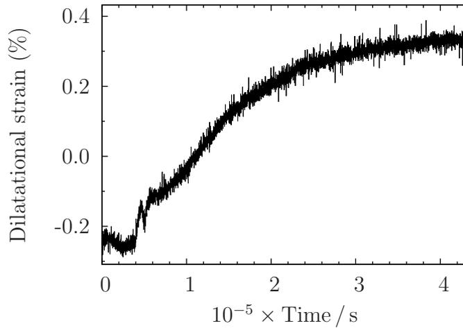
Figure 7.39: Dilatational strain Alloy 9 held at 250°C. The initial strain is negative, consistent with the change from (as-received) martensite to austenite. After 18.5 h ( $0.65 \times 10^5$  s), the dilatational strain has hardly changed from the initial value and after 120 h, the transformation appears to be stopping.
