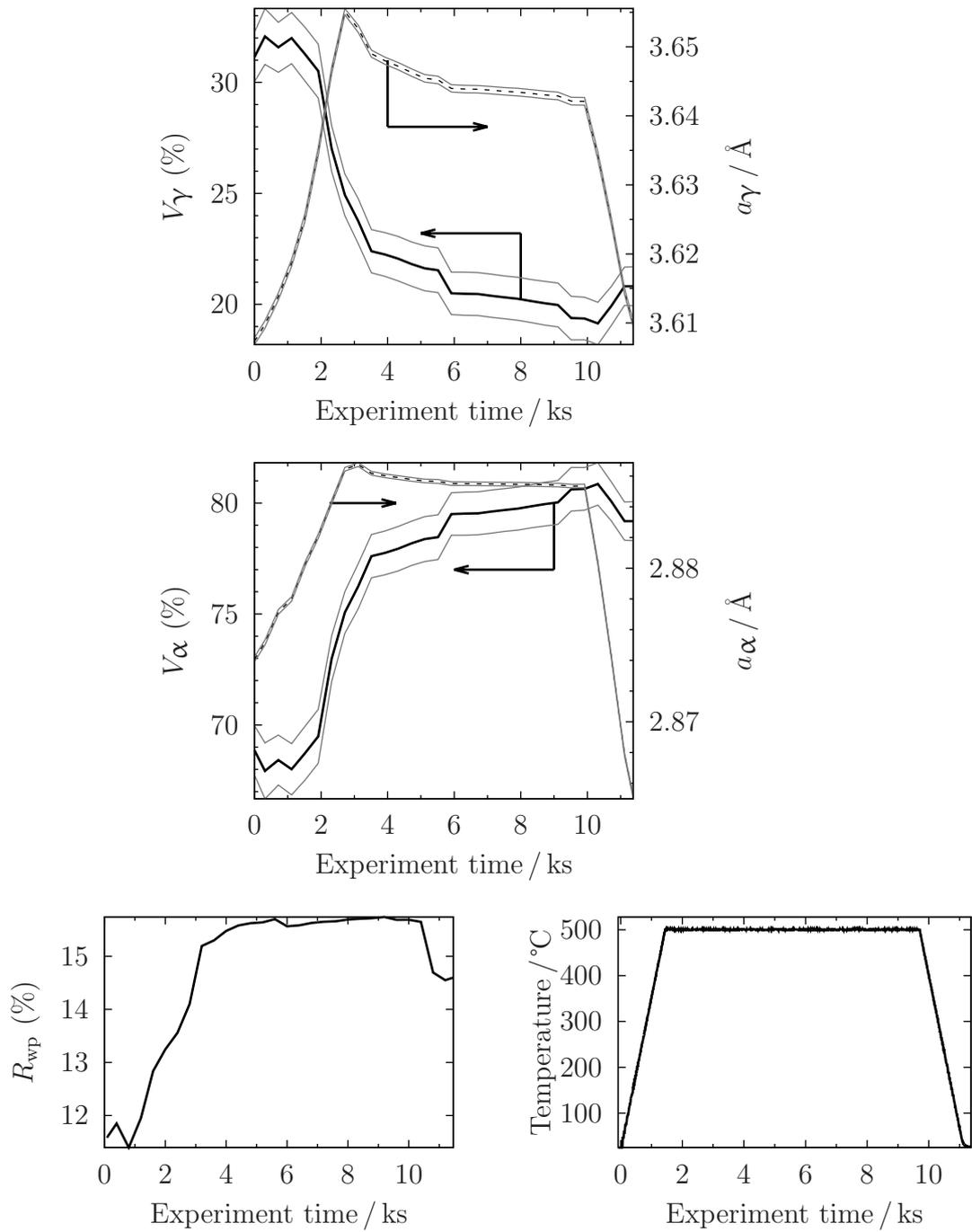
Figure 8.11: Rietveld analysis results for time-resolved synchrotron X-ray diffraction with *in-situ* tempering of Alloy 9 transformed at 225°C. Grey lines represent  $\pm$  one standard error. Arrows indicate the the relevant axis for each dataset.
