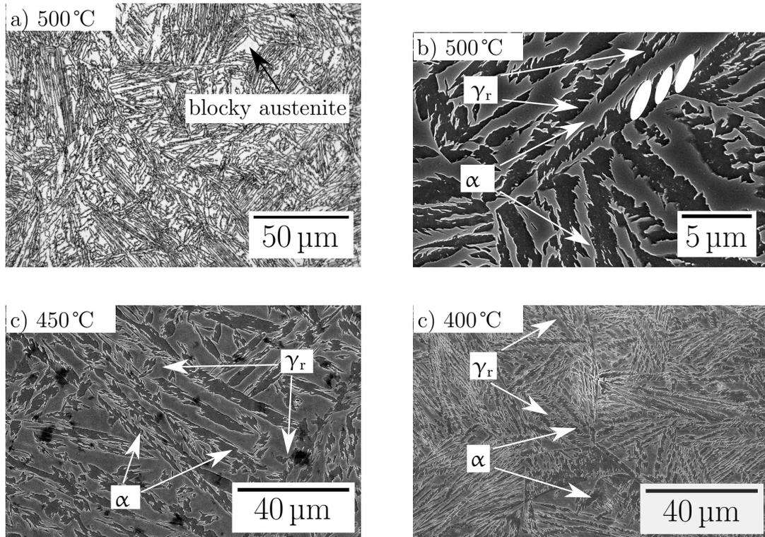
Figure 7.29: Alloy 8 transformed at the temperatures indicated. The dark regions in (c) are artefacts — the microstructure may be seen to continue unchanged through the dark regions. Lenticular shapes may be observed in ferrite, highlighted in figure 7.29(b), indicative of displacive transformation.
