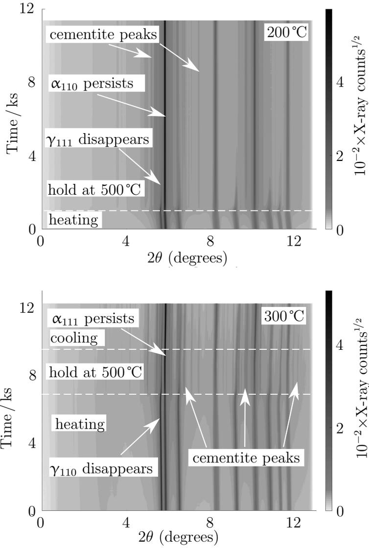
Figure 4.24: Synchrotron XRD data recorded from Alloy 1 transformed at the temperatures indicated during *in-situ* tempering at 500 °C. The square root of the number of observed counts is shown to allow small peaks to be observed.
