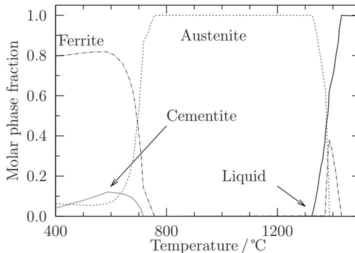
Figure 5.7: Calculated equilibrium phase fractions for Alloy 5 calculated using Thermo-Calc software [248, 249]. The alloy is predicted to be completely austenitic between 740 °C and 1320 °C.
