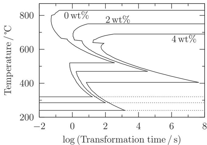
Figure 5.2: TTT curves calculated using mucg83 [241] for Fe–0.7 C–4.0 Si–1.4 Al–0.2 Mo– $y$  Ni (wt%). The nickel content is indicated on each curve. It is possible to derive sufficient hardenability to avoid reconstructive transformations using nickel.
