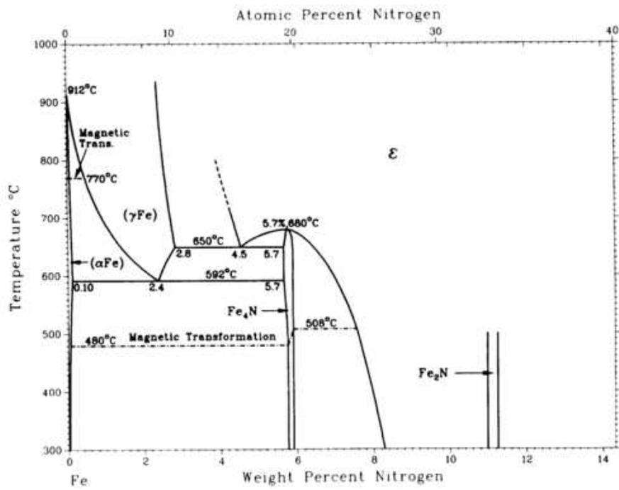
Figure 2.20: Iron–nitrogen equilibrium phase diagram [157]. Reproduced from [10] with permission of ASM International.
