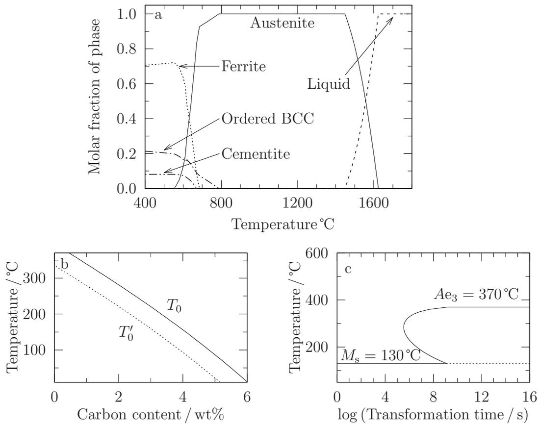
Figure 6.6: (a) equilibrium phase fractions calculated using MatCalc [247, 293]; (b)  $T_0$  and  $T'_0$  lines and (c) TTT curve calculated using MTTTData [199, 254, 259] for the experimentally-measured composition of the Alloy 9 cast.
