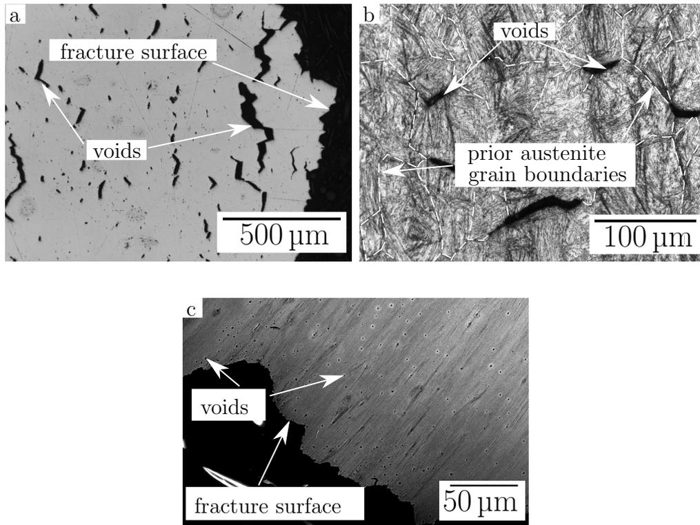
Figure 9.20: Voids formed during creep testing under 700 MPa at 450°C of (a) immediately below the fracture surface of Alloy 9, appearing to follow austenite grain boundaries; (b)  $\approx 1$  cm below the fracture surface of Alloy 9 with austenite grain boundaries highlighted, creep applied in the vertical direction; (c) Alloy 8.
