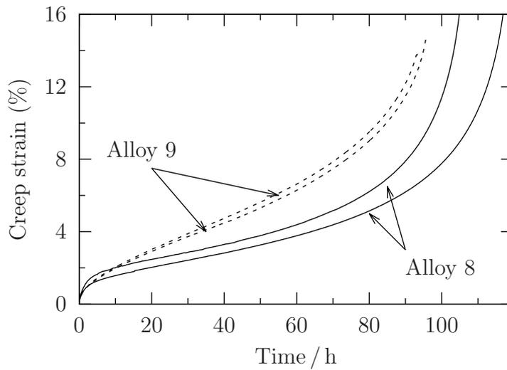
Figure 9.17: Measured creep data for two samples each of Alloy 8 and Alloy 9 under 700 MPa constant stress at 450°C. The creep curve shows that creep is extensive in both time and strain after the minimum strain rate occurs.
