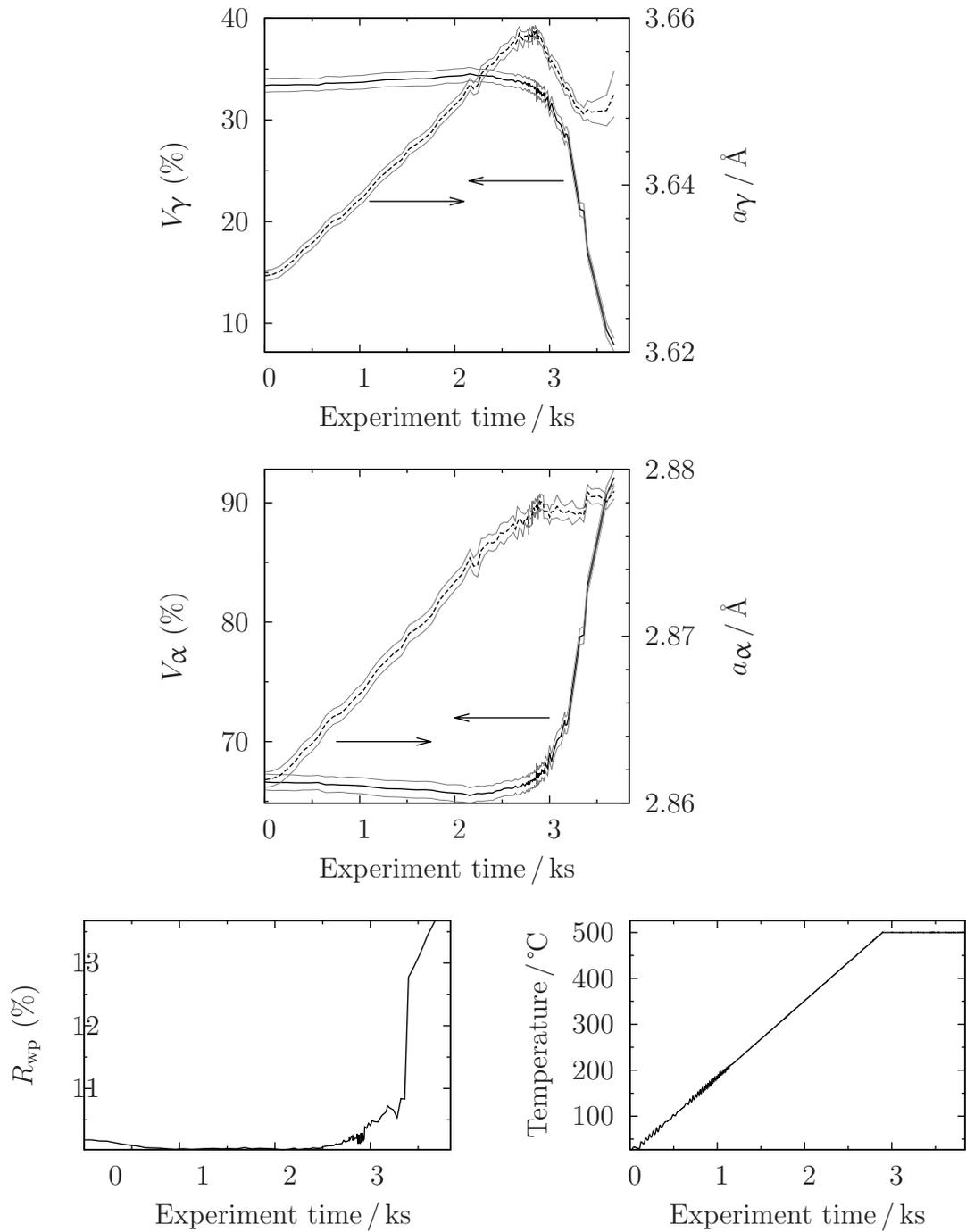
Figure 8.7: Rietveld refinement results for Alloy 8 transformed at 300°C and investigated using synchrotron XRD with *in-situ* heating. Grey lines represent  $\pm$  the standard error for each measurement.
