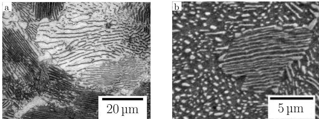
Figure 2.5: Micrographs showing the possible morphologies of pearlite, (a) optical micrograph with dark cementite adapted from [14, micrograph 15] and (b) with cementite bright, adapted from [14, micrograph 20]. The inversion of the shading is a result of the differing imaging techniques.
