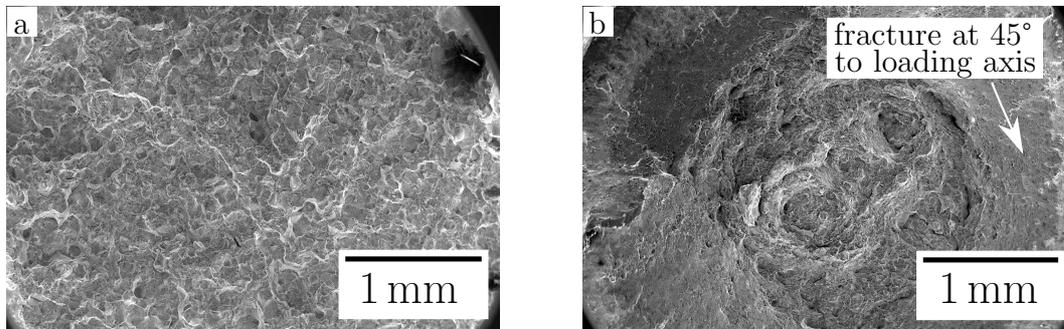
Figure 9.2: Fracture surfaces of (a) Alloy 8 and (b) Alloy 9 after tensile testing in the as-transformed condition. The region labelled as lying at  $45^\circ$  is involved in cup-and-cone failure.
