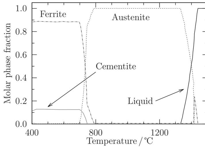
Figure 5.8: Calculated equilibrium phase fractions for Alloy 6 calculated using Thermo-Calc software [248, 249]. The alloy is predicted to be completely austenitic between 790°C and 1320°C.
