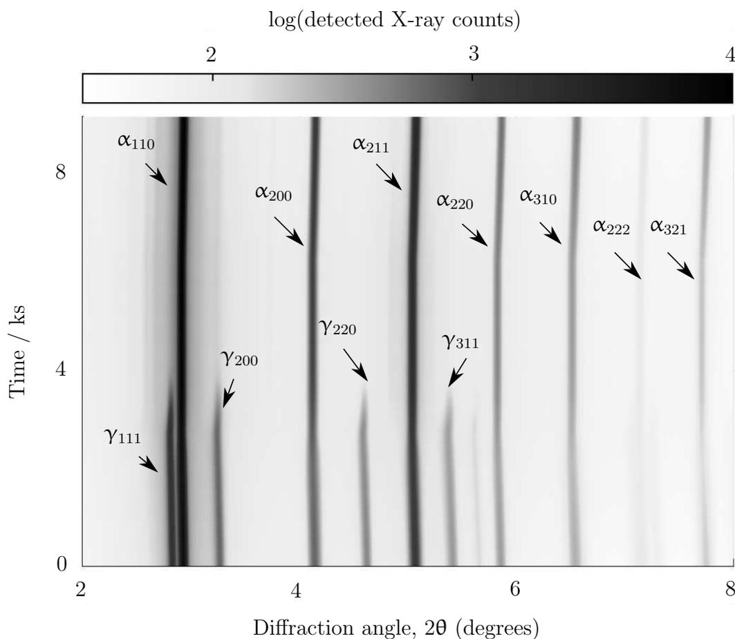
Figure 8.4: Time-resolved plot of synchrotron X-ray diffraction data for Alloy 8 transformed at 250°C, with austenite and ferrite peaks labelled.
