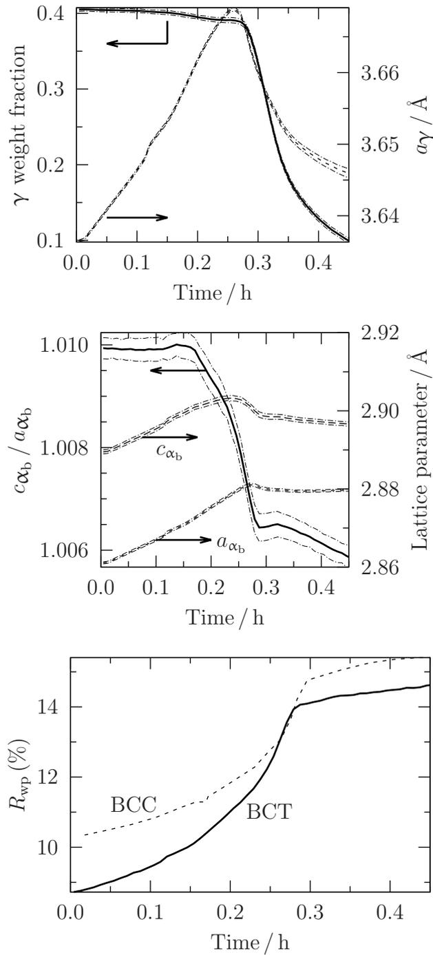
Figure 10.3: Lattice parameter and volume fraction of (a) austenite, (b) ferrite and (c)  $R_{wp}$  in Alloy 1 transformed at 200°C. The results are entirely consistent with tetragonal bainitic ferrite. The thin dashed lines represent the data  $\pm$  one standard error.
