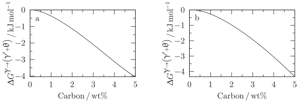
Figure 2.19: Driving force for decomposition of austenite to an equilibrium mixture of austenite and cementite at 450°C [25, 26]. (a) Fe- $x$ C-3.0Mn-2.3Si (wt%) as investigated by Saha Podder [134]; (b) Fe- $x$ C.
