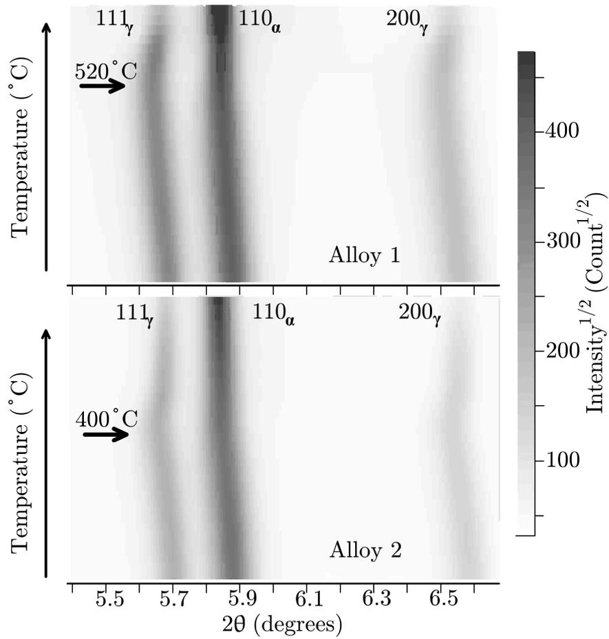
Figure 4.19: Diffraction data during *in-situ* heating of Alloy 1 and Alloy 2. Arrows indicate temperature at the time of minimum detected diffraction angle (maximum lattice parameter) of the austenite 111 peak. Reproduced with permission of Elsevier B. V.
