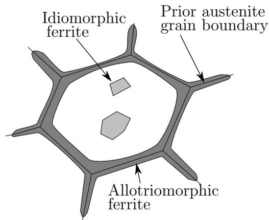
Figure 2.2: Schematic representation of allotriomorphic and idiomorphic ferrite.
