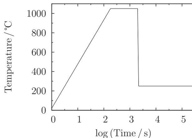
Figure 4.6: Schematic heat treatment of Alloy 1, transformation at  $250^\circ\text{C}$ .
