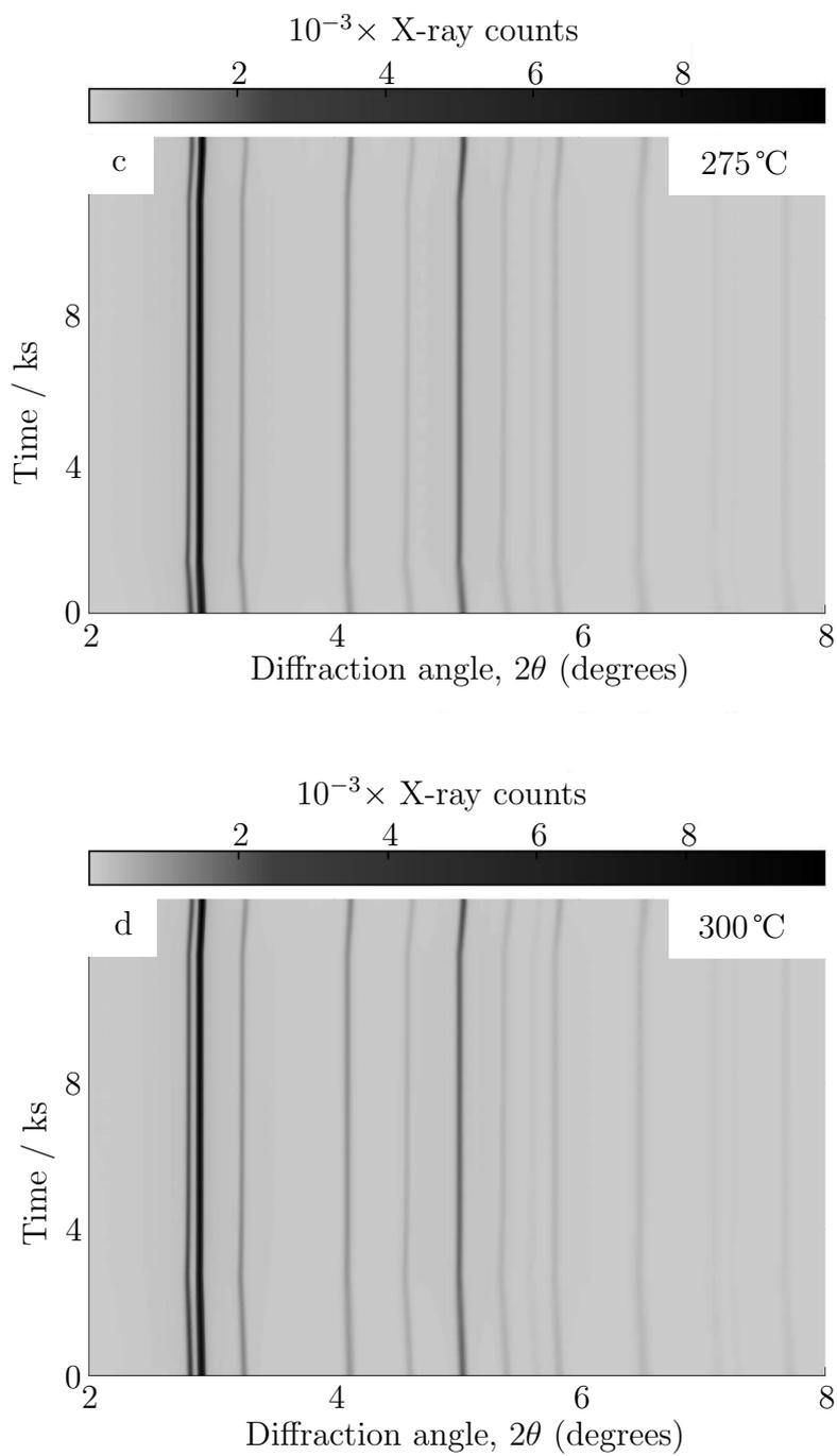
Figure 8.10: Time-resolved synchrotron X-ray diffraction results for Alloy 9 transformed at the temperature indicated on each figure.
