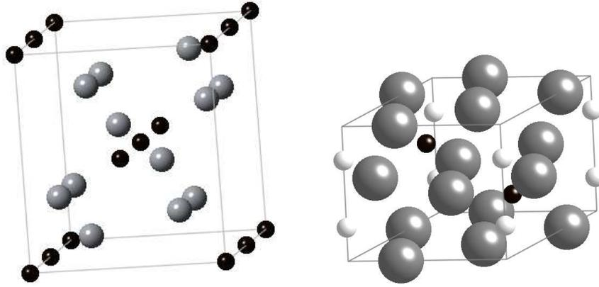
Figure 2.18: Unit cells of tempering carbides. Left: cementite — black atoms are carbon, grey atoms are iron. [135–138]; right:  $\epsilon$ -carbide. Large, grey atoms are iron; small, black atoms are carbon sites that are fully occupied and small, light grey atoms are carbon sites with an average occupancy of 6.25% [139].
