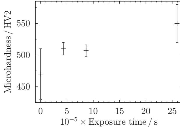
Figure 4.9: Microhardness of Alloy 1 subjected to tempering at 400°C for the times indicated. Exposure for  $4 \times 10^5$  s (5 d) is sufficient to cause a significant change in hardness, presumably due to a change in structure.
