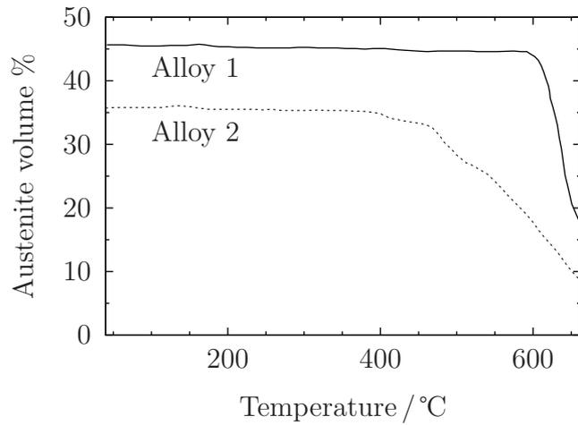
Figure 4.17: Synchrotron X-ray diffractometry results for Alloy 1 and Alloy 2 during continuous heating at  $5^{\circ}\text{C s}^{-1}$ . The austenite in Alloy 1, which is designed to resist thermal decomposition, survives to higher temperatures than the conventional Alloy 2.
