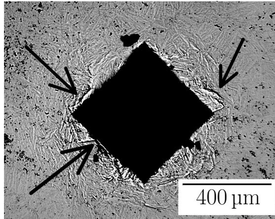
Figure 7.18: Surface cracks around indent during Vickers hardness testing with 30 kg applied load. This led to the exclusion of these data from the analysis of the microstructure and the hardness measured by applying 10 kg, which did not cause cracking, was used instead.
