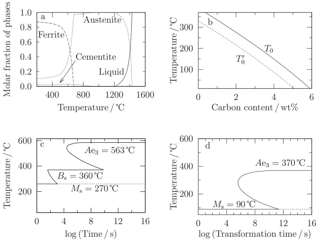
Figure 6.3: (a) calculated equilibrium phase fractions calculated using MTData [26, 199]; (b)  $T_0$  and  $T'_0$  lines calculated using MTTTData [199, 254, 259]; and TTT diagrams, calculated using (c) mucg83 [241] and (d) MTTTData for the designed composition of Alloy 9.
