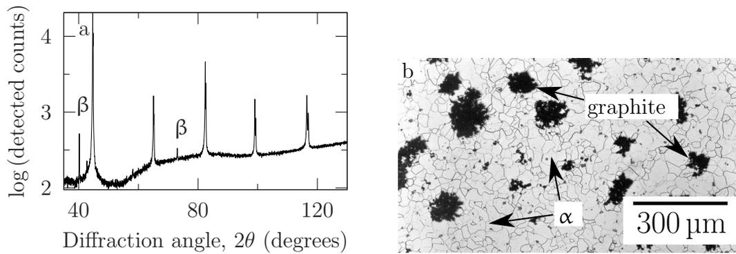
Figure 7.22: (a) XRD data for Alloy 8 transformed at 800°C, with peaks due to  $\text{CuK}_{\alpha 1}$ ,  $\text{CuK}_{\alpha 2}$  and  $\text{CuK}_{\beta}$  radiation. (b) graphite in Fe-2.4C-1.1Si-1.1Mn held at 900°C for several days to grow graphite nodules [14, micrograph 368].
