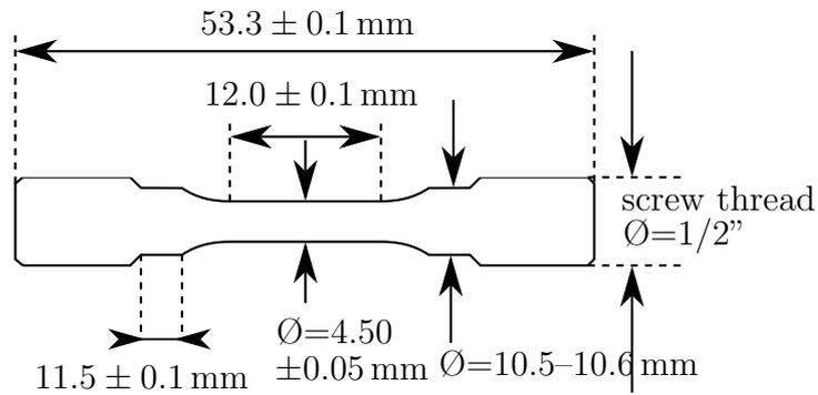
Figure 9.8: Schematic drawing of a fatigue specimen used in the current study. The screw threads of each sample were shot peened to prevent failure outside the gauge length.
