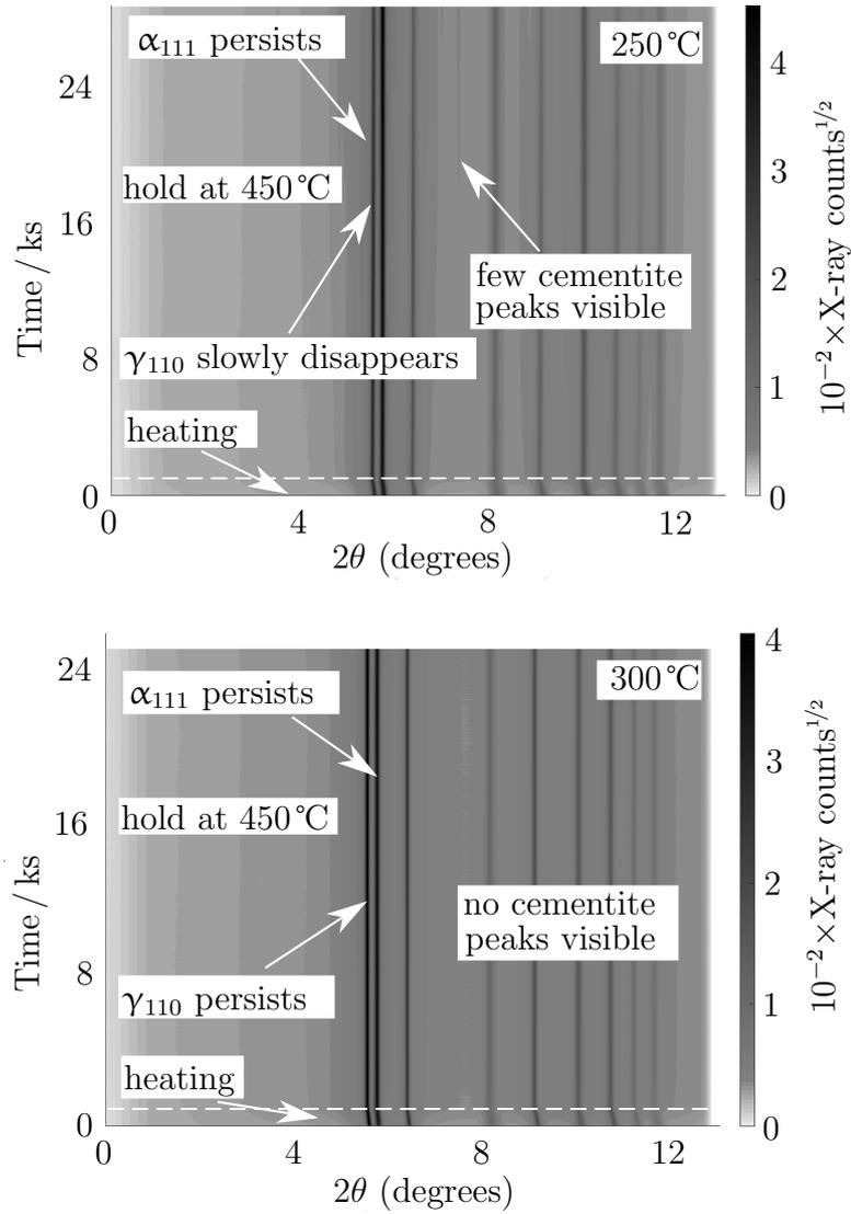
Figure 4.26: Synchrotron XRD data recorded from Alloy 1 transformed at the temperatures indicated during *in-situ* tempering at 450°C. The square root of the number of observed counts is shown to allow small peaks to be observed.
