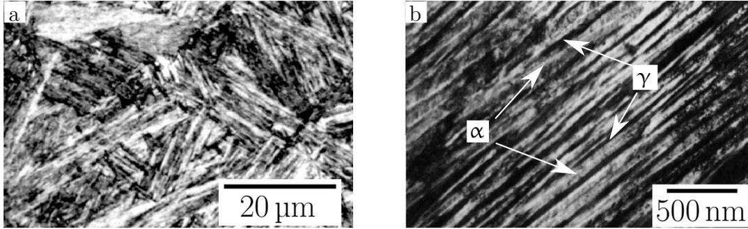
Figure 2.12: Micrographs showing bainite at different scales. (a) optical micrograph showing bainite packets. Optical microscopy cannot resolve individual ferrite sub-units and retained austenite films. (b) transmission electron micrograph of the interior of a bainite packet, showing retained austenite films and ferrite sub-units. Both adapted from [67].
