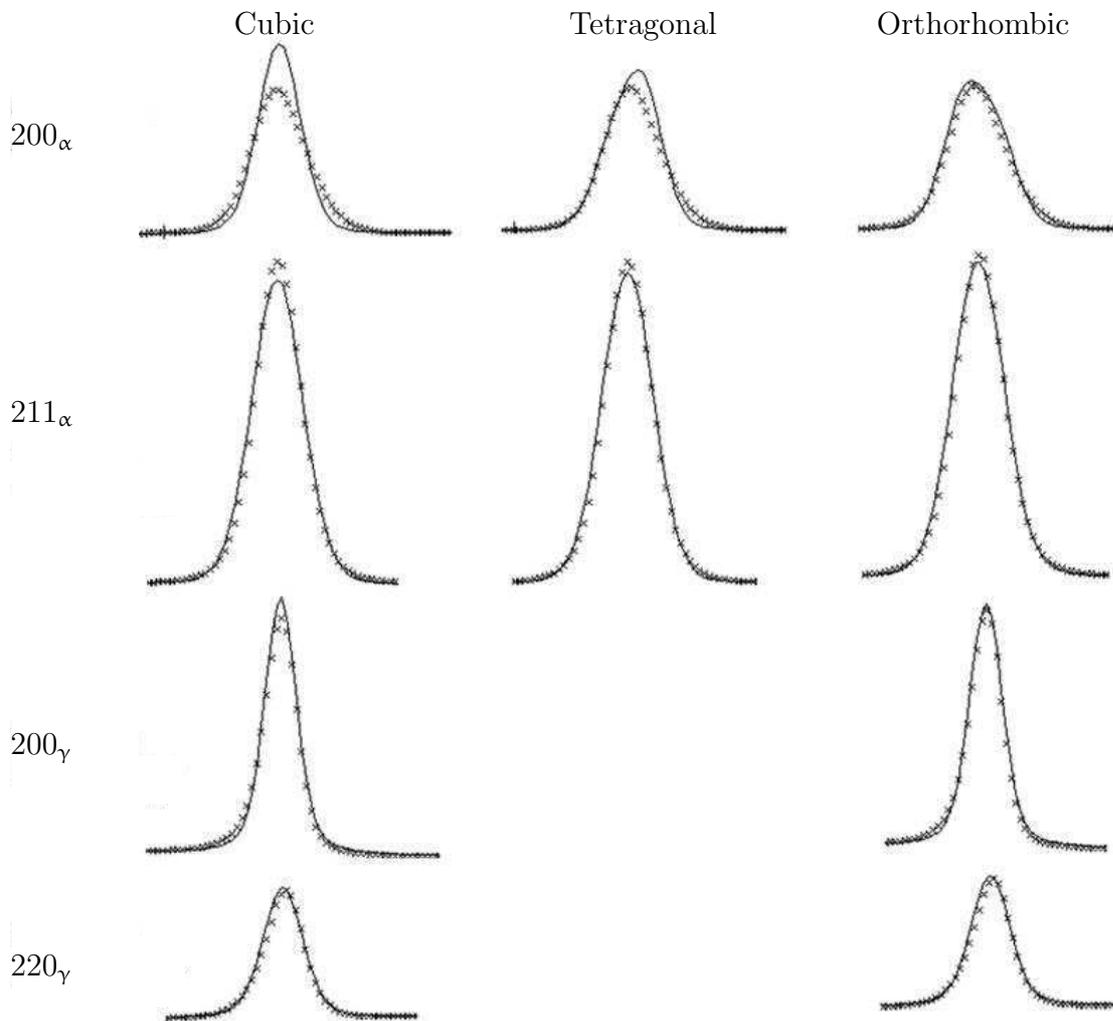
Figure 10.2: Peak profiles calculated in MAUD for the  $200_\alpha$  and  $211_\alpha$  peaks and austenite  $200_\gamma$  and  $220_\gamma$  peaks using cubic, tetragonal and orthorhombic space groups. Austenite is equally well-fitted by a face-centred cubic or a face-centred orthorhombic lattice. There is a significant improvement in the fit of ferrite from a body-centred cubic lattice to body-centred tetragonal. Reproduced with permission of Elsevier B. V.
