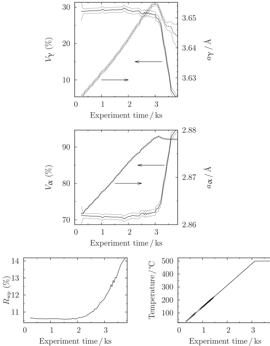
Figure 8.6: Rietveld refinement results for Alloy 8 transformed at 250°C and investigated using synchrotron XRD with *in-situ* heating. Grey lines represent  $\pm$  the standard error for each measurement.
