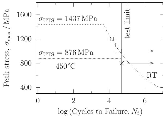
Figure 9.13: Fatigue test results for Alloy 9. Data are shown for tests performed at both ambient (+) and unit[450]°C (x). Tests marked with an arrow did not fail with in the 50,000 cycle limit. No S–N curve is shown for tests conducted at 450°C as no test resulted in a fatigue failure.
