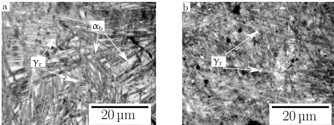
Figure 4.11: Alloy 1 tempered at 450°C for (a) 1 d and (b) 3 d. After 3 d there is a visible change in structure, presumably due to thermal decomposition.
