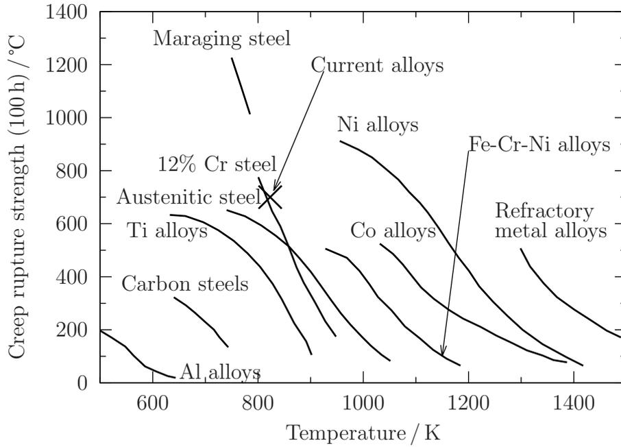
Figure 9.19: Comparison of typical creep performance of various steel grades and selected other materials [after 331] and comparison with the current alloys. Only maraging steels and nickel alloys outperform Alloy 8 and Alloy 9.
