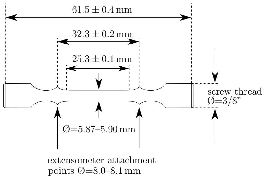
Figure 9.1: Sample geometry for tensile tests. All testpieces were machined from blanks after heat treatment to a maximum surface roughness of  $3 \text{ mm}$  in the gauge volume and  $5 \text{ }\mu\text{m}$  elsewhere.
